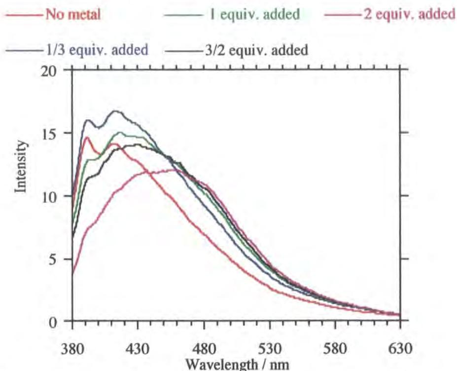
Figure 3.23 Fluorescence of ligand **166** on addition of potassium iodide (methanol, 298 K,  $\lambda_{em} = 350 \text{ nm}$ , ligand concentration =  $2.5 \times 10^{-5} \text{ mol dm}^{-3}$ )
