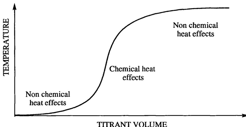
Figure 1.07 A typical thermogram
