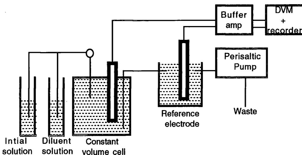
Figure 2.14 Apparatus used for ion selective electrode evaluation.
