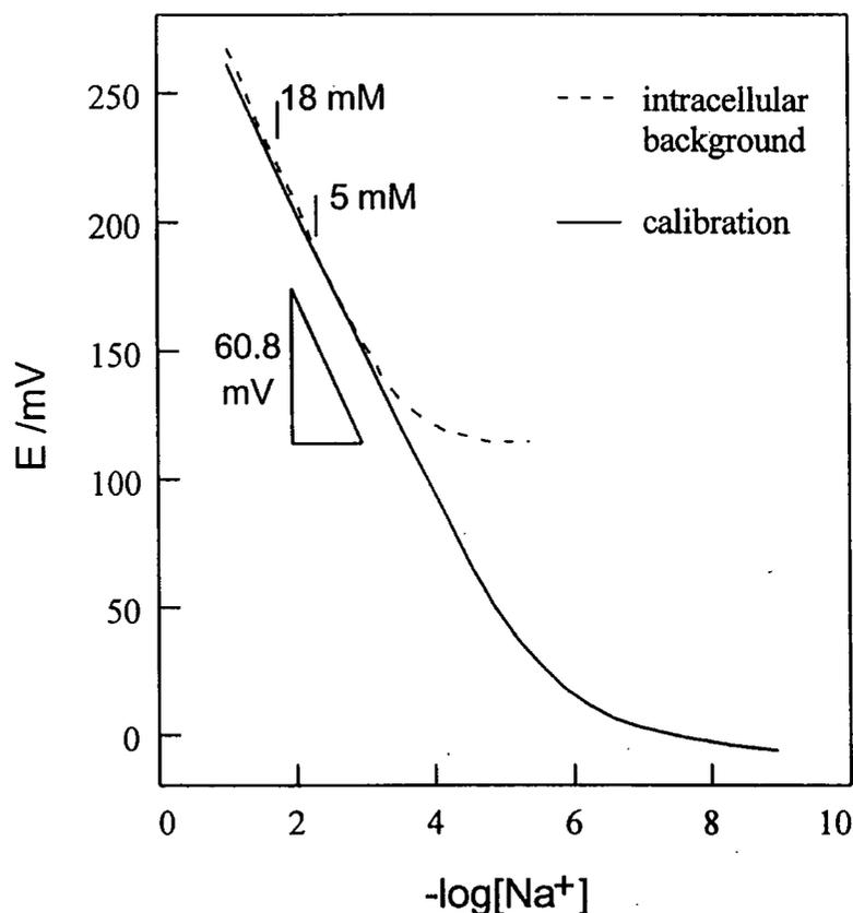
Figure 2.18 Response curve for  $\text{Na}^+$  obtained with the electrode based on 64 in the presence of interfering ions, of concentrations similar to those found in intracellular fluids (310K; 120 mM  $\text{K}^+$ , 3 mM  $\text{Mg}^{2+}$ , 0.4  $\mu\text{M}$   $\text{Ca}^{2+}$ ).
