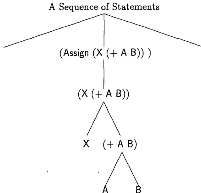
Figure 6.4: Diagrammatic Form of a WSL Syntax Tree
