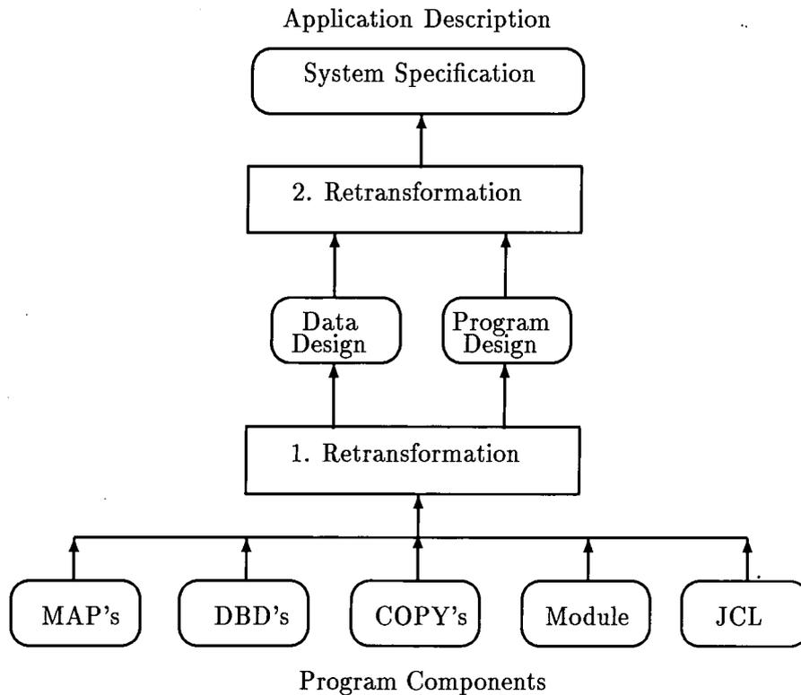
Figure 3.7: Inverse Transformation of Software from Code to Specification
