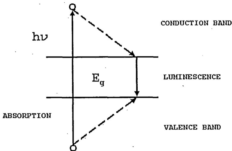
Figure 1.2: Schematic energy level diagram for a solid with bandgap energy  $E_g$  (Duley 1992).
