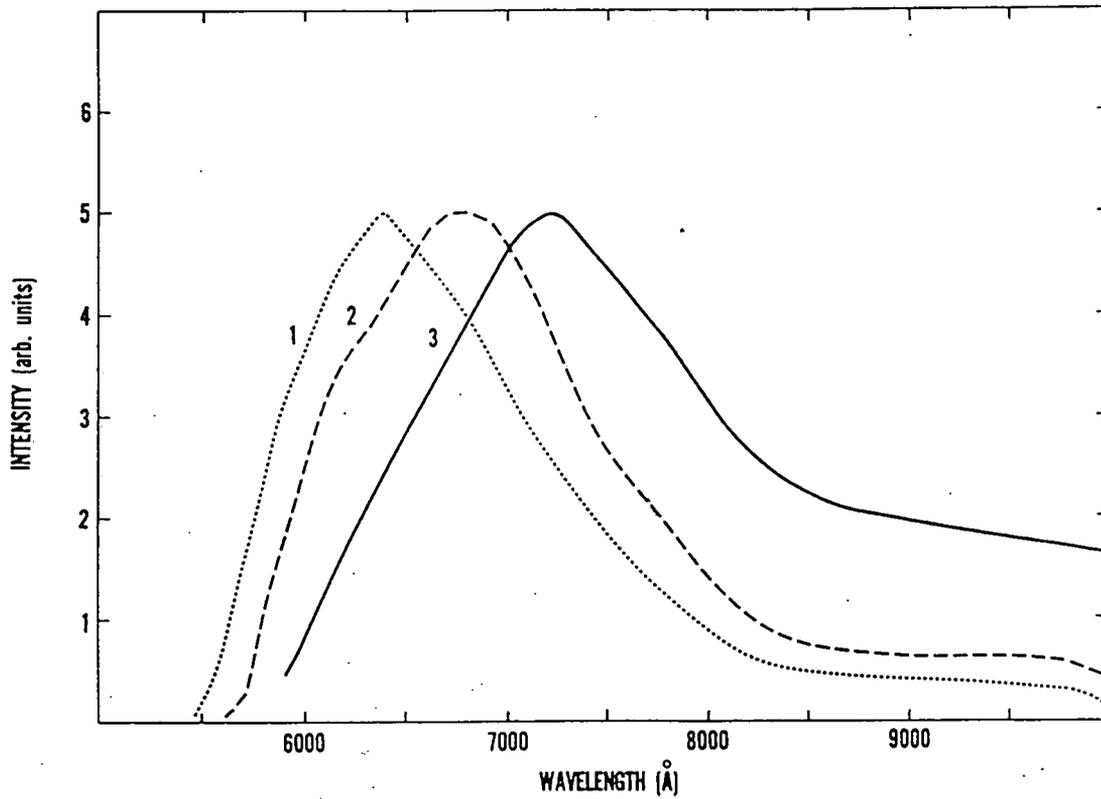
Figure 1.1: Reproduction by Witt and Schild (1988) of the photoluminescence spectra of laboratory HAC films observed after excitation with  $5145 \text{ \AA}$  radiation by Watanabe *et al.* (1982). Curves 1, 2, and 3 correspond to samples at increasing temperatures.
