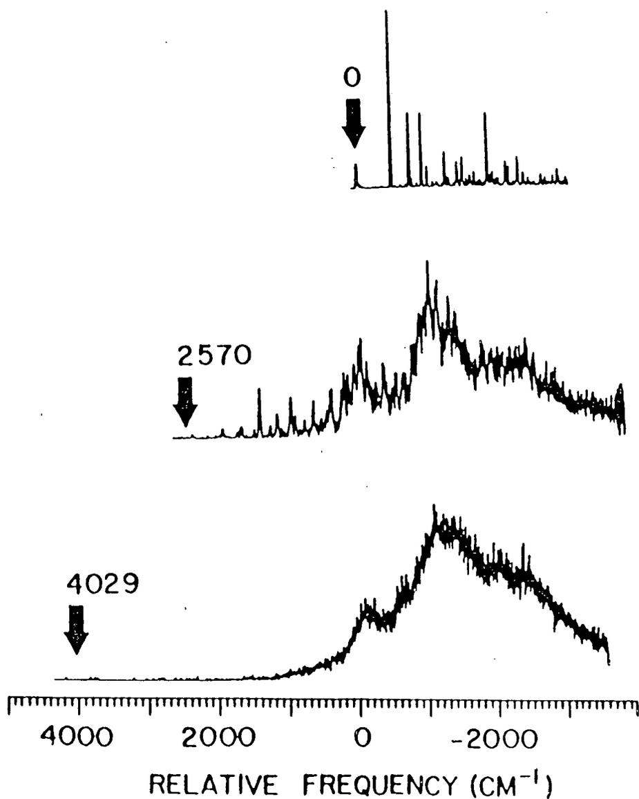
Figure 1.4: Fluorescence spectra of laboratory naphthalene (Beck *et al.* 1980; 1981). The number at the beginning of the spectra indicates the energy which is provided by a tunable laser in excess to the  $S_1 - S_0$  transition. The molecule is excited at progressively higher energies.
