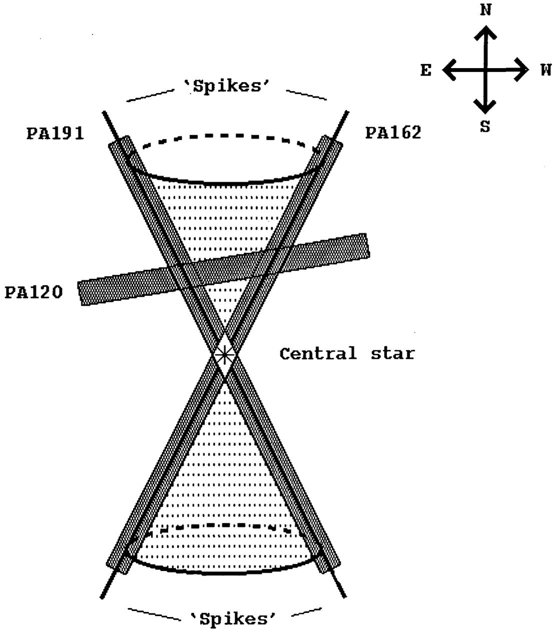
Figure 2.2: The three positions of the slit with respect to the Red Rectangle.
