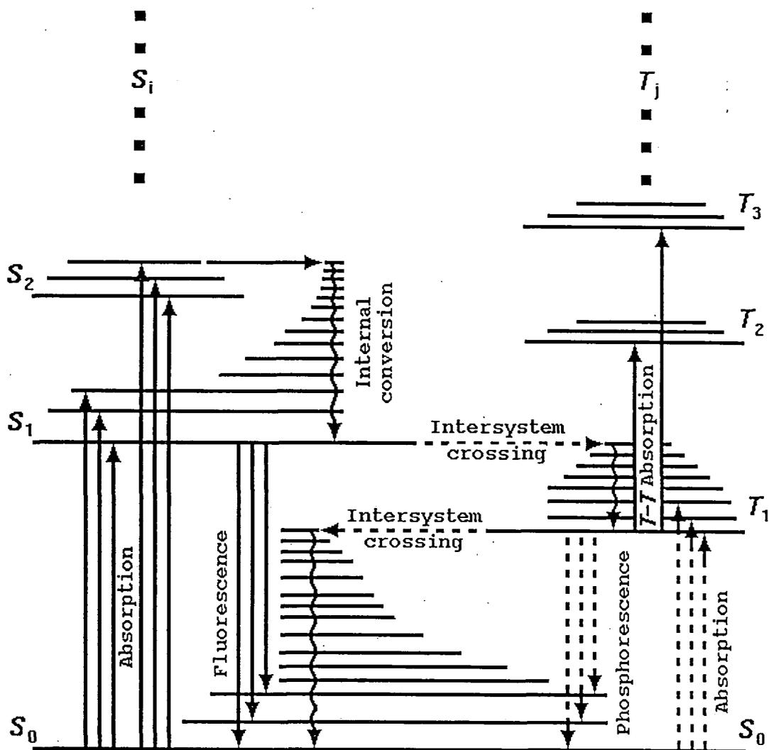
Figure 1.5: A schematic diagram of the lower energy levels of an organic molecule (d'Hendecourt *et al.* 1986).
