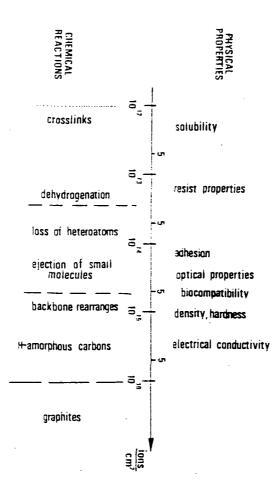
Figure 7: Qualitative trends of ion fluence vs. typical chemical reactions and related physical properties<sup>62</sup>.
