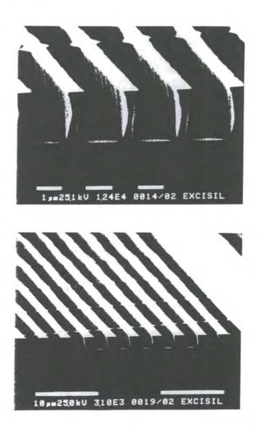
Figure 5: Self-developed submicrometer images produced in a thin film (0.2  $\mu$ m) of a polysilane (poly(p-tert-butylphenylmethylsilane) by irradiation at 248 nm. Images transferred by oxygen reactive ion etching<sup>50</sup>.
