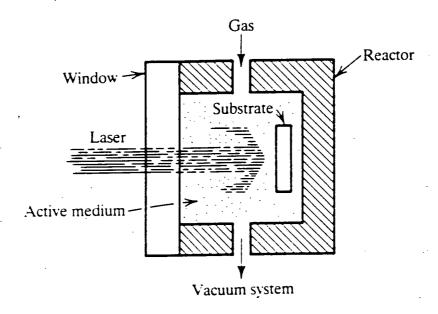
Figure 4: Schematic of Photo-CVD reactor<sup>7</sup>.
