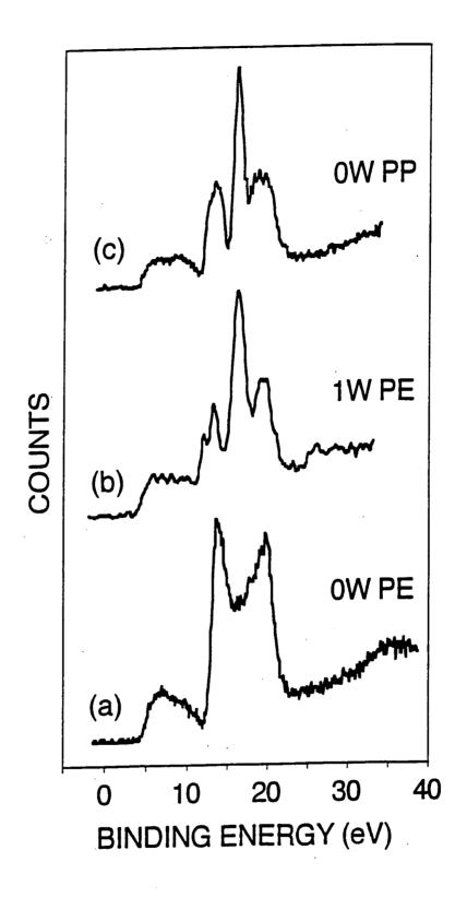
Figure 1: XPS valence band spectra of: (a) clean polyethylene; (b) 1W plasma oxidized/aged polyethylene (10<sup>5</sup> min); and (c) clean polypropylene. (The surface normal was tilted 30° away from the axis of the spectrometer).
