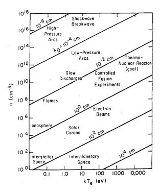
Figure 8: Typical plasmas characterised by their electron energy and density<sup>79</sup>.
