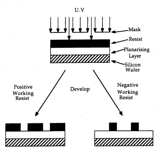
Diagram 1: Schematic of positive and negative working resists.
