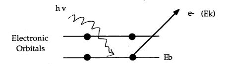
Scheme 1: Ejection of a photoelectron<sup>7</sup>.
