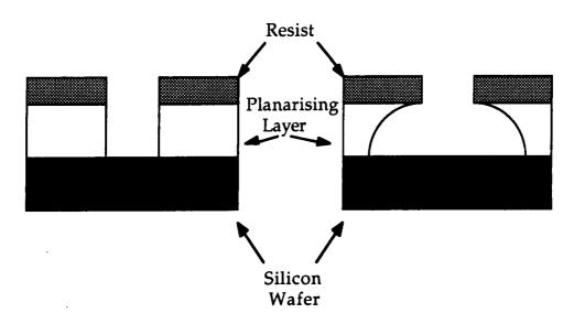
Diagram 1: Anisotropic (left) and isotropic (right) etching.
