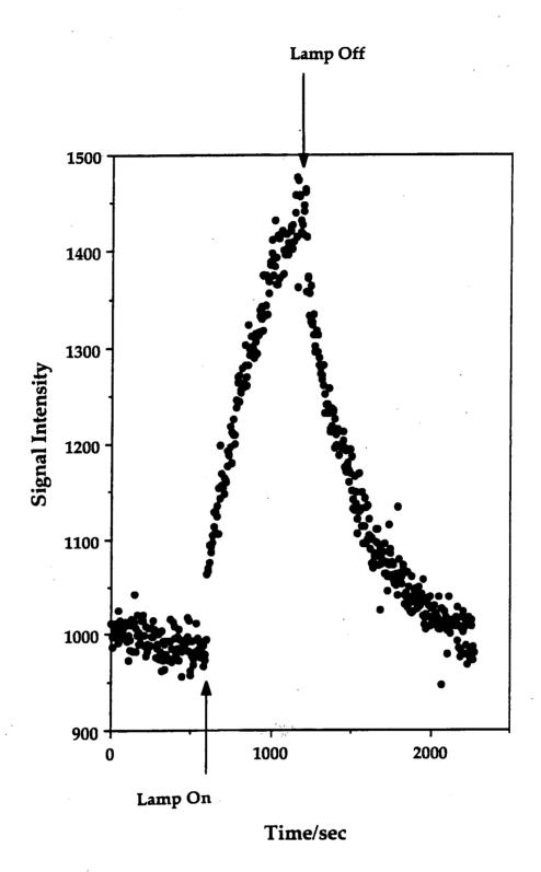
Figure 2: Mass 2 intensity profiles (before, during, and after UV irradiation) for photo-oxidation.
