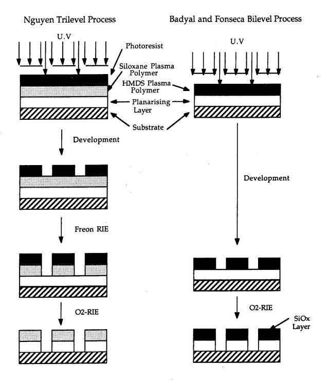
Diagram 6: Trilevel vs Bilevel schemes in wafer fabrication.
