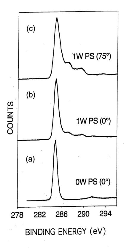
Figure 2: C(1s) region of (a) clean polystyrene; (b) 1W plasma oxidized/aged polystyrene (10<sup>5</sup> min, the surface normal was aligned with the axis of the spectrometer); and (c) 1W plasma oxidized polystyrene/aged (10<sup>5</sup> min, the surface normal was tilted 75° away from the axis of the spectrometer).
