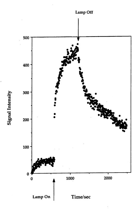
Figure 13: Mass 105 intensity profile (before, during, and after UV irradiation) for photolysis.
