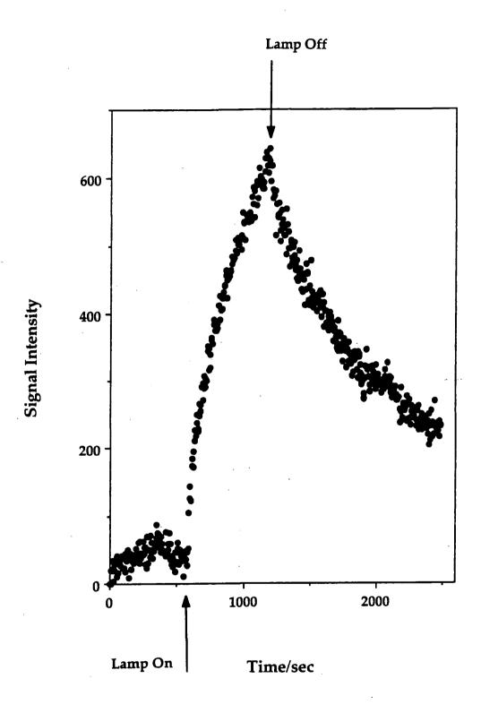
Figure 9: Mass 91 intensity profile (before, during, and after UV irradiation) for photloysis.
