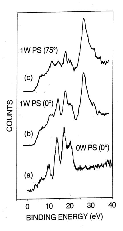
Figure 3: XPS valence band spectra of: (a) clean polystyrene; (b) 1W plasma oxidized/aged polystyrene (10<sup>5</sup> min, the surface normal was aligned with the axis of the spectrometer); and (c) 1W plasma oxidized/aged polystyrene (10<sup>5</sup> min, the surface normal was tilted 75° away from the axis of the spectrometer).
