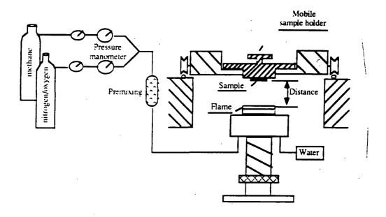
Figure 2: Equipment used in flame treatment of polymer surfaces<sup>4</sup>.
