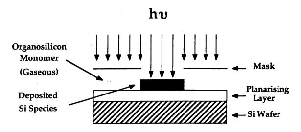
Diagram 7: Proposed scheme for direct deposition of silicon-containing species upon a planarising layer.
