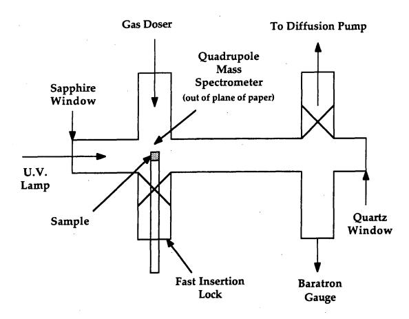
Figure 1: Schematic of ultra high vacuum chamber used.
