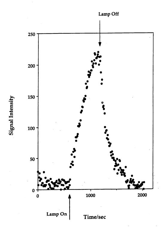
Figure 5: Mass 41 intensity profile for pure PVC (before, during, and after UV irradiation).
