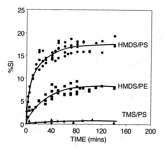
Figure 4: Irradiation induced uptake of silicon for: (a) hexamethyldisilane / polystyrene; (b) hexamethyldisilane / polyethylene; and tetramethylsilane / polystyrene. (N.B. %C + %Si + %O = 100%, as determined by XPS)
