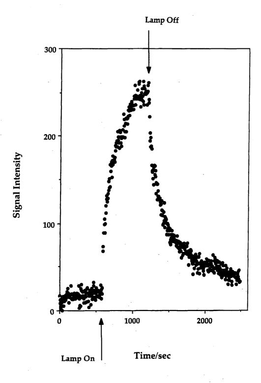
Figure 12: Mass 104 intensity profile (before, during, and after UV irradiation) for photolysis.
