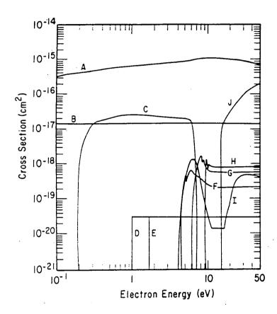
Diagram 4: Elastic and inelastic collision cross-sections for electrons in oxygen; (A) elastic scattering; (B) rotational excitation; (C) vibrational excitation; (D) excitation to the  $^1\Delta_g$  state; (E) excitation of the  $^1\Sigma_u^+$  state; (F) excitation of the  $^3\Sigma_u^+$  state; (G) excitation of the  $^3\Sigma_u^-$  state; (H) excitation of higher electronic states; (I) dissociative attachment; (J) ionisation<sup>22</sup>.
