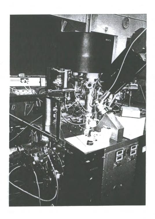
Plate 1: Kratos ES300 surface analysis instrument.
