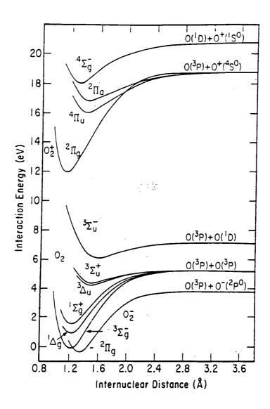
Diagram 1: Potential energy curves for some states of O<sub>2</sub>-, O<sub>2</sub>, and O<sub>2</sub>+.9
