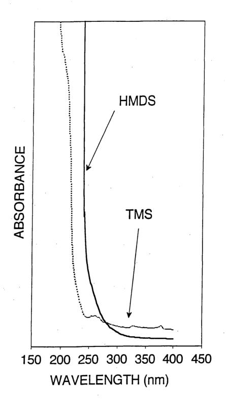
Figure 3: UV absorption spectra of hexamethlydisilane and tetramethlysilane.
