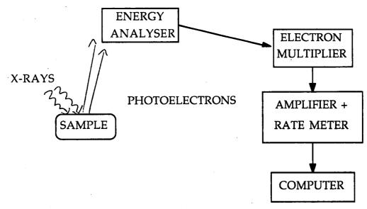
Scheme 3 : XPS experiment schematic.
