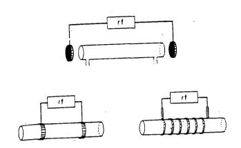
Figure 12: Typical arrangements for r.f. discharges<sup>81</sup>.
