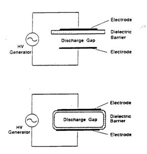
Figure 11: Silent discharge configurations with one (top) or two (bottom) dielectric barriers<sup>96</sup>.
