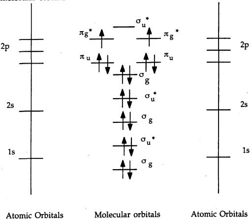
Diagram 1: Occupied molecular orbitals of molecular oxygen<sup>21</sup>.
