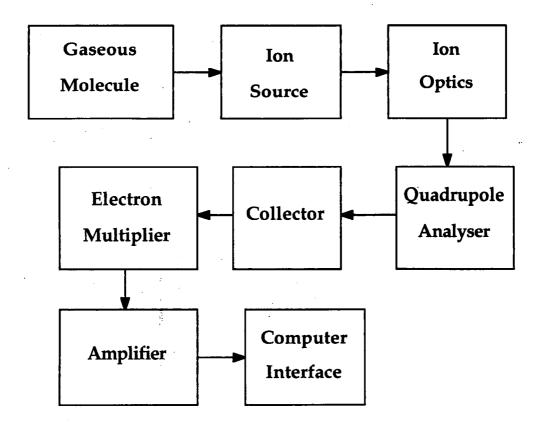
Scheme 9: Schematic of a Quadrupole Mass Spectrometer.
