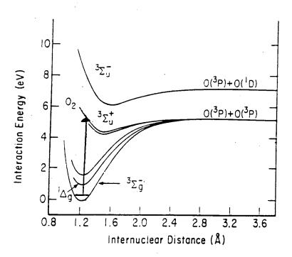
Diagram 3: Potential energy curves showing the formation and subsequent dissociation of  ${}^3\Sigma_u{}^+$ , resulting in production of O ( ${}^3P$ ). (Modified from Reference 22)
