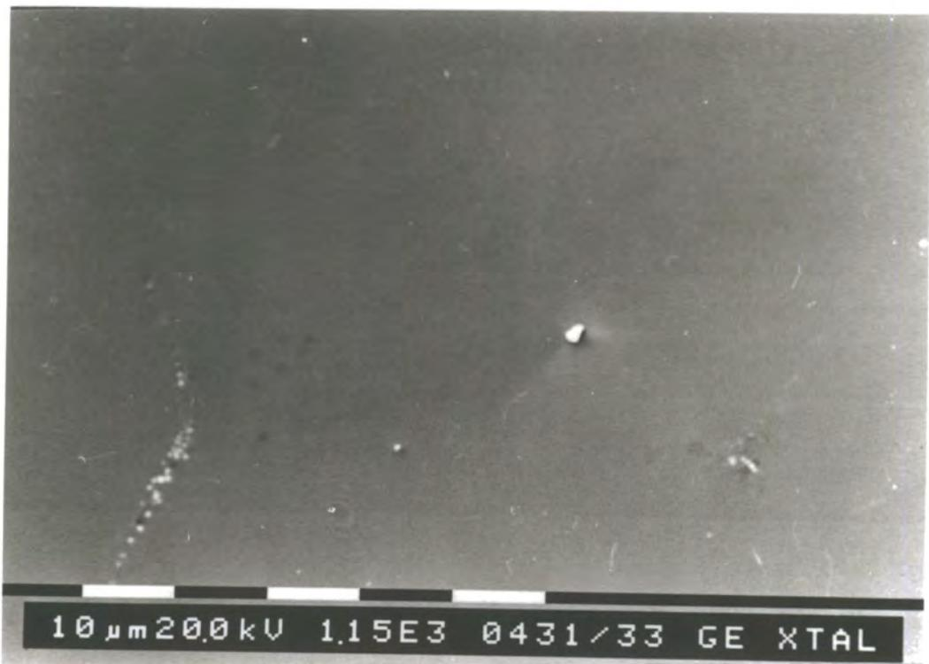
Figure 4.11 - An SEM Micrograph of a Good Quality Film
