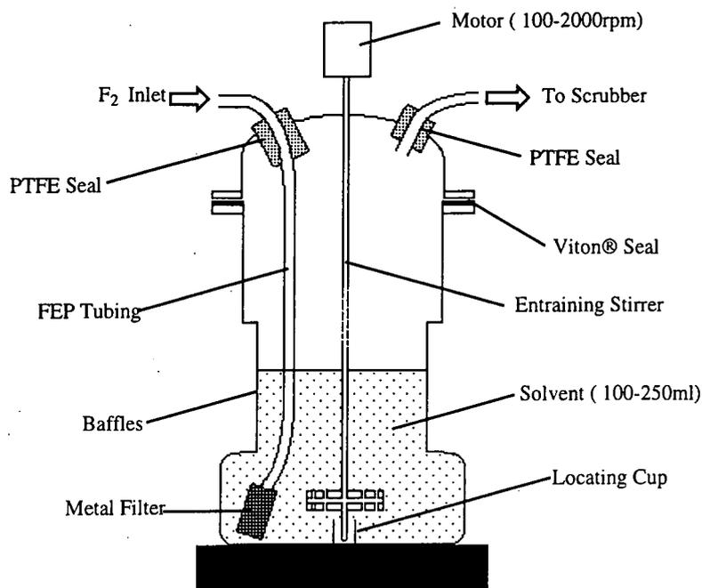
Figure 5: Fluorination Reactor(III).
