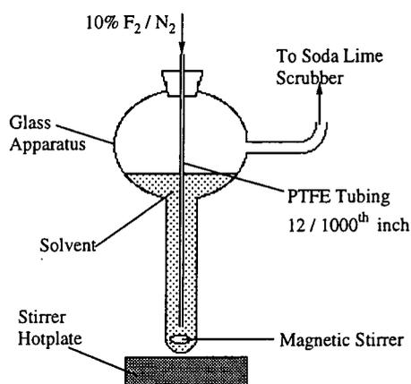
Figure 3: Fluorination Reactor(I).
