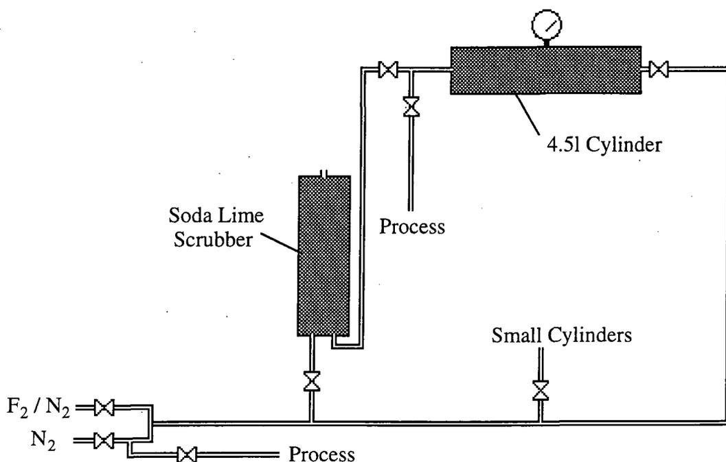
***N.B. Fluorination Reactions Must Never Be Run Directly From The Large 50% Fluorine / Nitrogen Cylinder***
