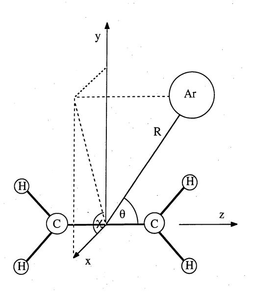
Fig. 1.i Co-ordinate System for Argon-Ethene.
