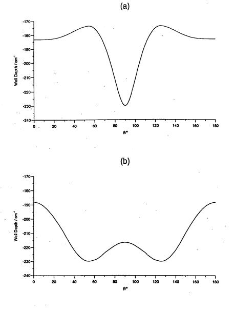
Fig. 6.iii Well depth as a function of angle. (a) Function of  $\theta$  where R and  $\chi$  have been varied to find the deepest point in the well at each angle. (b) Function of  $\chi$  at  $\theta = 90^{\circ}$  where R only has been varied.
