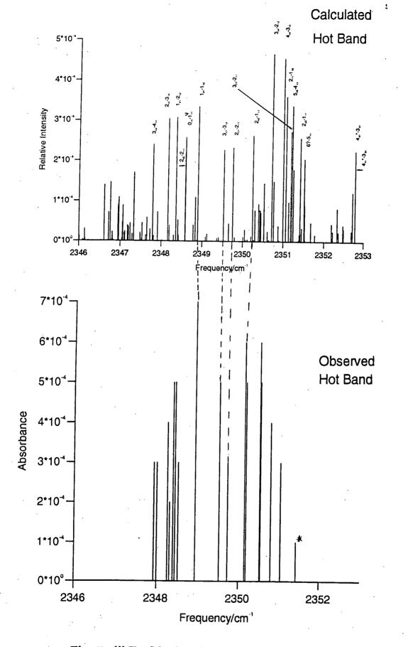
Fig. 5.viii He–CO<sub>2</sub> Calculated and observed hot band transitions in the region of all the observed hot band lines. Dotted lines indicate (very) tentative assignment.
