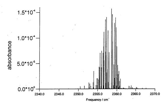
Fig. 5.ix He-CO<sub>2</sub> Calculated Combination Band Transitions.
