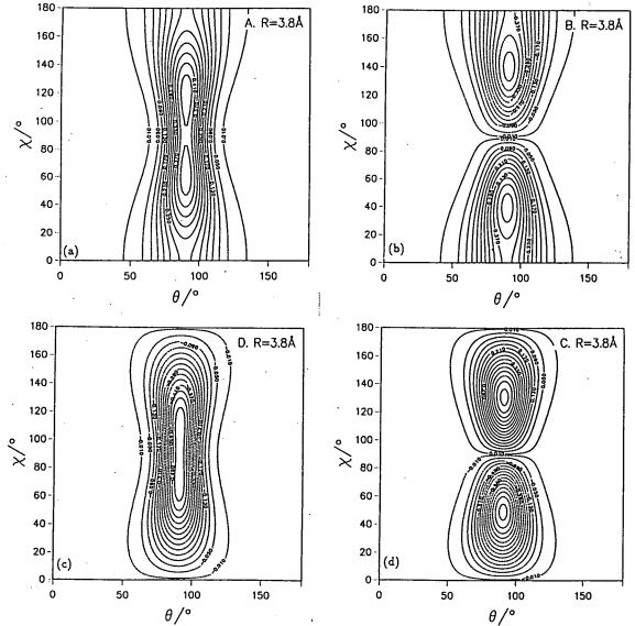
Fig. 6.v Lowest Energy Level of  $Ar-C_2H_4$  in each Symmetry Category as a Function of  $\theta$  and  $\chi$ . (a) Ground State (Symmetry A), (b) Symmetry B<sub>2</sub>, (c)Symmetry B<sub>1</sub>, (d)Symmetry B<sub>3</sub>.
