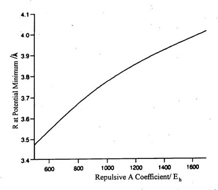
Fig. 2.11 Variation of Intermolecular Separation at the potential minimum  $R_m$  with Carbon Repulsive Coefficient.
