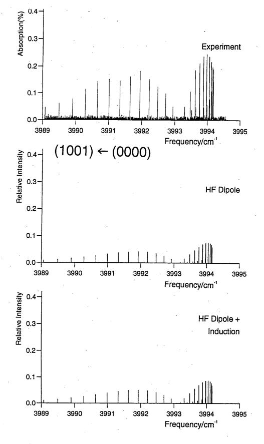
Fig. 4.vi Comparison of experimental and calculated spectra for the 1001  $\leftarrow$  0000 band of Ar-HF. The calculated intensities are scaled (with a single overall scaling factor for all bands) to reproduce the experimental peak intensity for the 1000  $\leftarrow$  0000 band.
