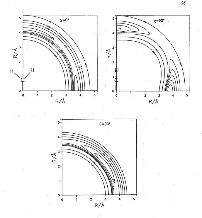
Fig. 6.ii Plots of the Peet Potential. (a) In the molecule plane. (b) Perpendicular to the molecule plane along molecule axis. (c) Perpendicular to molecule plane and molecule axis.
