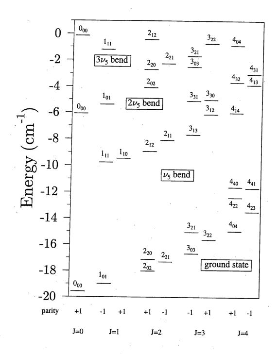
Fig. 5.iii Asymmetric Top Energy Levels for He-CO<sub>2</sub> in the CO<sub>2</sub> Ground Vibrational State from Close Coupling Calculations on the Modified Beneventi potential.
