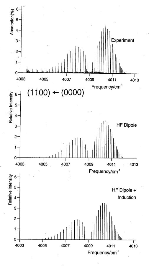
Fig. 4.iv Comparison of experimental and calculated spectra for the 1100  $\leftarrow$  0000 band of Ar-HF. The calculated intensities are scaled (with a single overall scaling factor for all bands) to reproduce the experimental peak intensity for the 1000  $\leftarrow$  0000 band.
