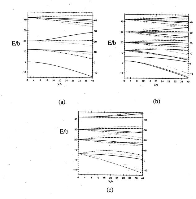
Fig. 3.v Correlation diagrams for energy levels of atom-tetrahedral molecule complexes, as a function of increasing  $V_3$  anisotropy. (a) A states; (b) F states; (c) E states. Only levels with  $K \leq 2$  are shown. Solid lines are K = 0 states; dashed lines are K = 1 states; dotted lines are K = 2 states.
