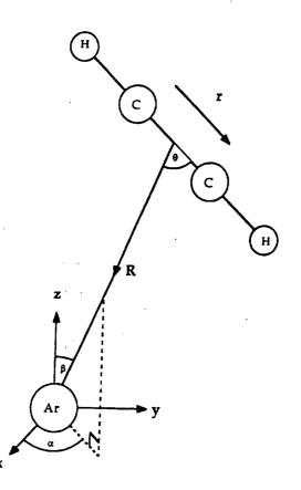
Fig. 2.i Coordinate System for Argon-Acetylene.
