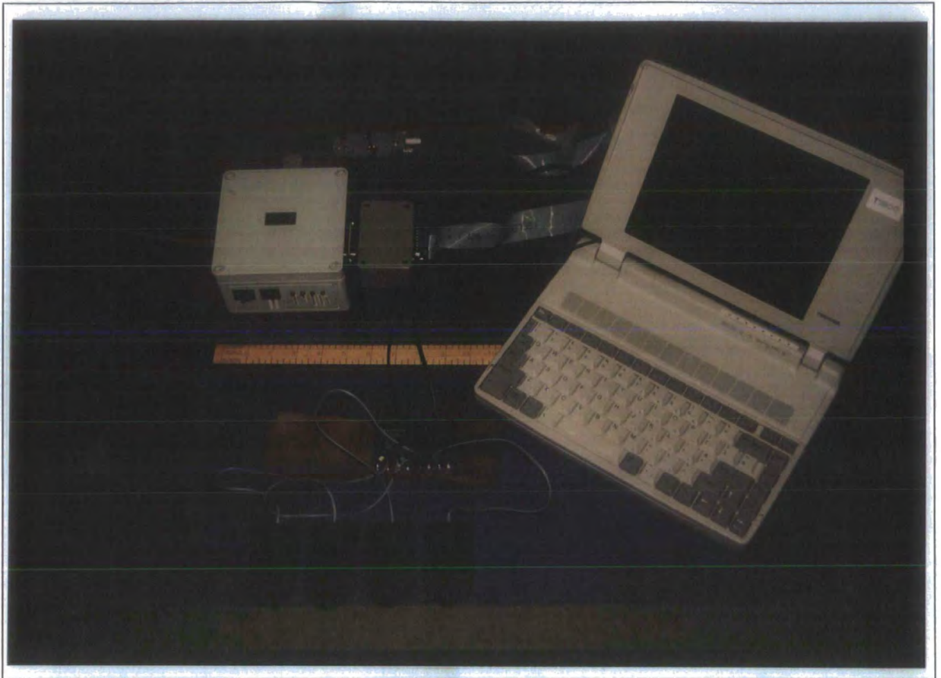
Figure 2.6 - A photograph of the whole monitoring system, with the ambulatory monitor connected to the PC.
