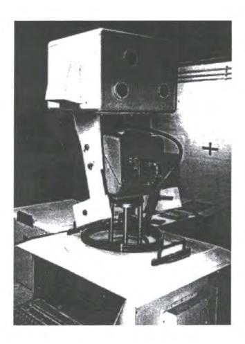
Figure 3.1 An upgraded radiometer unit, showing instrument box, pan-and-tilt head and computer box
