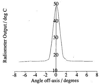
Fig 3.4a Azimuth Angle Point-Spread Function for KT19 Radiometer
