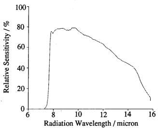
Figure 3.2a Spectral Sensitivity of KT17 Radiometer
