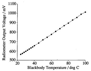
Fig. 3.5. Calibration Curve for Low Temperature Range KT19
