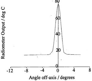
Fig 3.4b Zenith Angle Point-Spread Function for KT19 Radiometer
