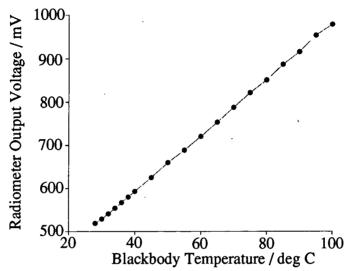
Fig 3.6. Calibration Curve for Standard KT19 Thermometer
