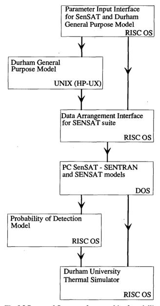
Fig. 6.8. Proposed Structure for a combined modelling and display software suite
