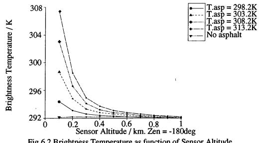
Fig. 6.2 Brightness Temperature as function of Sensor Altitude for asphalt targets of different temperatures.
