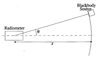
Fig. 3.3 Experimental set-up for determination of sensor field-of-view
