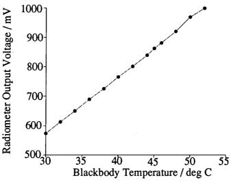
Fig. 3.9. Calibration Curve for CE825
