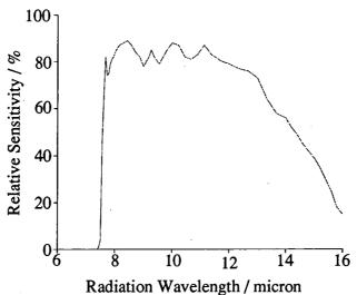
Figure 3.2b Spectral Sensitivity of KT19 Radiometer
