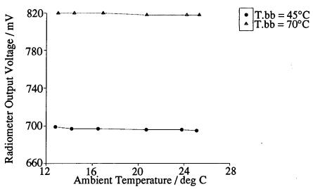
Fig. 3.7. Dependence of Output Voltage on Ambient Temperature for low temp KT19
