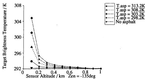
Fig. 6.3 Brightness Temperature as function of Sensor Altitude for asphalt targets of different temperatures
