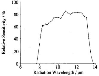
Fig.6.1. Spectral Sensitivity of Bendix Scanner
