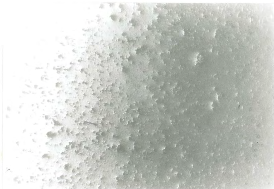
Figure 2.7 A 10% polyaniline solution left for 24 hours, centrifuged then spun.
