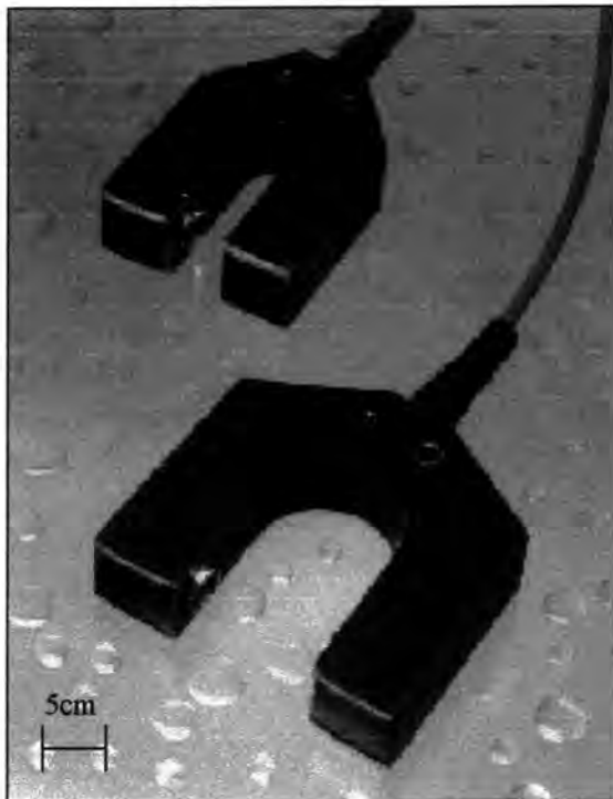
Figure 4.1. Two models from Partech's range of IR sensors. Note the different gap sizes, giving each sensor a different range and accuracy.
