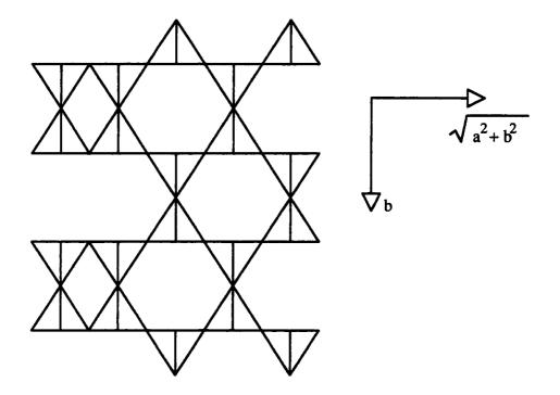
Figure 3.16 The hypothetical structure of Brandt and co-workers for kenyaite.9,10
