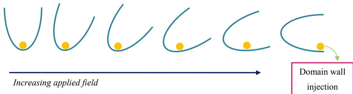
Figure 7:9. Schematic of domain wall injection, in which the domain wall is illustrated as a quasi-particle pinned in a potential well. A domain wall pinned at the junction between the nucleation pad and a wide nanowire can be compared to that of a wall in a shallow potential well, as shown in (a). A wall pinned at the junction between the nucleation pad and a narrow wire is like a particle pinned in deep potential well as shown in (b).
