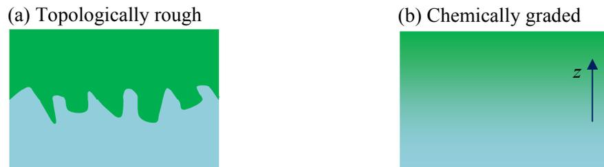
Figure 4:8. Examples of the type of transition that can exist at an interface between two materials (a) topologically rough and (b) chemically graded interface.
