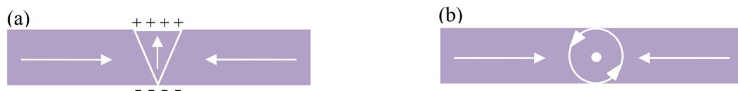
Figure 7:13. Schematic illustration to show how the magnetostatic energy associated with (a) the transverse wall structure and (b) the vortex wall structure.
