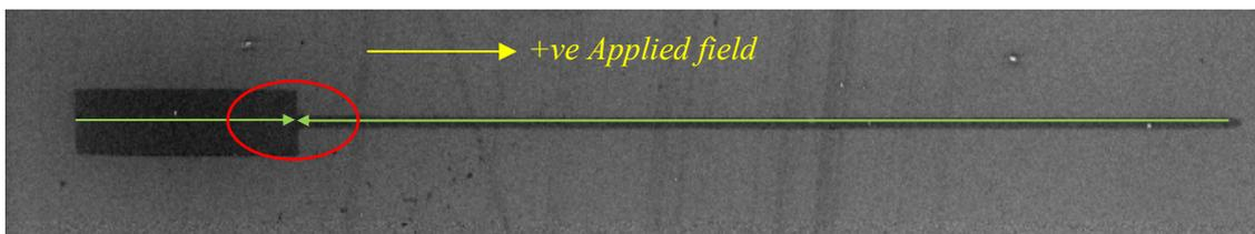
Figure 7:6. Schematic to show location of the laser spot used to measure domain wall injection from the nucleation pad to the nanowire. The arrows indicate the formation of a head-to-head domain wall that is pinned at the pad-wire interface.
