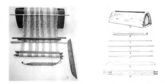
Fig.19: A set of Taiyal loom (from National Museum of History,1997:50). A. Main beam. B. Shed stick. C.E.F. Laze rods. D. Heald rod. G. Sword. H. Breast beam. (sketch drawing from Chen,1988[1968]:102)
