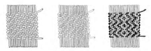
Fig.22: a. A balanced twill weave (2:2) that intersects over and under two threads at a time. b. A 3:1 twill weave. c. A diamond twill (adapted from Fraser-Lu,1988:57).
