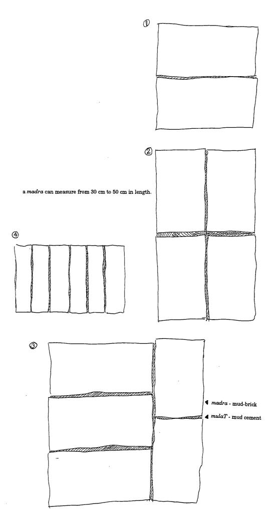
Fig. 6. Methods of laying madar.
