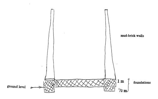
Fig. 5. Sketch of house walls and foundations showing the sloped outer walls and the straight inner walls.
