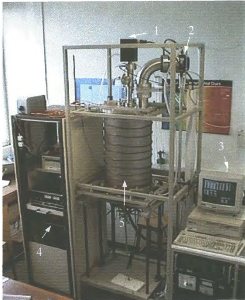
Figure 2. Photograph of the Durham growth system. Arrow numbers: 1) mass spectrometer, 2) turbomolecular pump, 3) PC control, 4) measuring and diagnostic instruments and 5) vacuum jacket.
