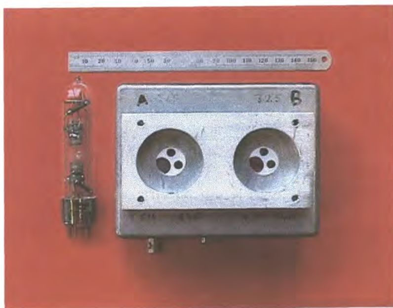
Figure 8. HC Lamp and detection system for in situ monitoring of cadmium and tellurium vapour pressures in the CdTe Durham vapour growth apparatus.
