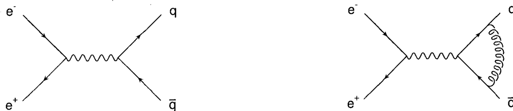
Figure 2.2: The lowest order (left) and next-to-leading order (right) Feynman diagrams for the production of 2 partons in e^+e^- annihilation. The momenta of the particles are incoming and outgoing for initial and final state particles respectively, whilst the arrows on the electron and quark lines represent the direction of fermion flow.
