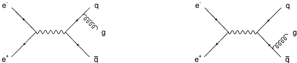
Figure 2.3: The two lowest order Feynman diagrams for three parton production, e^+e^- \rightarrow q\bar{q}g . The gluon simply couples to the quark-antiquark line either side of the photon.
