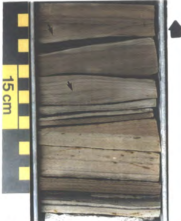
Fig. 2.4 Slabbed core sample from well C1-49 showing parallel lamination in the lower part overlain by hummocky cross-stratification, emphasised by very thin mm thick carbonaceous drapes. Arrows show curvature of lamination within the hummocky cross-stratification.
