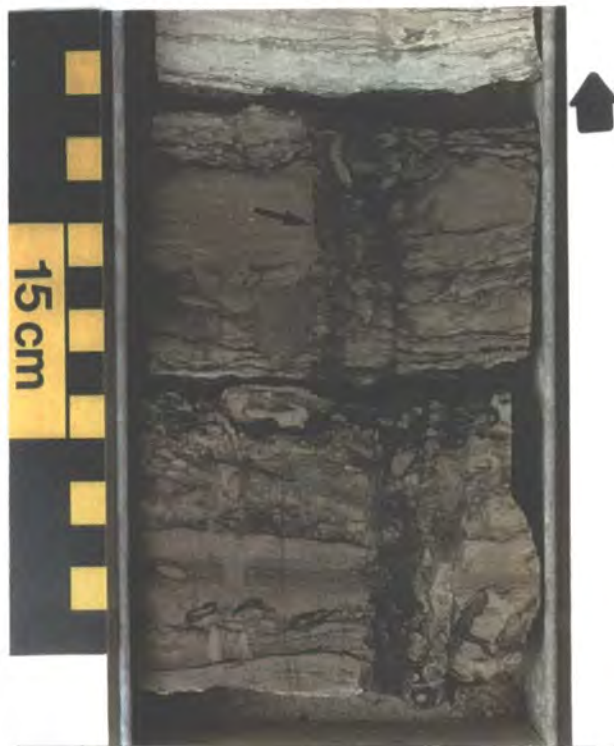
Fig. 2.7 Slabbed core sample from well C1-49 showing bioturbated sandstone and shale, with vertical and horizontal burrows. Note in-fill of large burrow (arrow) and obliteration of sedimentary structures by burrows, except for some remnant streaky wavy lamination.
