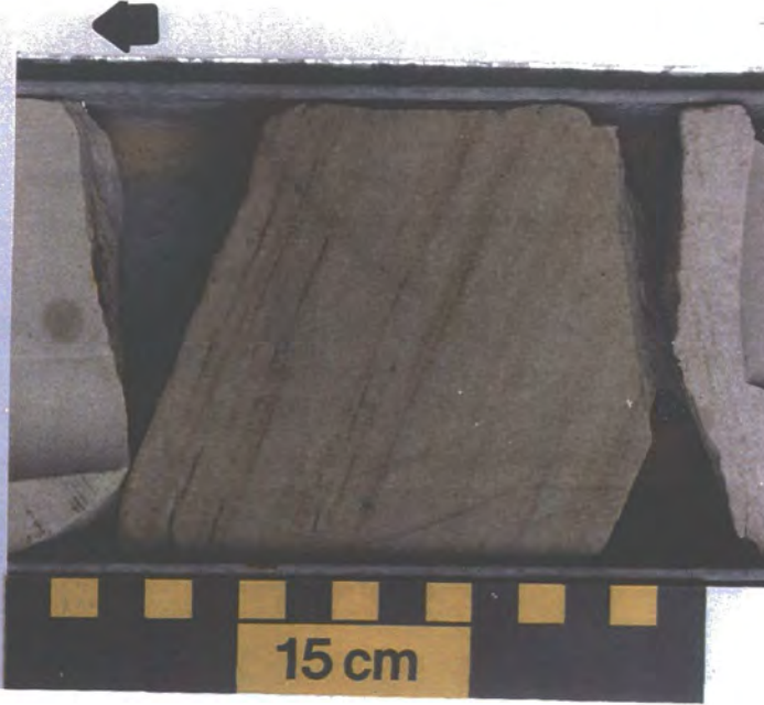
Fig. 2.22 Slabbed core sample from lower Tahara sandstone, well C1-49, showing planar cross-bedded sandstone.
