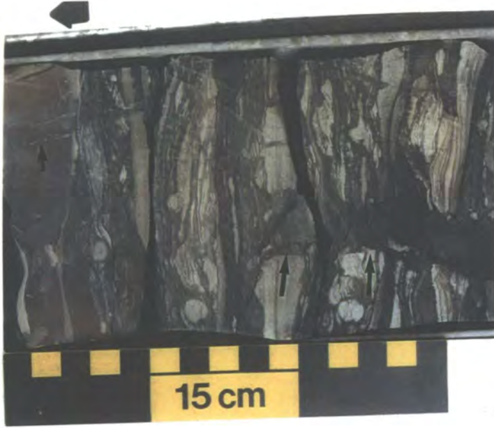
Fig. 2.10 Slabbbed core sample from heterolithic type 1 facies, well C1-49, showing bioturbated mudstone, silty shale and sandstone. Note vertical burrows (arrow) and dispersed horizontal burrows. At the top is an ironstone bed with sharp contact, containing streaky sandstone laminae and closely spaced desiccation cracks (filled with calcite, small arrow).
