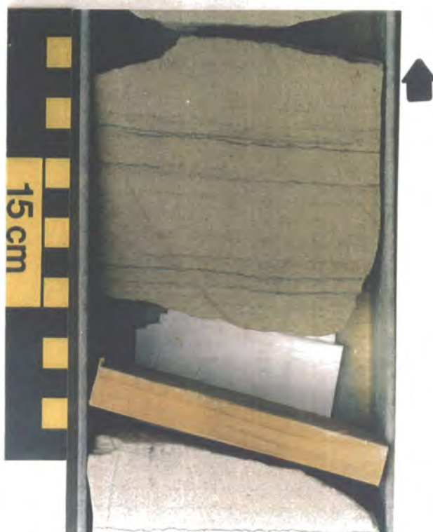
Fig. 2.23 Slabbed core sample from lower Tahara sandstone, well C1-49, showing the horizontally laminated sandstone enhanced by very thin carbonaceous laminae.
