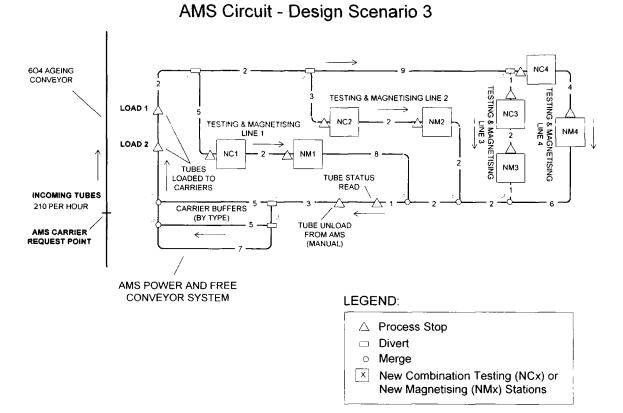
Figure A15. Schematic of Design Scenario 3 for AMS Circuit Layout.
