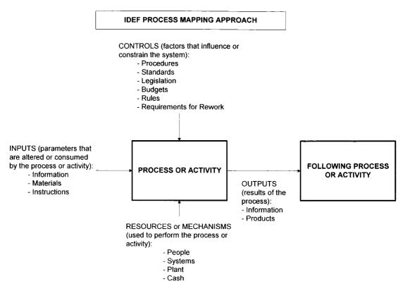
Figure 1. IDEF Process Mapping Methodology
