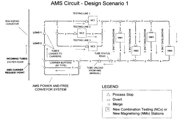
Figure A13. Schematic of Design Scenario 1 for AMS Circuit Layout.
