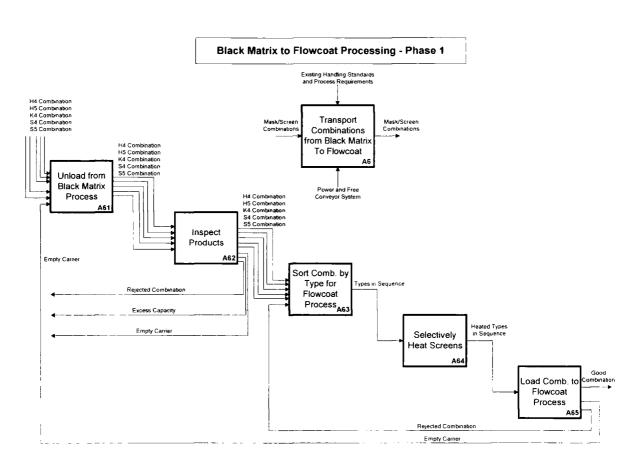
Figure 31. Process Map for Product Handling from Black Matrix to Flowcoat.
