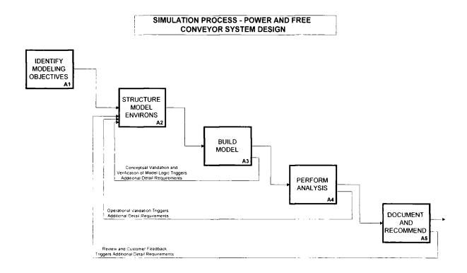
Figure 30. Simulation Methodology for Automated Systems.
