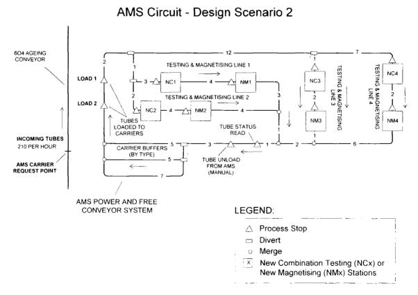
Figure A14. Schematic of Design Scenario 2 for AMS Circuit Layout.
