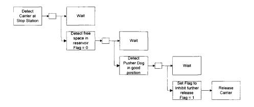
Figure 34. Detailed Process Map for Carrier Presence Control.
