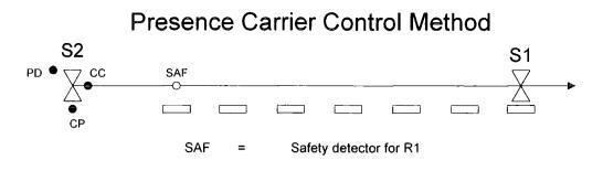
Figure 17. Reservoir Utilising Presence Carrier Control.
