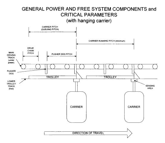
Figure 10. General Power and Free System Configuration.
