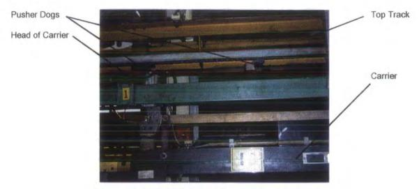
Figure A8. AMS Circuit Handling System Stop Station.
