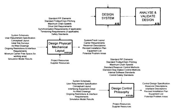
Figure 9. The Process of Designing the System.
