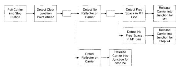
Figure 43. Example Structured Flow Diagrams for the AMS Handling System.
