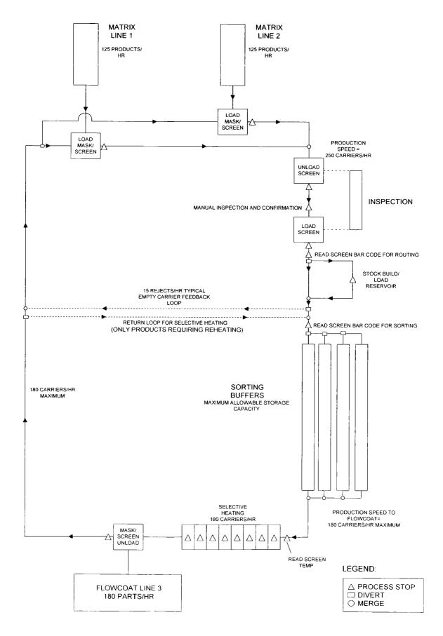
Figure 32. Schematic for the 215 System.
