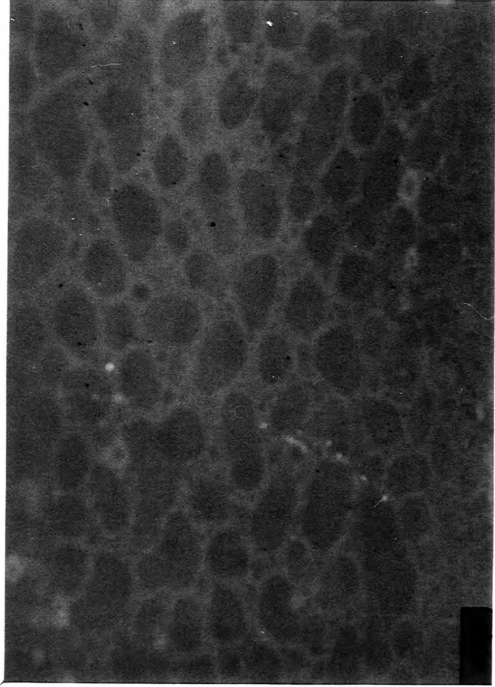
Figure 5.20 Scanning electron microscope (SEM) photograph of a thin SRO film of 0.5 min deposition time and \gamma = 0.22 at 650 °C.
