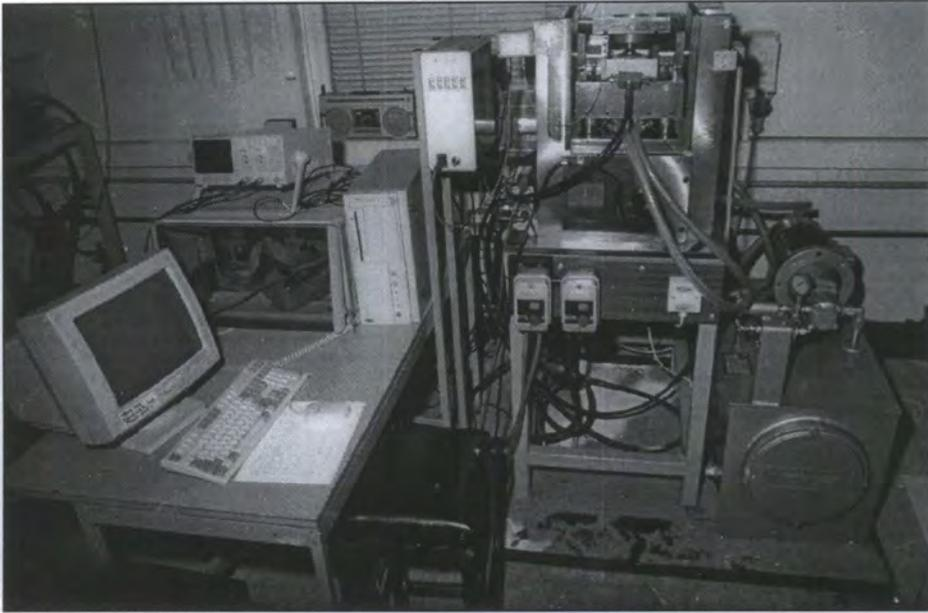
**Figure 3.1** Hip function friction simulator
