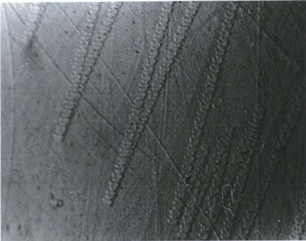
**Figure 9.17** A microscope photograph of tears on the surface of a C3 cup
