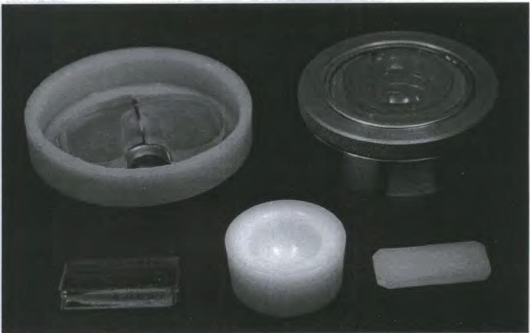
**Figure 4.1** Examples of polyurethane and UHMWPE components
