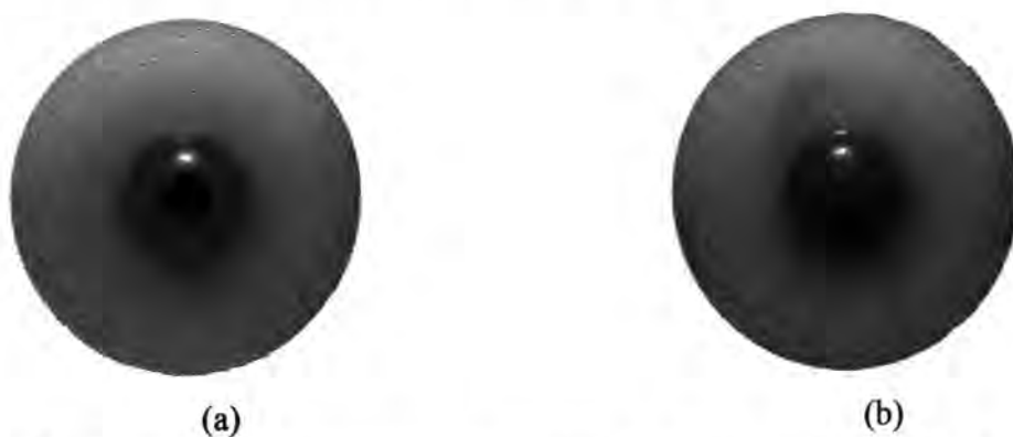
Figure 5.5 The effect of silver chloride precipitation on the inner surface of electrode membrane (a) standard inner fill solution and (b) silver chloride precipitate
