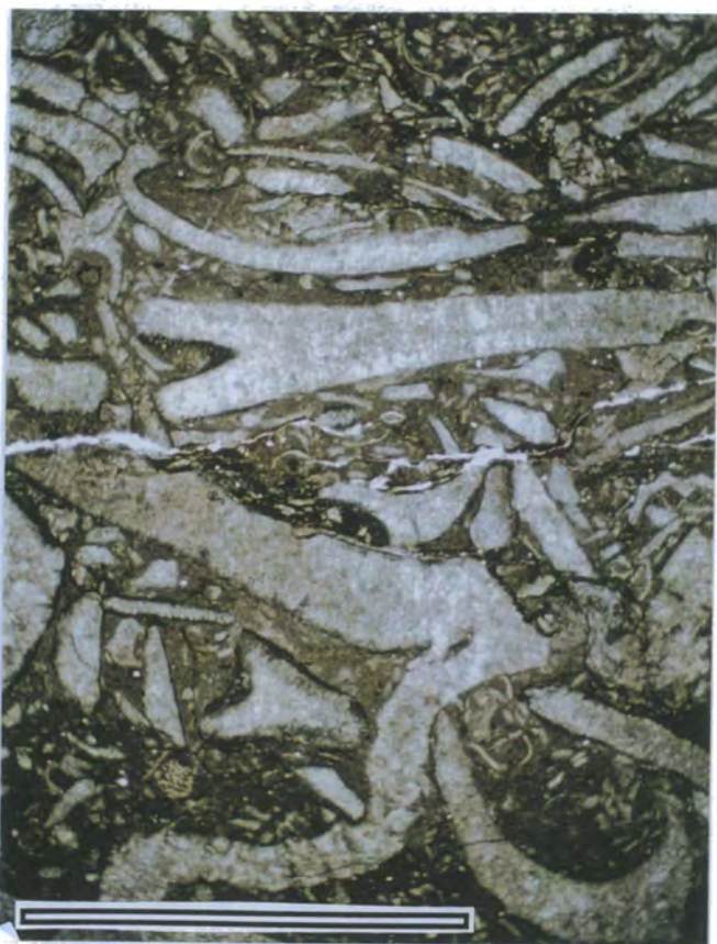
Plate 15 Microfacies S5. Bioclastic packstone, dominated by bivalves. Scale bar = 5mm. Sample number KL2, Keldenich quarry, Germany.
