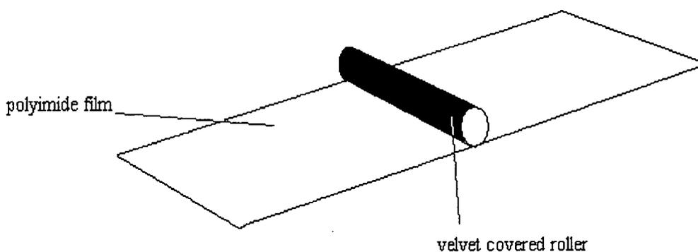
Various parameters can be altered to change the alignment such as the type of rubbing cloth used, rotation speed of the roller, speed that the polymer film passes under the roller and pile depth of the cloth.
