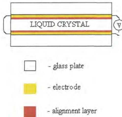
The glass plates are usually coated with a layer of transparent conducting material, for example, indium tin oxide. To create patterns in the cell the indium tin oxide coating can be etched so only part of the liquid crystal is 'switched' when an electrical field is applied. One of the plates is often coated with a reflective layer, e.g. vapour-deposited aluminium, to reflect incident light through the liquid crystal and back out of the cell.
