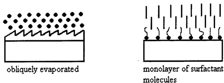
Another alignment technique shown schematically in Figure 1.9 is to use monolayer Langmuir coatings applied from aqueous solution to a surface. A glass slide is passed through an aqueous solution of surfactant (e.g. hexadecyltrimethylammonium bromide) and emerges coated in a monolayer of the surfactant. How the nematic liquid crystal is aligned depends on the concentration of the surfactant and the rate at which the glass plate is drawn through the solution.
