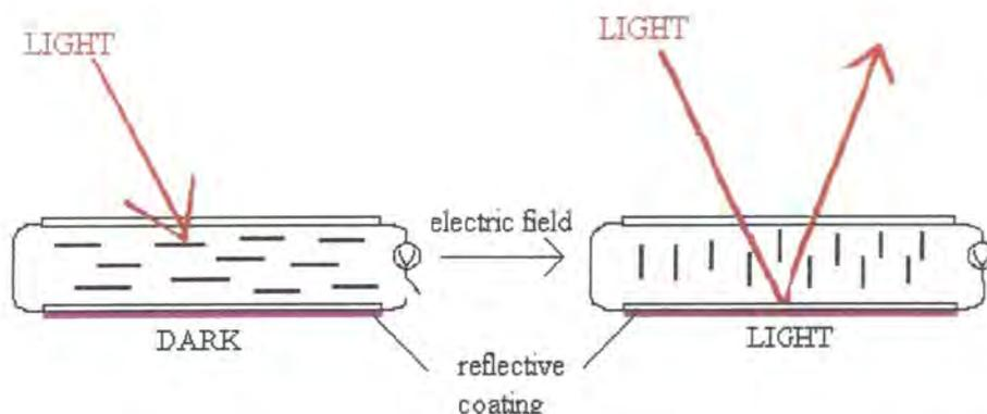
An electric field is applied across the cell which induces alignment with the field of the electrical dipole along the long axes of the liquid crystal molecules and
