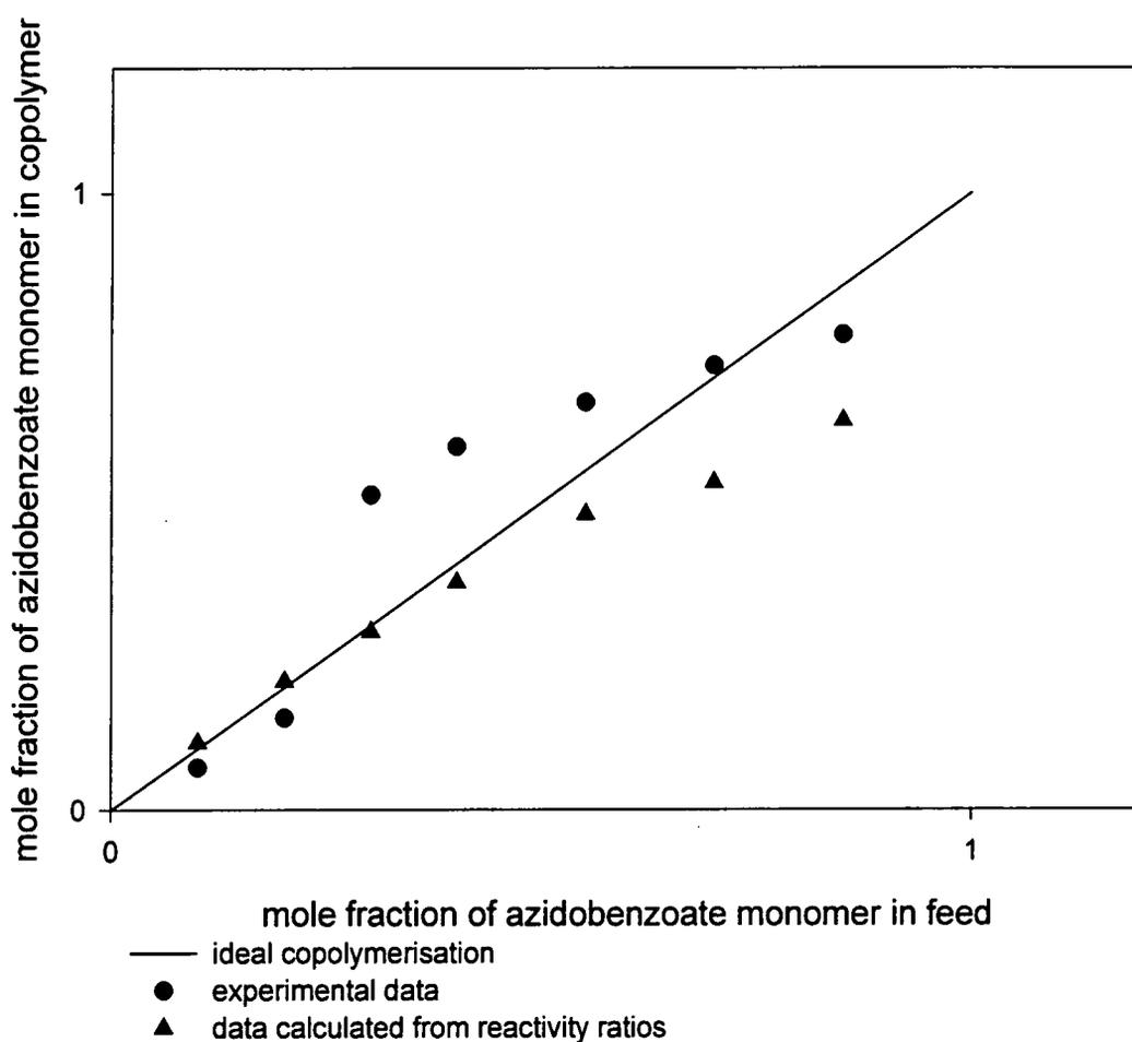
Graphs 4.1 and 4.2 each show three plots; the straight lines represent the results for an ideal copolymerisation where  $r_1 \approx r_2 \approx 1$ , the circles are points determined from experimental data ( $^1\text{H}$  NMR spectra of the copolymers and the feed mole fractions) and the triangles are the results of applying the values for the reactivity ratios obtained later in this section to the following equation.
