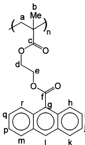
Table 2.8 Assignment of peaks of  $^1\text{H}$  NMR spectrum of homopolymer
