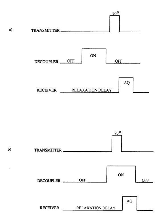
Fig 4.12 Pulse sequences for a) inverse gated decoupling and b) gated decoupling experiments
