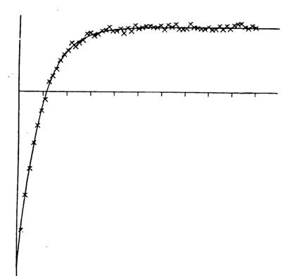
Fig 4.27 Magnetisation recovery after an inversion recovery experiment for water oxygen-17 spin-lattice relaxation in a concentrated sucrose solution.
