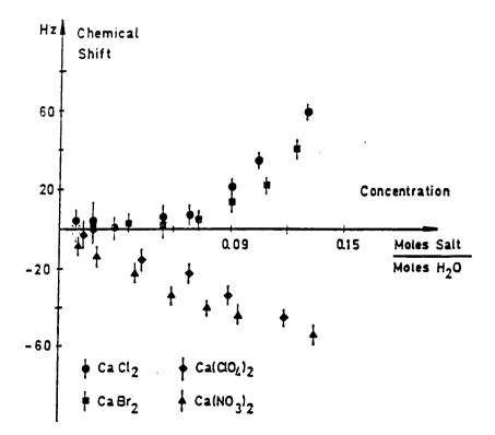
Fig 7.1 Chemical shifts of calcium-43 for aqueous solutions of calcium salts as a function of concentration. The reference is calcium chloride solution at infinite dilution.<sup>2</sup>
