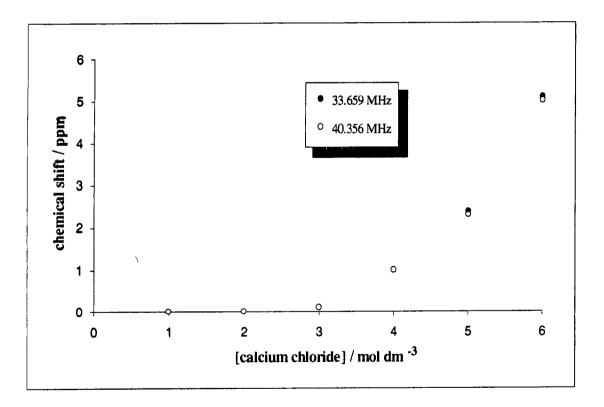
Fig 8.2 The dependence of <sup>43</sup>Ca chemical shift on calcium chloride concentration at two frequencies. The reference is 1.0 mol dm<sup>-3</sup> calcium chloride solution. A positive sign indicates a high frequency shift.
