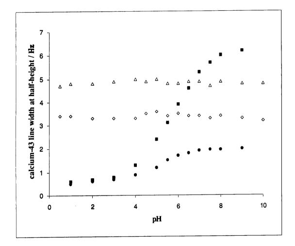
Fig 8.23 The dependence of the <sup>43</sup>Ca longitudinal relaxation time on pH for 1.0 mol dm<sup>-3</sup> calcium chloride + 1.0 mol dm<sup>-3</sup> sodium acetate and 1.0 mol dm<sup>-3</sup> calcium chloride + 1.0 mol dm<sup>-3</sup> sodium ascorbate solutions
