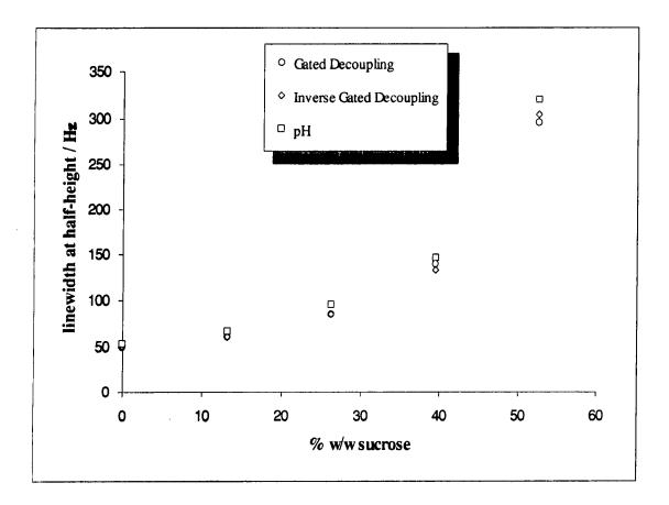
Fig 4.13 The variation of water oxygen-17 linewidth at half-height with sucrose concentration for gated decoupling (o), inverse gated decoupling (◊) and pH (□) experiments. SF = 33.909 MHz, temperature = 298 K.
