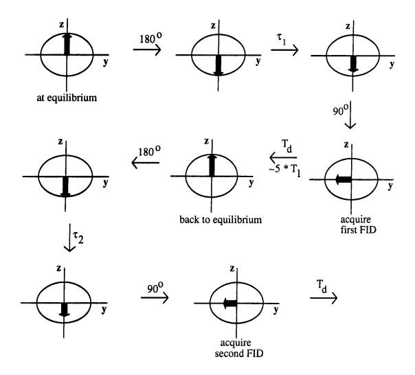
Fig 4.2 A diagrammatic representation of the pulse sequence for an inversion recovery experiment used to measure the spin-lattice relaxation time, T<sub>1</sub>
