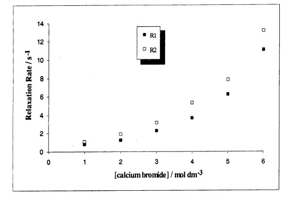
Fig 8.4 The variation of <sup>43</sup>Ca longitudinal and transverse relaxation rates as a function of calcium bromide concentration for aqueous calcium bromide solutions.
