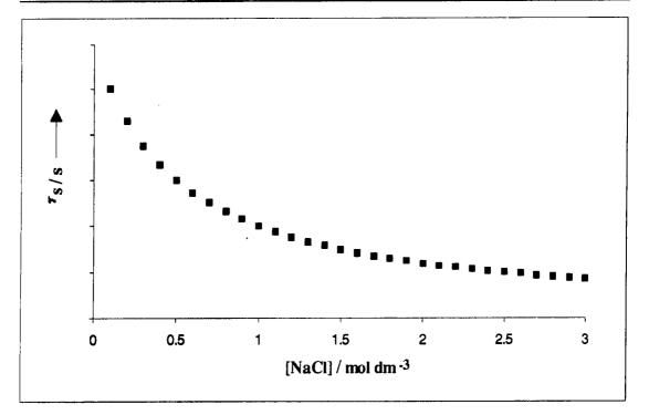
Fig 5.13 Theoretical plot of the correlation time of the slow component of bound water,  $\tau_s$ , as a function of sodium chloride concentration using Gordon's equation. The viscosity, activity coefficient,  $D_p^o$  and  $D_s^o$  terms are assumed to be constants and independent of salt concentration.
