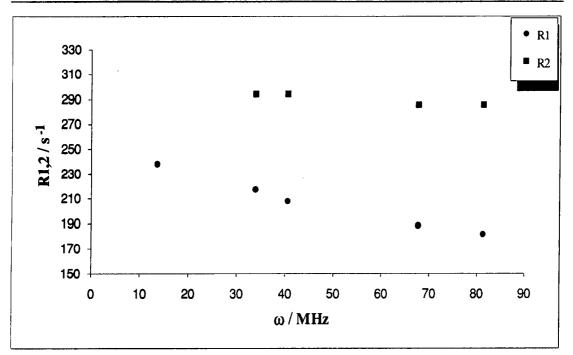
Fig 4.30 Variation of water oxygen-17 relaxation rates for an aqueous lysozyme solution with frequency. Concentration = 8.29 % w/w lysozyme, temperature = 298 K
