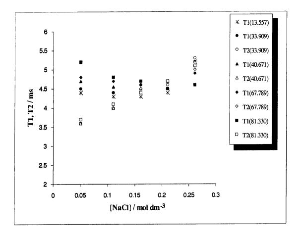
Fig 5.9 The effect of sodium chloride concentration on water oxygen-17 longitudinal and transverse relaxation times for an aqueous lysozyme solution. Concentration = 8.29 % w/w lysozyme, temperature =298 K
