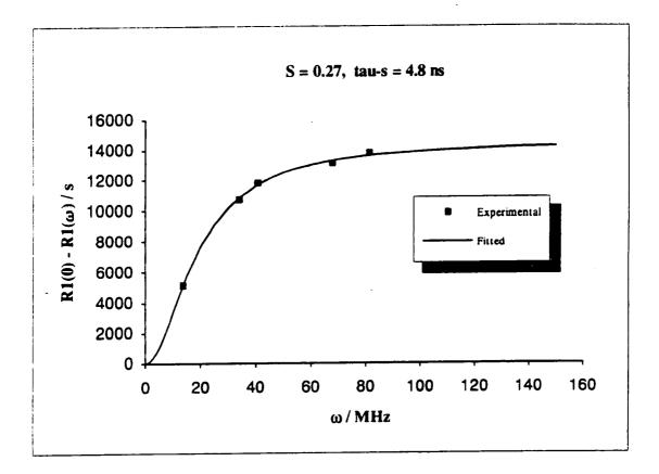
Fig 4.17 Comparison of the experimental and theoretical  $R_1(0) - R_1(\omega)$  data as a function of  $\omega$  for saturated sucrose solution.  $R_1(0)$  was estimated by extrapolating the experimental data to zero frequency. From the iterative fitting procedure S and  $\tau_s$  were found to be 0.27 and 4.8 ns, respectively
