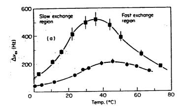
Fig 7.5 The temperature dependence of the calcium-43 linewidth in the presence of 0.86 mM TnC, 3.67 mM Ca<sup>2+</sup>, pH 7.0 (■); and 0.75 mM TnC, 5.92 mM Ca<sup>2+</sup>, pH 7.1 (●).<sup>3</sup>
