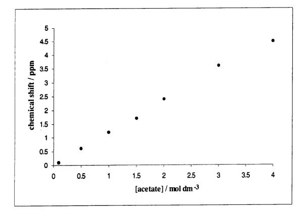
Fig 8.11 The variation of <sup>43</sup>Ca chemical shift as a function of acetate ion concentration for aqueous 1.0 mol dm<sup>-3</sup> calcium chloride + sodium acetate solutions. The reference is 1.0 mol dm<sup>-3</sup> calcium chloride solution. A positive sign indicates a high-frequency shift. No bulk susceptibility corrections were carried out.
