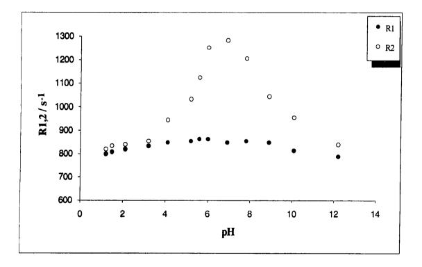
Fig 4.10 The dependence of water oxygen-17 relaxation rates on pH for a constant sucrose solution. Concentration = 52 % w/w sucrose, SF = 33.909 MHz, temperature = 298 K.
