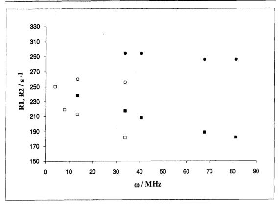
Fig 5.5 The variation of water oxygen-17 longitudinal and transverse relaxation rates for an aqueous lysozyme solution with frequency.
