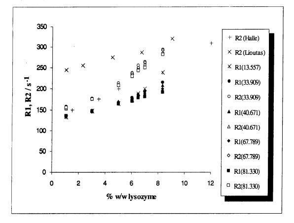
Fig 5.2 The dependence of water oxygen-17 longitudinal and transverse relaxation rates on lysozyme concentration for aqueous lysozyme solutions at various spectrometer frequencies. Filled symbols correspond to longitudinal and open symbols to transverse relaxation data obtained in this research.
