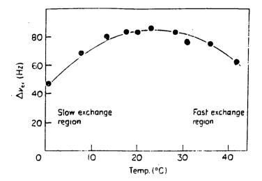
Fig 7.6 The temperature dependence of the calcium-43 linewidth for a solution of 1.7 mM phospholipase and 5.9 mM Ca<sup>2+</sup> at pH 7.4 <sup>26</sup>
