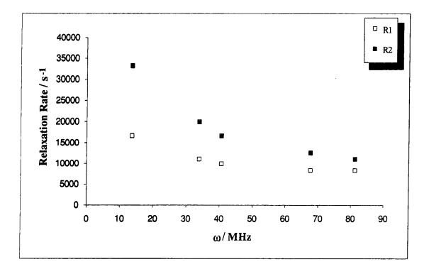
Fig 4.20 The variation of water oxygen-17 longitudinal and transverse relaxation rates on spectrometer frequency for a concentrated sucrose solution. Concentration = 73 % w/w sucrose, temp = 298 K, pH = 2.6
