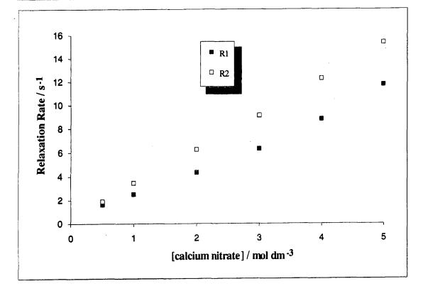
Fig 8.8 The variation of <sup>43</sup>Ca longitudinal and transverse relaxation rates as a function of calcium nitrate concentration for aqueous calcium nitrate solutions.
