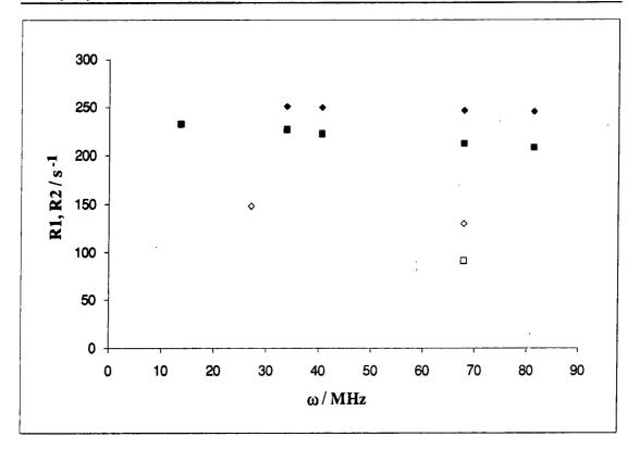
Fig 5.10 Variation of water oxygen-17 relaxation rates with frequency for an aqueous solution in the presence of 0.1 mol dm<sup>-3</sup> NaCl. Squares represent longitudinal relaxation, whereas diamonds represent transverse relaxation.
