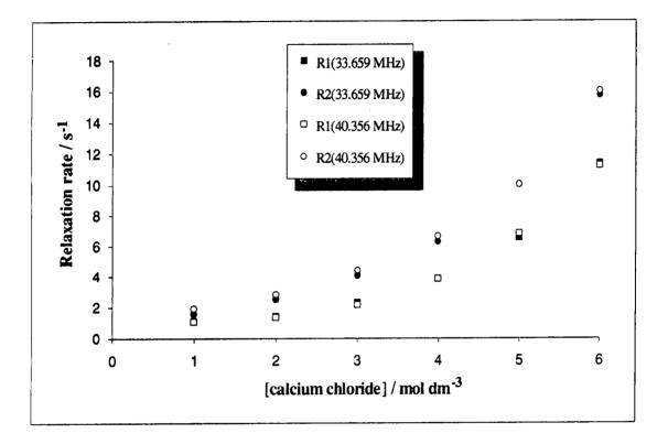
Fig 8.3 The variation of <sup>43</sup>Ca longitudinal and transverse relaxation rates as a function of calcium chloride concentration for aqueous calcium chloride solutions at two frequencies.
