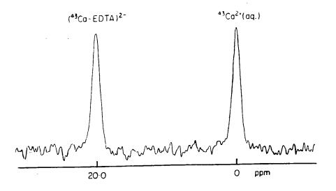
Fig 7.2 Calcium-43 NMR studies of an aqueous solution containing 4 mM  $Ca^{2+}$ and 2 mM EDTA at pH 7.<sup>3</sup>
