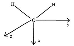
Fig 2.1 principal axis system for the electric field gradient tensor at the oxygen nucleus in an isolated water molecule. The water nuclei lie in the plane of the paper as do the x and y axes, whereas, the z axis is perpendicular to the plane of paper<sup>1,2</sup>
