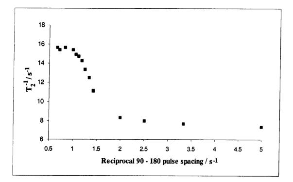
Fig 3.1 The dependence of water proton  $T_2^{-1}$  on the reciprocal of 90-180 ° CPMG pulse spacing for a sucrose solution. Concentration = 65.8 % w/w sucrose, pH = 2.8, temperature = 298 K
