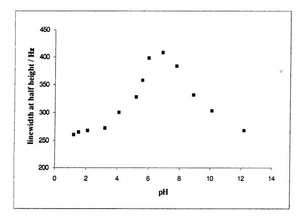
Fig 4.11 The dependence of water oxygen-17 linewidth on pH for a constant concentration of sucrose.
