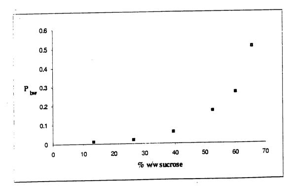
Fig 4.18 The variation of the fraction of bound water,  $P_{bw}$ , with sucrose concentration.  $\omega = 13.557$  MHz, S = 0.26,  $\tau_f = 123$  ps
