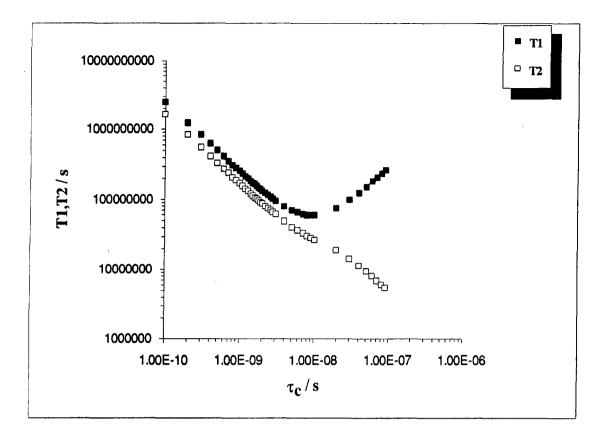
Fig 1.3 The dependence of  $T_1$  and  $T_2$  on correlation time,  $\tau_c$
