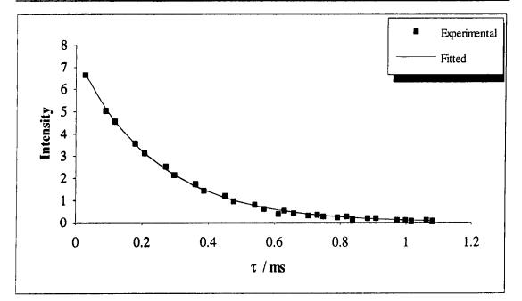
Fig 4.25 Plot of water oxygen-17 FID data to a single exponential transverse relaxation model for an aqueous sucrose solution. SF = 67.789 MHz, temperature = 298 K, pH = 2.6
