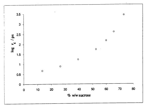
Fig 4.19 The dependence of the correlation time of the slow component of bound water,  $\tau_s$ , on sucrose concentration.  $\omega = 13.557$  MHz, S = 0.26
