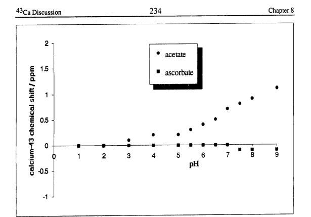
Fig 8.24 The dependence of <sup>43</sup>Ca chemical shift on pH for 1.0 mol dm<sup>-3</sup> calcium chloride + 1.0 mol dm<sup>-3</sup> sodium acetate and 1.0 mol dm<sup>-3</sup> calcium chloride + 1.0 mol dm<sup>-3</sup> sodium ascorbate solutions. The reference is 1.0 mol dm<sup>-3</sup> calcium chloride solution. A positive sign indicates a high-frequency shift. No bulk susceptibility corrections were carried out.
