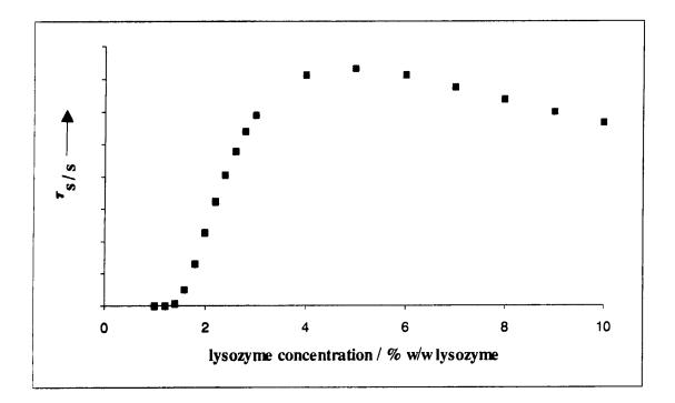
Fig 5.12 Theoretical plot of the correlation time of the slow component of bound water,  $\tau_s$ , as a function of lysozyme concentration using Gordon's equation<sup>2</sup> (eqn 5.1) in the absence of salt. The ionic activity term,  $dln\gamma^{\pm}/dC_p$ , is assumed to be a constant and independent of lysozyme concentration.
