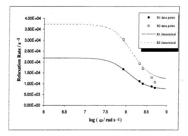
Fig 4.36 Comparison between the experimental and theoretical data for water oxygen-17 R<sub>1</sub> and R<sub>2</sub> in aqueous sucrose solution. The theoretical data are derived using Halle's model. The theoretical curve for transverse relaxation data includes the extra contribution.
