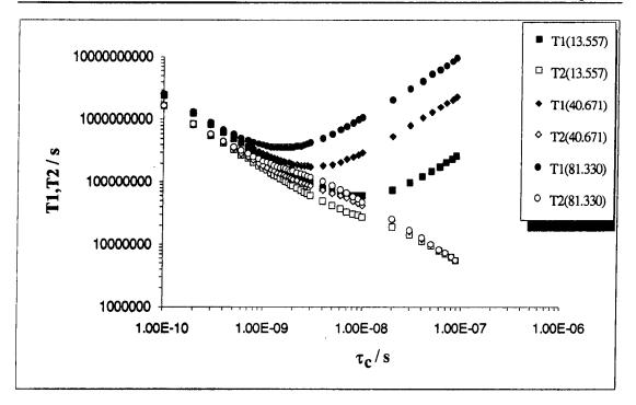
Fig 4.22 The dependence of  $T_1$  and  $T_2$  on  $\tau_c$  for different spectrometer frequencies.
