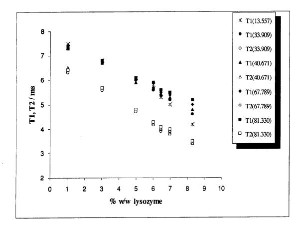
Fig 5.3 The dependence of water oxygen-17 longitudinal and transverse relaxation times on lysozyme concentration for aqueous lysozyme solutions at various spectrometer frequencies.
