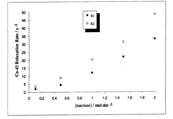
Fig 8.14 The dependence of <sup>43</sup>Ca longitudinal and transverse relaxation rates on sucrose concentration for 1.0 mol dm<sup>-3</sup> calcium chloride + sucrose solutions.
