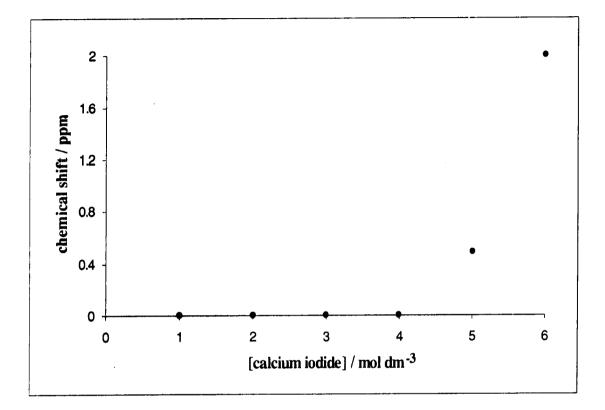
Fig 8.7 The dependence of <sup>43</sup>Ca chemical shift on calcium iodide concentration. The reference is 1.0 mol dm<sup>-3</sup> calcium chloride solution. A positive sign indicates a high-frequency shift. No bulk susceptibility corrections were carried out.
