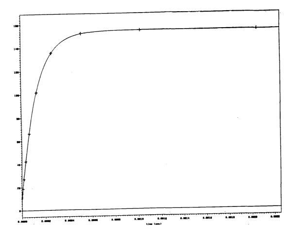
Fig 4.28 Lorentzian line fitting to an oxygen-17 signal for a concentrated sucrose solution. Concentration = 73 % w/w sucrose, SF = 33.909 MHz, pH = 2.6, temperature = 298 K
