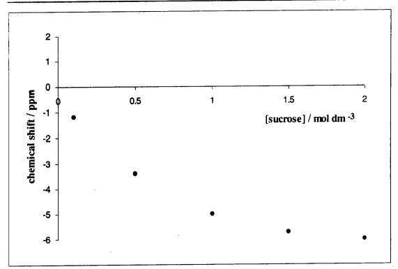
Fig 8.15 The dependence of <sup>43</sup>Ca chemical shift on sucrose concentration for 1.0 mol dm<sup>-3</sup> calcium chloride + sucrose solutions. The reference is 1.0 mol dm<sup>-3</sup> calcium chloride solution. A negative sign indicates a low-frequency shift. No bulk susceptibility corrections were carried out.
