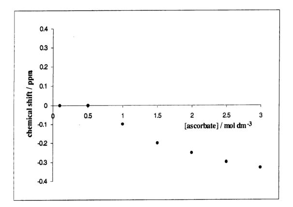
Fig 8.13 The dependence of <sup>43</sup>Ca chemical shift on ascorbate ion concentration for 1.0 mol dm<sup>-3</sup> calcium chloride + sodium ascorbate solutions. The reference is 1.0 mol dm<sup>-3</sup> calcium chloride solution. A negative sign indicates a low-frequency shift. No bulk susceptibility corrections were carried out.
