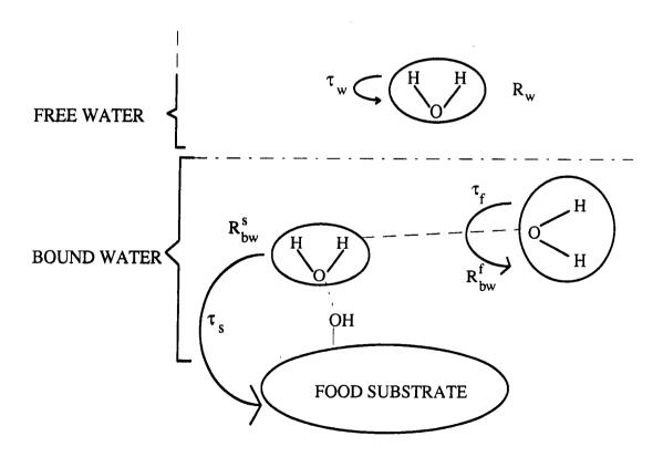
Fig. 2.3 Halle's model for a water-substrate system. The various symbols and terms are explained in text.
