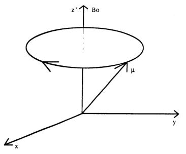
Fig 1.1 Precession of a magnetic moment  $\mu$  about an applied B<sub>0</sub>
