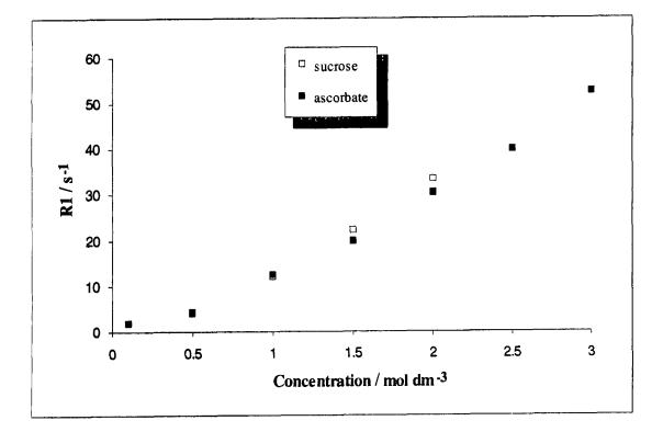
Fig 8.19 The dependence of <sup>43</sup>Ca longitudinal relaxation rates on sucrose and ascorbate ion concentrations for 1.0 mol dm<sup>-3</sup> calcium chloride + sucrose/sodium ascorbate solutions
