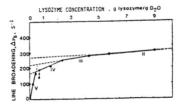
Fig 5.4 Water oxygen-17 NMR line broadening as a function of lysozyme concentration (data from Lioutas *et al.*<sup>6</sup>)
