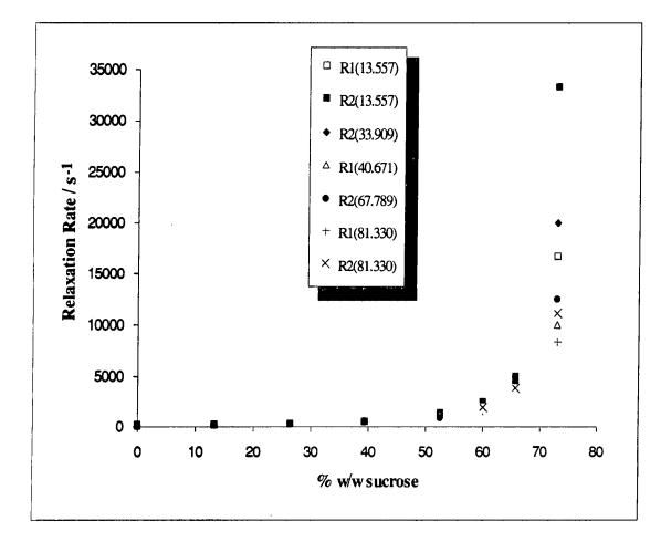
Fig 4.14 The dependence of water oxygen-17 relaxation rates,  $R_1$  and  $R_2$ , on sucrose concentration at different spectrometer frequencies.
