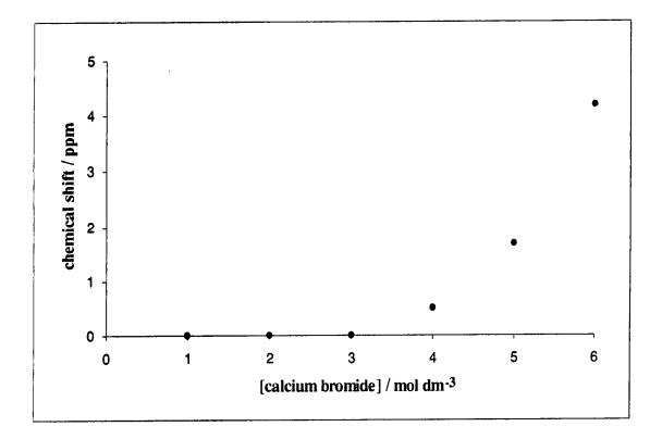
Fig 8.5 The dependence of <sup>43</sup>Ca chemical shift on calcium bromide concentration. The reference is 1.0 mol dm<sup>-3</sup> calcium chloride solution. A positive sign indicates a high-frequency shift. No bulk susceptibility corrections were carried out
