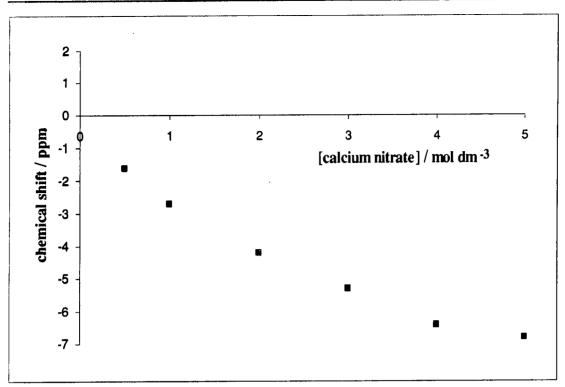
Fig 8.9 The dependence of <sup>43</sup>Ca chemical shift on calcium nitrate concentration for aqueous calcium nitrate solutions. The reference is 1.0 mol dm<sup>-3</sup> calcium chloride solution. A negative sign indicates a low-frequency shift. No bulk susceptibility corrections were carried out.
