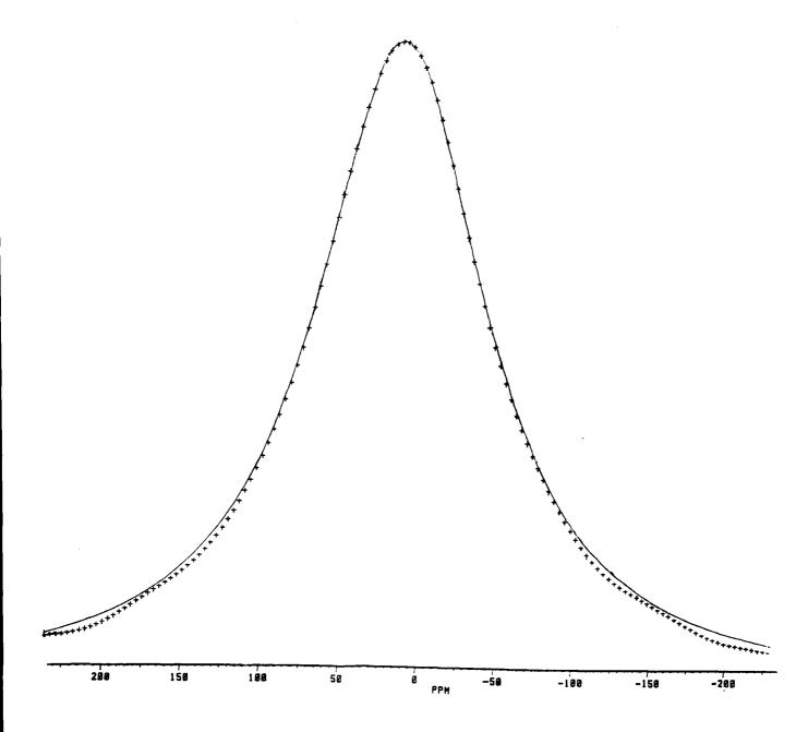
Fig 4.29 Lorentzian line fitting to an oxygen-17 signal for a concentrated sucrose solution. Concentration = 73 % w/w sucrose, pH = 2.6, SF = 81.330 MHz, temperature = 298 K
