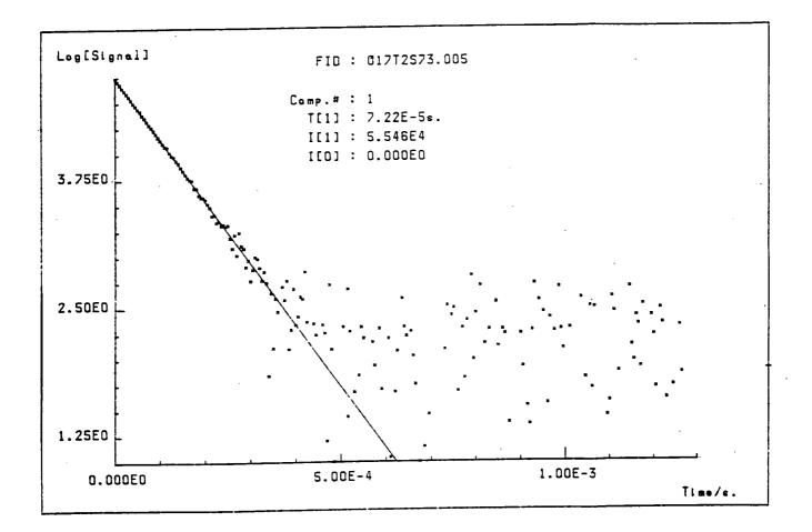
Fig 4.24 Quickfit plot for water oxygen-17 FID in a concentrated sucrose solution. Concentration = 73 % w/w sucrose, SF = 40.671 MHz, pH = 2.6, temperature = 298 K
