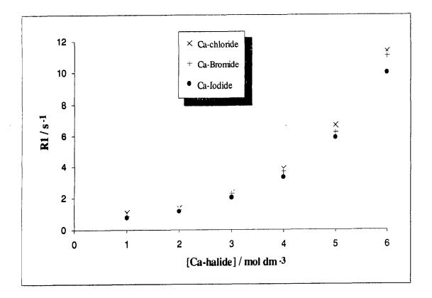
Fig 8.18 The dependence of the <sup>43</sup>Ca longitudinal relaxation rate on calcium halide concentration for aqueous calcium halide solutions.
