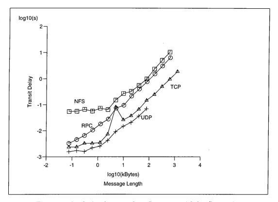
Figure 5: Analysis of protocol performance with log/log scale
