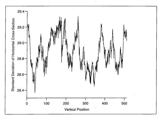
Figure 42: Standard deviation of horizontal cross-sections taken from "morevoids" with respect to vertical position in image
