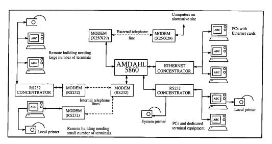
Figure 2: Schematic diagram of star-shaped data network
