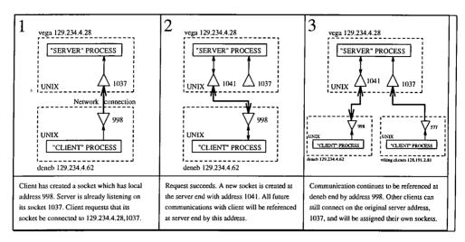
Figure 3: Socket behaviour during connection requests
