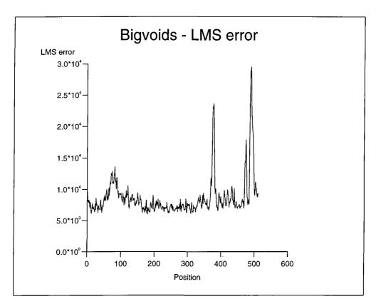
Figure 21: Detection performance based on line-by-line LMS deviation from average in figure 20
