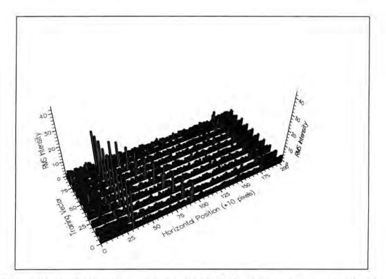
Figure 40: Synthetic void experiment: first half of training set, corresponding to presence of defect
