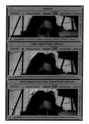
Figure 13: Frequency-domain filtering operation showing progressive loss of high spatial frequencies
