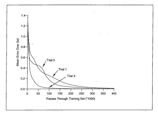
Figure 24: Training performance for MLP trained by backpropagation using training set of 10 random input/output relations, training parameter  $\eta=0.001$ . Network has 5 input, 7 hidden and 5 output nodes.
