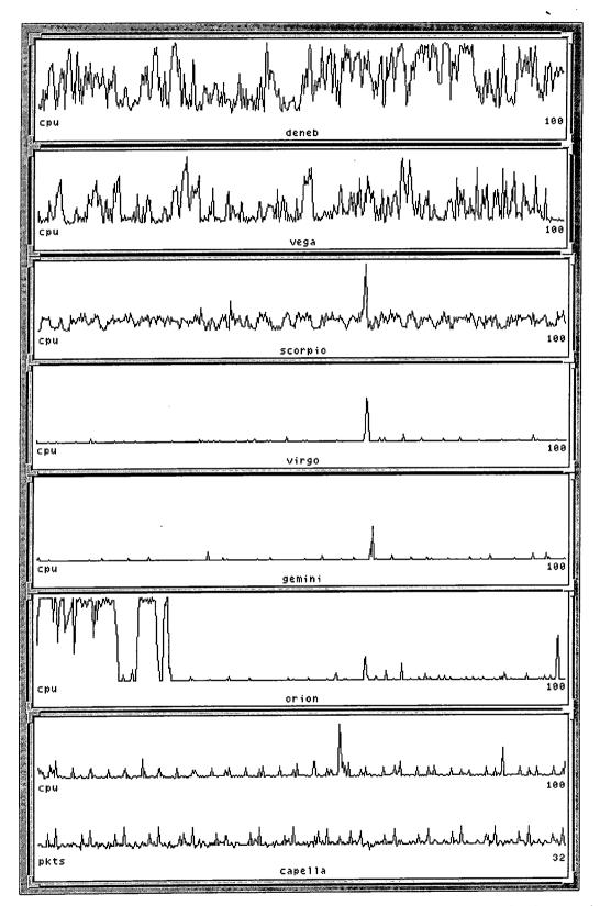
Figure 52: Processor utilisation for 6 of the 44 slave hosts during background application activity. CPU load and Ethernet traffic are shown for *capella*, the controlling node.
