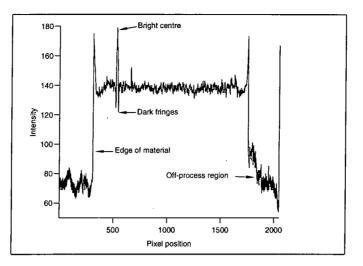
Figure 1: Image cross-section showing typical "void" defect
