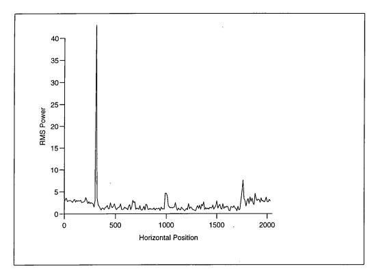
Figure 27: Raw data from figure 26 after RMS processing, reducing 2048 pixels to 204 floating-point power representations.
