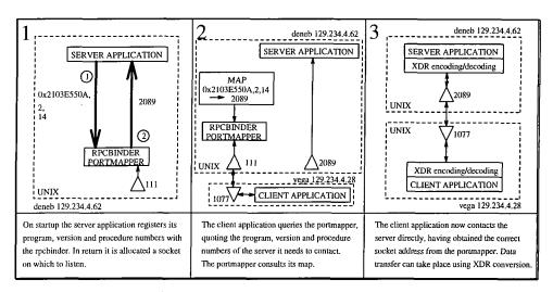
Figure 4: Procedure for typical RPC call
