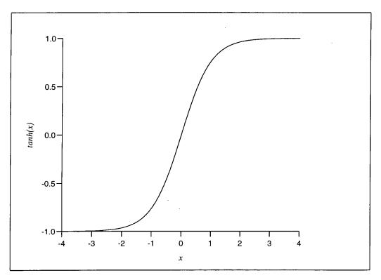
Figure 22: Non-linearity transfer function tanh(x)
