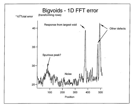
Figure 19: Detection performance based on line-by-line deviation from FFT average in figure 17
