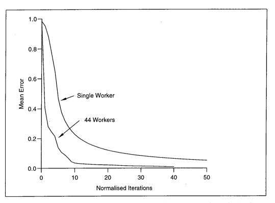
Figure 50: Comparison of training performance between single-node implementation and that with 44 hosts or slave workers.
