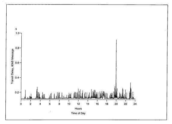
Figure 7: Ethernet transmission delay for 80kB TCP message
