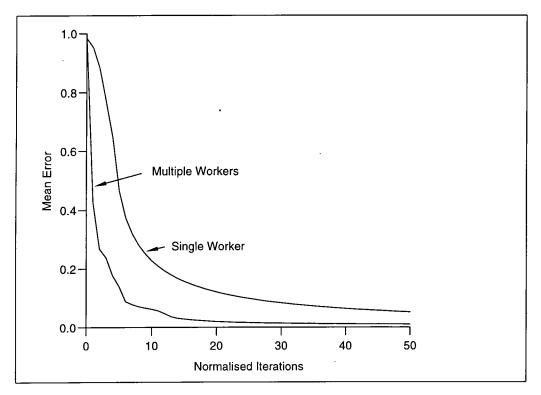
Figure 49: Comparison of training performance between single-node implementation and that with 19 hosts or slave workers.
