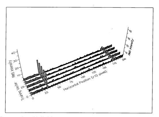
Figure 30: Second half of the training set used, consisting of 5 randomly-obtained RMS-processed cross-sections taken from "good" material.
