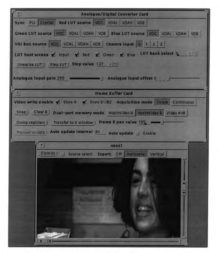
Figure 14: Interface to machine vision system via networked PC, including acquired image
