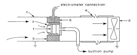
Fig. 5. Spore trap designed to measure spore charge directly. (a) All metal suction trap,
