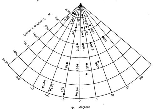
$\phi$ , degrees Fig. 4. Measured profiles of the mean electric field downwind of the stack. The electric field value at each site has units of kV m<sup>-1</sup>.
