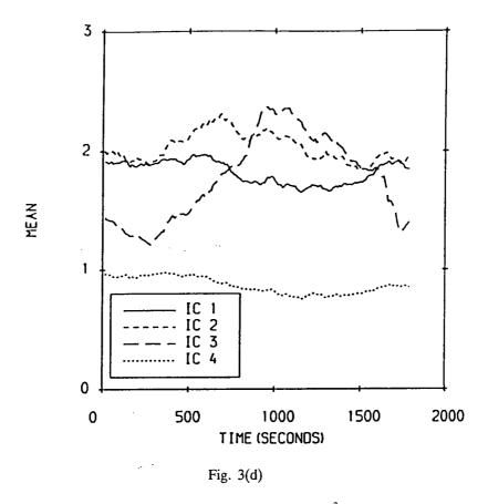
Fig. 3. The time variation of the mean concentration (in n Cm<sup>-3</sup>). In all cases the mean has been calculated at 200 equally spaced times. (a) Experiment 13, means calculated over 400 s. (b) Experiment 13, means calculated over 1200 s. (c) Experiment 16, means calculated over 400 s. (d) Experiment 16, means calculated over 800 s.
