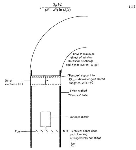
Figure 3. The ion generator.
