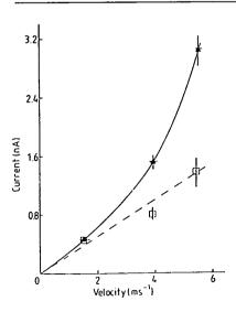
Figure 4. Probe calibration curve for saturated ( $\blacktriangle$ ) and nonsaturated ( $\Box$ ) conditions.
