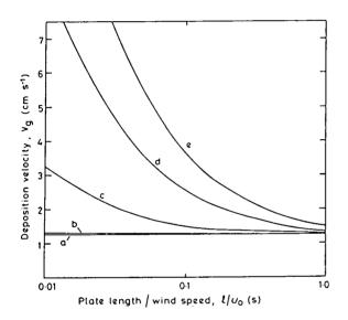
Fig. 3. Computed deposition velocity,  $v_g$ , for  $10\,\mu$ m radius charged particles (representing barley mildew spores) sedimenting onto a flat horizontal plate (representing barley leaves) as a function of  $l/u_0$  where l is the plate length and  $u_0$  is the windspeed, for charges per particle of (a) zero, (b)  $1 \times 10^4$ e, (c)  $1 \times 10^5$ e, (d)  $5 \times 10^5$ e and (e)  $1 \times 10^6$ e.
