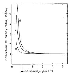
Fig. 2. Computed ratio,  $\alpha/\alpha_0$ , of collection efficiencies of charged and uncharged 10  $\mu$ m radius particles (representing barley mildew spores) impacting onto a 2.5 mm radius vertical cylinder (representing barley stems) as a function of wind speed,  $u_0$  for charges per particle of (b)  $1 \times 10^5$ e, (c) 5  $\times 10^5$ e and (d)  $1 \times 10^6$ e.
