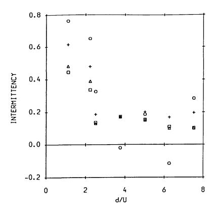
Fig. 9. Intermittency estimates plotted against downwind distance d(m) normalised by mean wind speed  $U(m s^{-1})$ .  $+ \theta_T = 2\sigma_N$ ,  $\Delta \theta_T$  set at change in slope,  $\Box$  intermittency determined by truncated normal fit,  $\bigcirc$  intermittency determined from (6). The stable cases are those at the two smallest values of d/U.
