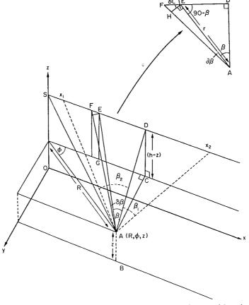
Fig. A.1. The coordinate position and associated parameters of a point A with reference to a line charge originating at a point S, height h above ground.
