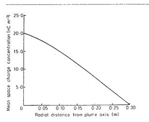
Figure 7 Mean space charge concentration profile obtained in turbulent flow conditions (2 m downstream, ion generator voltage 2.5 kV). For further details see text.
