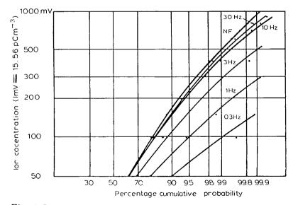
Fig. 4. Ion concentration frequency distributions at 10 m downwind.
