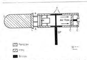
Figure 1 The ion generator: sectional drawing (electrical connections not shown). S, streamlining; L, lip; A, air intake; F, fan; M, fan motor; SP, support pillar; T, threaded section; R, ring (outer electrode); W, diametral wire (inner electrode); C, contact point.
