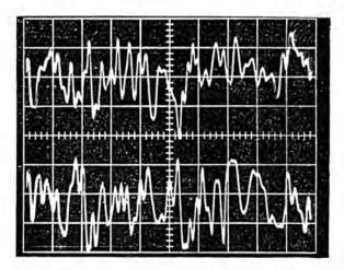
Figure 11 Space charge concentration fluctuations in turbulent flow 2 m downstream of the ion generator at two points 0.15 m on either side of the plume axis. (Otherwise, as figure 9, except that zero of lower trace is four divisions down.)
