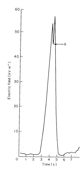
Figure 4. Observed variation of the electric field at a point under a moving charged spray. Spray velocity 0.71 m s<sup>-1</sup>.
