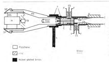
Figure 3 The ion collector: sectional drawing, SP, motor retaining spring; MS, motor support; M, fan (F) motor; FB, fan boss; FH, fan motor housing; T, threaded section; S, support pillar; TS, N, central electrode (C) tensioning spring and retaining nut; O, outer electrode; F, BNC socket mounting flange; CS, contact spring; EA, PTFE electrode assembly carrier; H, heater (12 W); 1, inlet tube.
