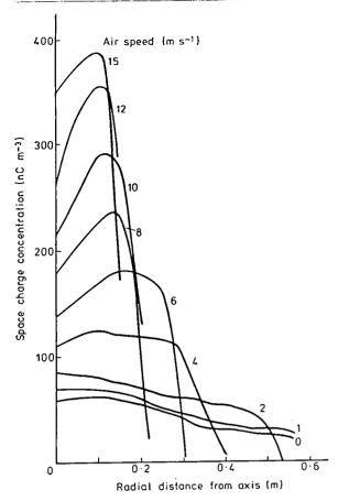
Figure 3 Radial concentration profiles at 1 m downstream.
