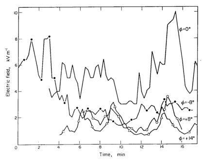
Fig. 5. Variation in electric field values at four crosswind positions defined by the  $\phi$  values, 490 m from the stack.
