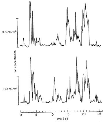
Figure 8. Simultaneous ion concentration measurements at vertically separated points. Upper trace, 1.5 m; lower, 1.0 m; ion collectors, 30 m downwind of a continuous point source of  $+0.15 \ \mu$ A at 2.2 m height; wind speed,  $\sim 2-5 \ m/s$ ; slightly unstable conditions, 22.8.75.
