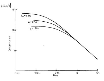
Fig. A4. Predicted values of ion puff concentration as a function of time.
