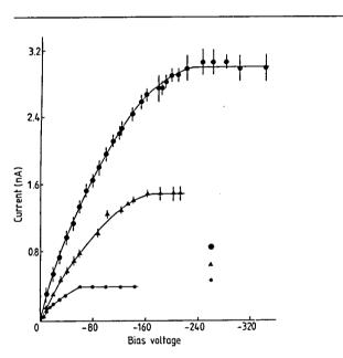
Figure 3. Characteristic curves for the probe.  $\bullet$ ,  $U = 5.4 \text{ m s}^{-1}$ ;  $\blacktriangle$ ,  $U = 3.9 \text{ m s}^{-1}$ ; \*,  $V = 1.5 \text{ m s}^{-1}$ .
