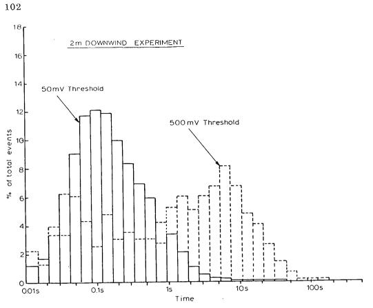
Fig. 7. Burst return period distributions obtained using 'SHADA'.
