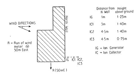
Fig. 2. Arrangements for the pulsed source (Nov. 1982) experiments.
