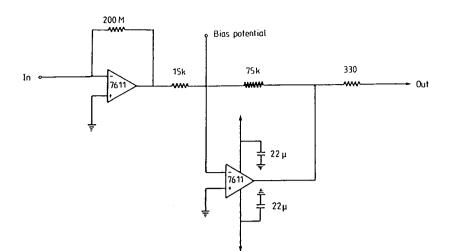
Figure 2. Head amplifier circuit for the ion probe.
