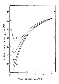
Fig. 1. Computed collection efficiency,  $\alpha$ , for charged 10  $\mu$ m radius particles (representing barley mildew spores) impacting onto a 2.5 mm radius vertical cylinder (representing barley stems) as a function of wind speed,  $u_0$ , for charges per particle of: (a) zero, (b)  $1 \times 10^5$ e, (c) 5  $\times 10^5$ e and (d)  $1 \times 10^6$ e.
