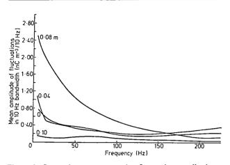
Figure 6 Space charge concentration fluctuation amplitude as a function of frequency in low-turbulence conditions (at 2 m downstream) with an air speed of 5 m s<sup>-1</sup> and 2.5 kV applied to the ion generator. Numbers on curves indicate distances from plume axis, i.e. radial positions.
