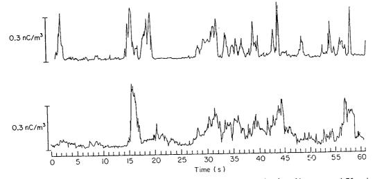
Figure 9. Simultaneous ion concentration measurements at vertically separated points. Upper trace, 1.75 m; lower 0.25 m; ion collectors. 30 m downwind of a continuous point source of  $+0.15 \,\mu$ A at 2.2 m height; wind speed,  $\sim 2-5$  m/s; slightly unstable conditions, 22.8.75.
