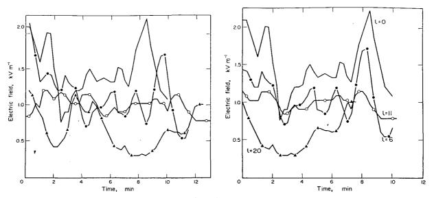
Fig. 6. (i) The variation in electric field at four sites downwind of the stack: 1300 m ----; 1650 m -----; 2057 m -O-O---; 2790 m -▲-▲-.
