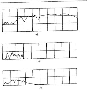
Figure 6. Typical signals obtained from the ion flux probe located at downwind distances of (a) 5 m, (b) 10 and (c) 15 m. Vertical scale: 0.1 V per division; horizontal scale: (a) 50 ms/div. (b) 0.2 s/div. (c) 0.2 s/div.
