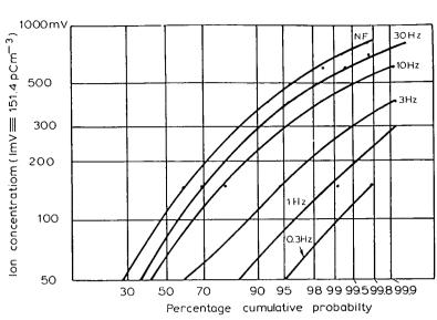
Fig. 2. Ion concentration frequency distributions at 2 m downwind.
