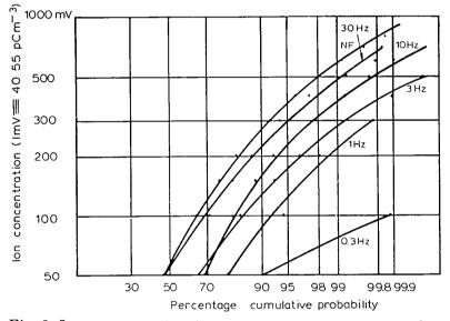
Fig. 3. Ion concentration frequency distributions at 5 m downwind.
