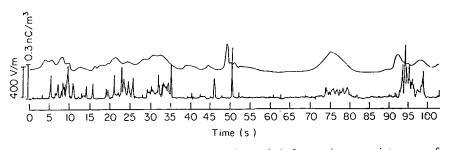
Figure 5. Ion concentration and electric field variations downwind of a continuous point source of positive ions. Ion source height, 2.2 m; output, 0.15  $\mu$ A; ion collector, 30 m downwind at 1.5 m height; field mill, 25 m downwind on ground; meteorological conditions, slightly unstable, 22.8.75.
