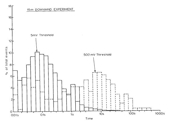
Fig. 8. Burst return period distributions obtained using 'SHADA'.
