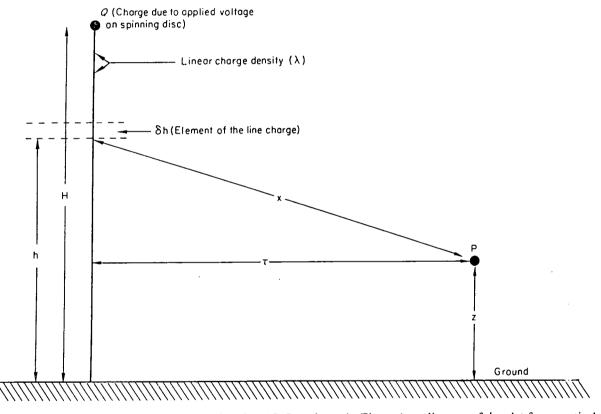
Figure 3. The linear space charge approximation. H, R and z as in Figure 1; r, distance of droplet from vertical axis of disc.
