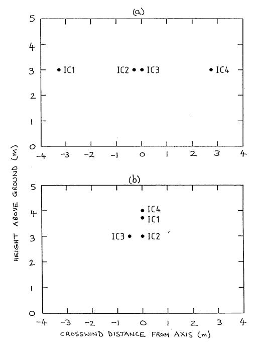
Fig. 1. The ion collector arrays, looking downwind from the source. (a) Experiments 8-11. Source height 3 m. (b) Experiments 13, 16, 17. Source height 3.5 m.
