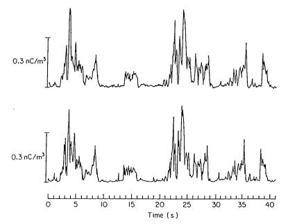
Figure 7. Simultaneous ion concentration measurements at vertically separated points. Upper trace, 1.5 m; lower, 1.45 m; ion collectors, 30 m downwind of a continuous point source of  $\sim 0.15 \,\mu$ A at 2.2 m height; wind speed, 2-5 m/s; slightly unstable conditions, 22.8.75.
