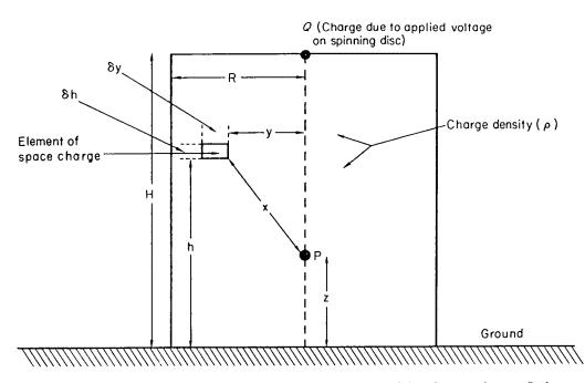
Figure 1. The cylindrical space charge approximation. H, Maximum height of space charge; R, its outer radius; z, height of a point P along the axis.
