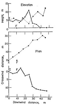
Fig. 8. Examples of computed ion plume configurations for time A (\_\_\_\_\_) and time B (....) of Fig. 7. (see text.) I = ion source. F = field mill.
