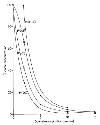
FIG. 7. Downwind concentration distribution at various probability levels.
