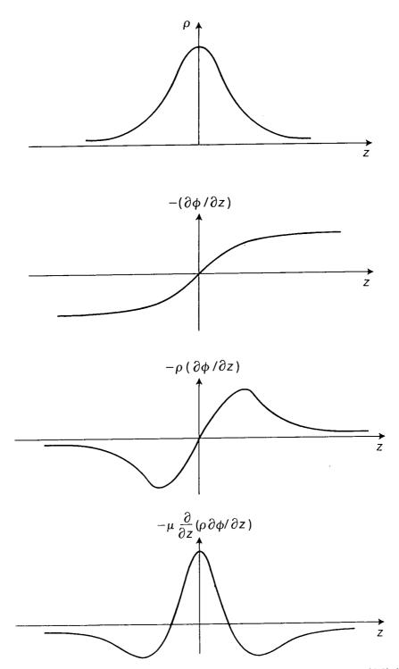
FIG. 1. Schematic diagram showing the effect of the electrostatic term in equation (6.2) for an initial charge distribution  $\rho(z, 0)$  proportional to exp  $(-kz^2)$ .
