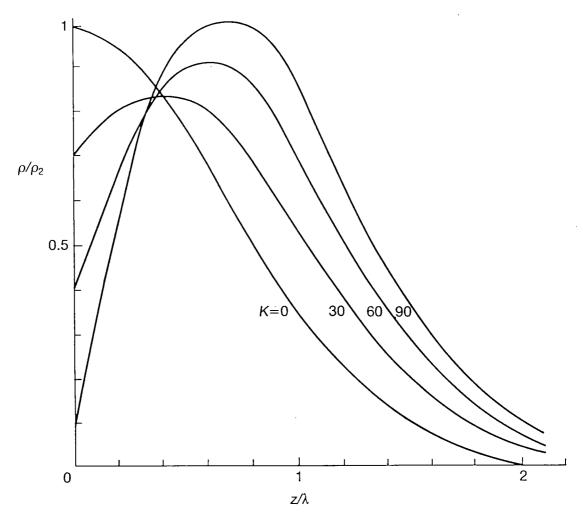
FIG. 2. Sketches showing the charge distribution for  $\alpha t = 0.01$  for various values of K defined in equation (6.13).
