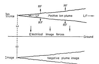
Fig. 1. Electrical forces influencing ion plumes. The positive ion source at height H produces a positive ion plume. The electrical mirror image is negative. There are also outward radial forces of electrostatic repusion
