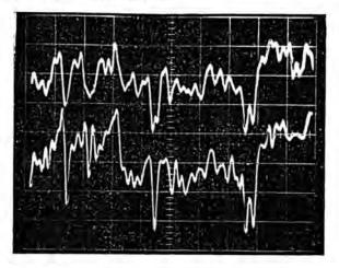
Figure 9 Space charge concentration fluctuations in turbulent flow at 2 m downstream of the ion generator at two points 0.025 m on either side of the plume axis. Vertical axis (increasing downwards)  $8.3 \text{ nC m}^{-3}$ /large division; horizontal axis 0.2 s/division. Zero of upper trace is at top; that of lower trace is two divisions down. See text for further details.
