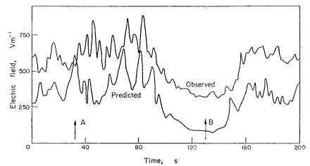
Fig. 7. Time variations of observed electric field at the surface 10 m downwind of an ion source 5 m high, together with values computed from bivane data. Mean wind speed  $= 3.4 \text{ ms}^{-1}$ . The nearly constant difference of about 250 Vm<sup>-1</sup> corresponds to the prevailing natural electric field upwind of the source.
