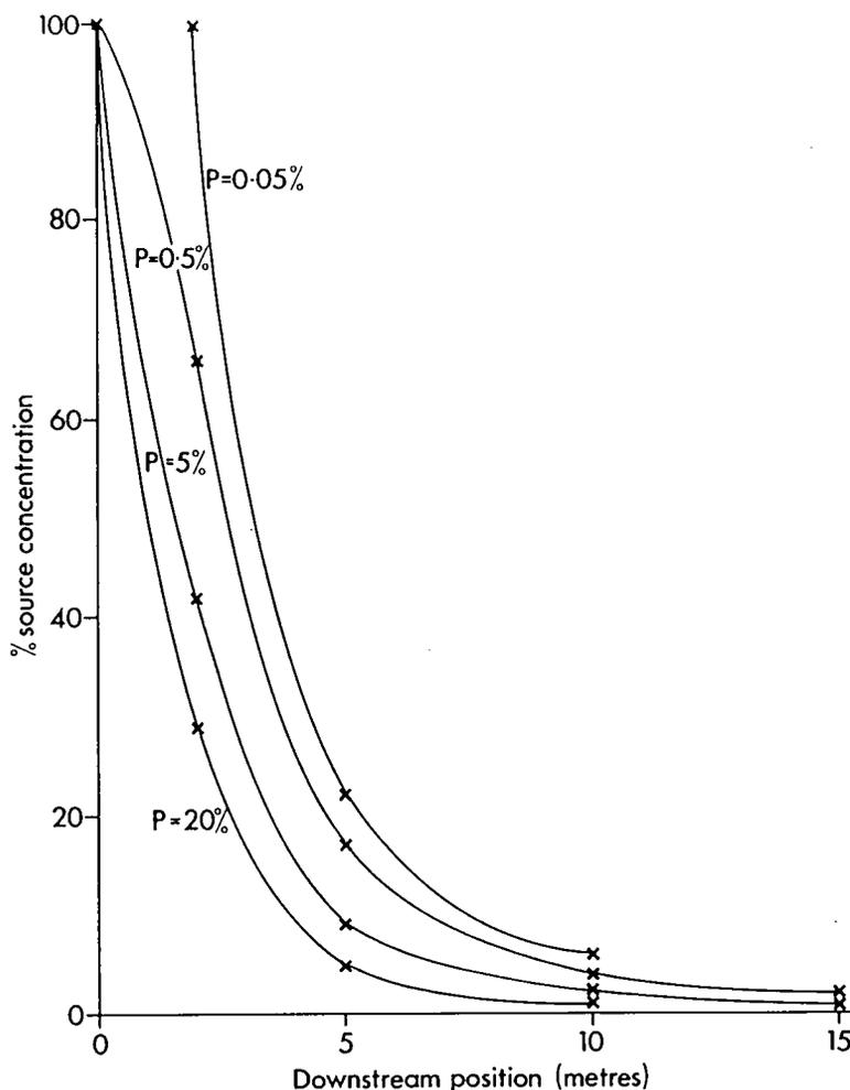
FIG. 7. Downwind concentration distribution at various probability levels.
