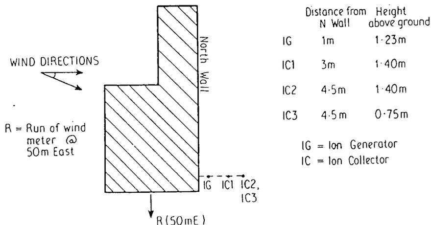
Fig. 2. Arrangements for the pulsed source (Nov. 1982) experiments.
