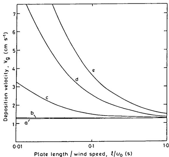
Fig. 3. Computed deposition velocity,  $v_g$ , for  $10 \mu\text{m}$  radius charged particles (representing barley mildew spores) sedimenting onto a flat horizontal plate (representing barley leaves) as a function of  $l/u_0$  where  $l$  is the plate length and  $u_0$  is the windspeed, for charges per particle of (a) zero, (b)  $1 \times 10^4 e$ , (c)  $1 \times 10^5 e$ , (d)  $5 \times 10^5 e$  and (e)  $1 \times 10^6 e$ .
