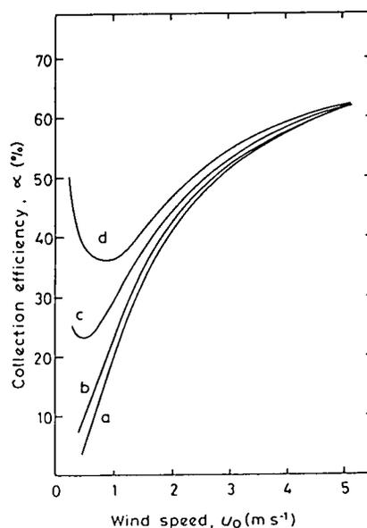
Fig. 1. Computed collection efficiency,  $\alpha$ , for charged  $10 \mu\text{m}$  radius particles (representing barley mildew spores) impacting onto a  $2.5 \text{ mm}$  radius vertical cylinder (representing barley stems) as a function of wind speed,  $u_0$ , for charges per particle of: (a) zero, (b)  $1 \times 10^5 e$ , (c)  $5 \times 10^5 e$  and (d)  $1 \times 10^6 e$ .
