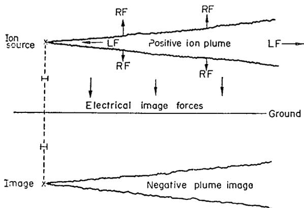
Fig. 1. Electrical forces influencing ion plumes. The positive ion source at height  $H$  produces a positive ion plume. The electrical mirror image is negative. There are also outward radial forces of electrostatic repulsion (RF) and longitudinal forces of repulsion (LF).
