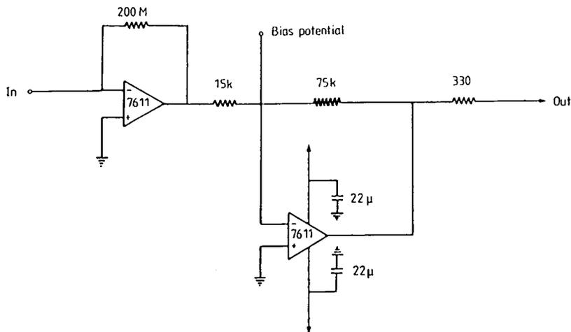
Figure 2. Head amplifier circuit for the ion probe.
