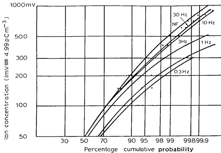
Fig. 5. Ion concentration frequency distributions at 15 m downwind.
