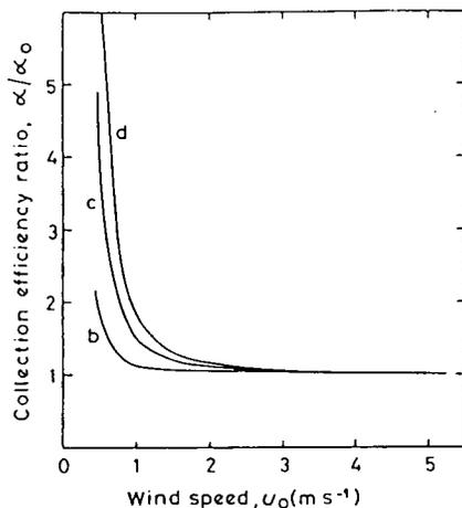
Fig. 2. Computed ratio,  $\alpha/\alpha_0$ , of collection efficiencies of charged and uncharged  $10\ \mu\text{m}$  radius particles (representing barley mildew spores) impacting onto a  $2.5\ \text{mm}$  radius vertical cylinder (representing barley stems) as a function of wind speed,  $u_0$  for charges per particle of (b)  $1 \times 10^5 e$ , (c)  $5 \times 10^5 e$  and (d)  $1 \times 10^6 e$ .
