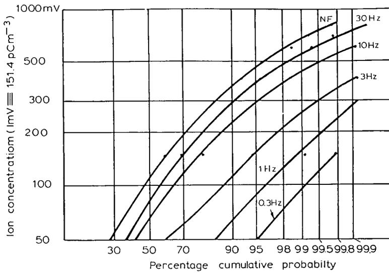
Fig. 2. Ion concentration frequency distributions at 2 m downwind.
