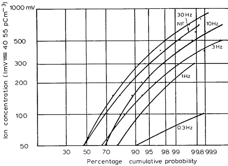
Fig. 3. Ion concentration frequency distributions at 5 m downwind.
