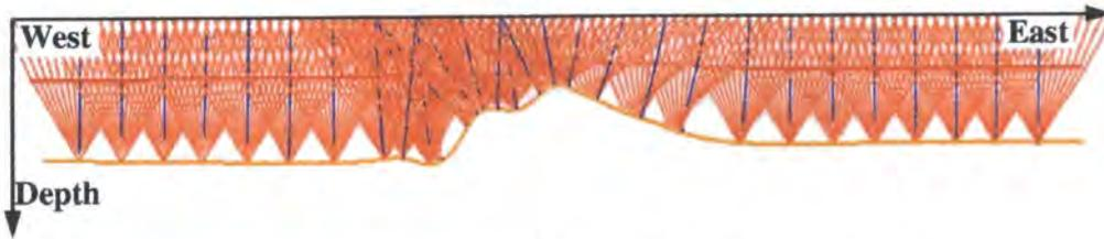
*Figure 3-4: Cross-section showing the calculated ray fans*
