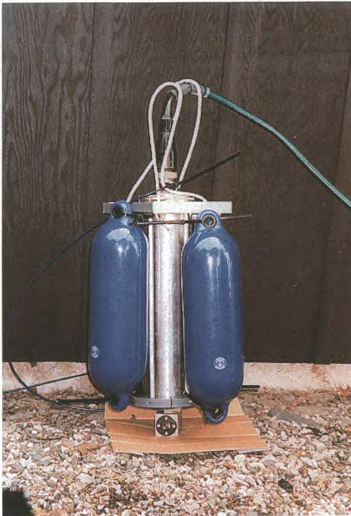
Figure 3.2 Field fluorometer used for in situ measurement of chlorophyll a .
