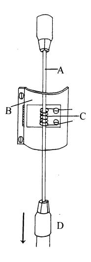
Fig 2.2: Microelectrode puller.
