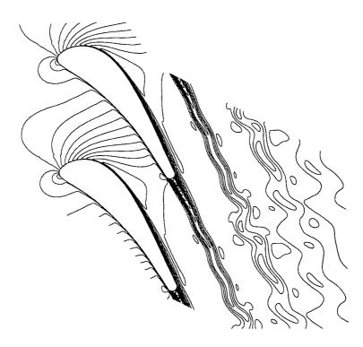
Fig. 6-33 Contours of Mach Number by Solving Unsteady NS Equation ( Dlimit =10% )
