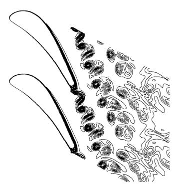
Fig. 6-18 Contours of Instantaneous Entropy around Turbine Blade in a Laminar Flow Case
