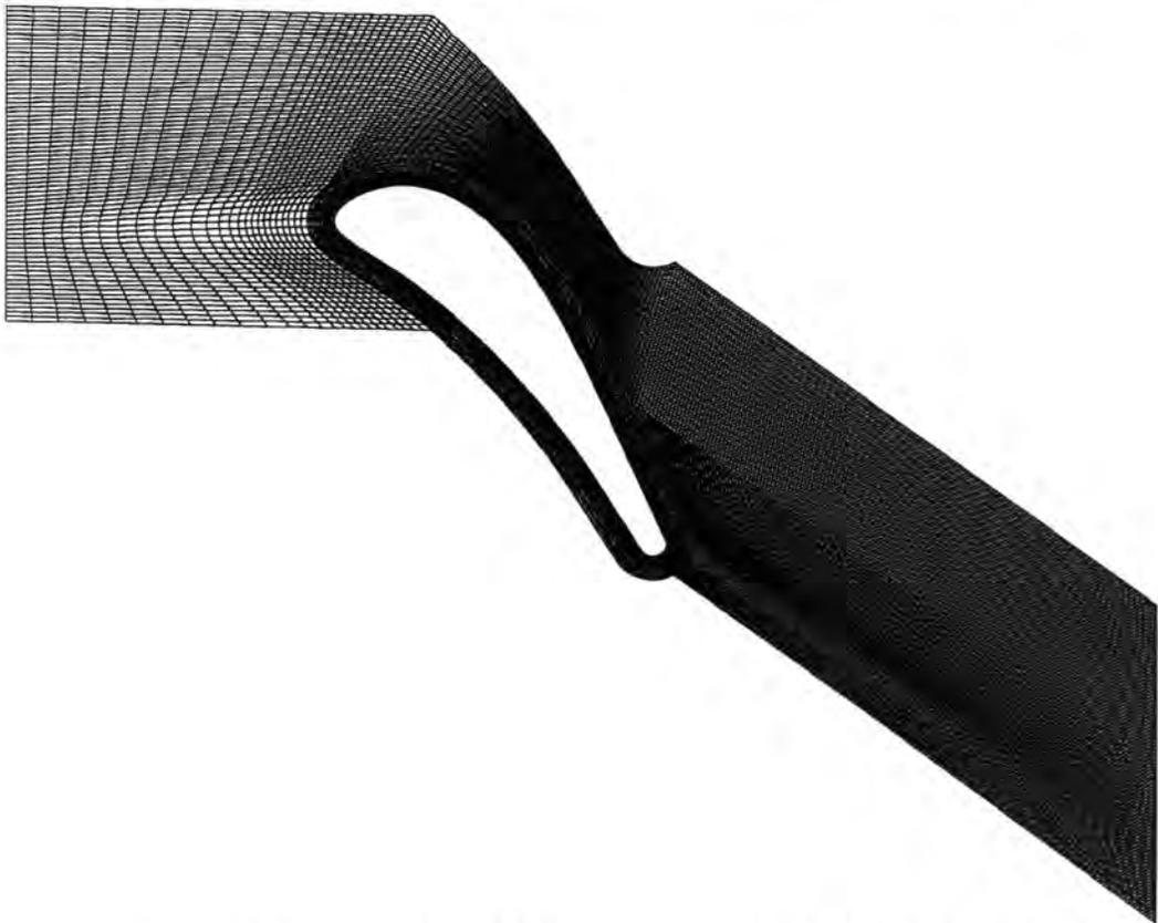
**Fig. 6-15 Computational Mesh around VKI Turbine Cascade**
