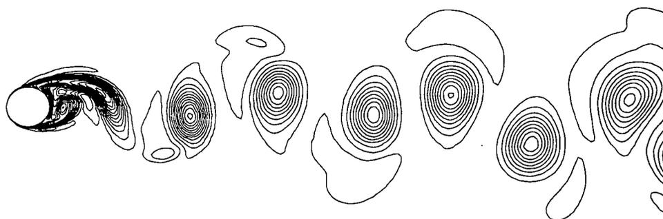
**Fig. 6-7 Contours of Instantaneous Entropy around Cylinder**
