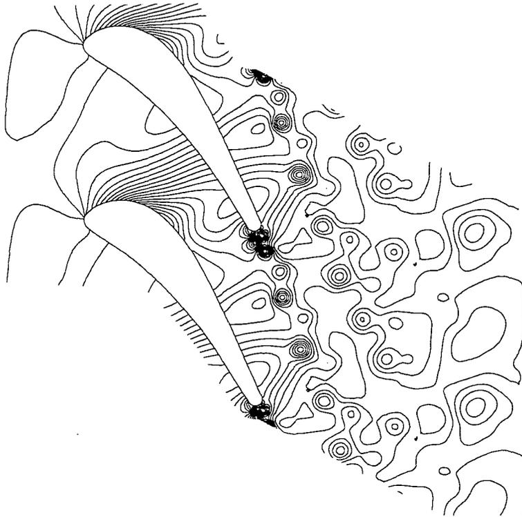
**Fig. 6-17 Contours of Instantaneous Static Pressure around Turbine Cascade in a Laminar Flow Case**
