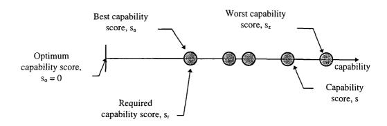
Figure 4.4: Representation of a group of collated capability scores
