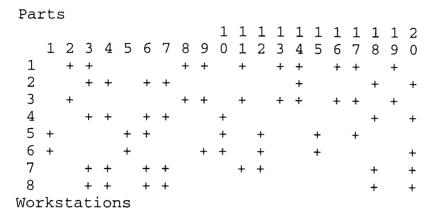
Figure 2.1 Example machine part incidence matrix (discussed in Section 2.4)
