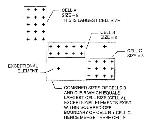
Figure 2.12: Merging cells to reduce exceptional elements
