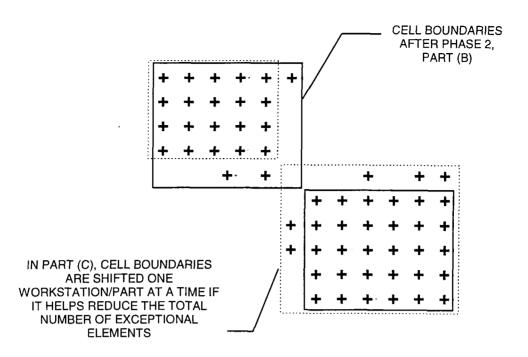
Figure 2.11: Shifting cell boundaries to reduce exceptional elements
