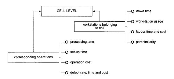
Figure 4.10: Lower level PCS values represented at higher levels
