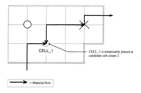
Figure 3.2: Material handling at a cell positioned at a candidate cell centre
