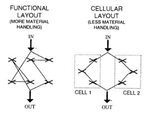
Figure 1.2: Material handling advantages of cellular layout over functional layout
