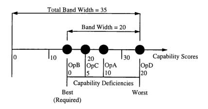
Figure 4.12: Band width diagram for example data
