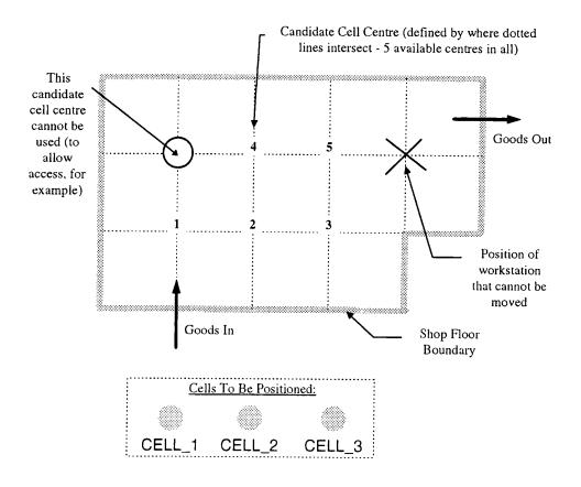
Figure 3.1: Example outlining the cell positioning problem
