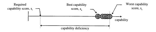
Figure 4.5: Effect of setting the required capability score nearer the optimum value
