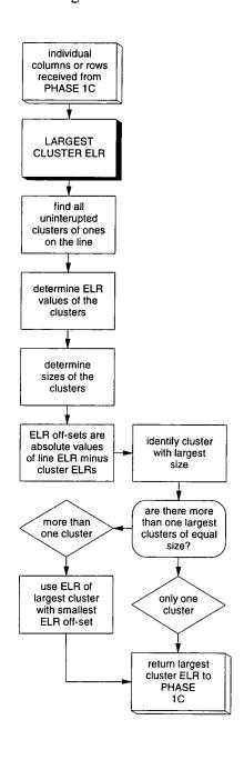
Figure 2.6: Determining largest cluster ELR value to be used in Phase 1, step c
