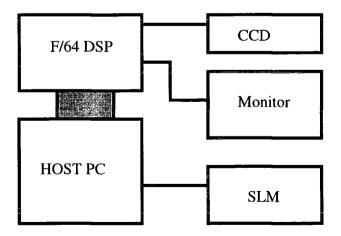
Figure 5.7. The image processing and control hardware system.
