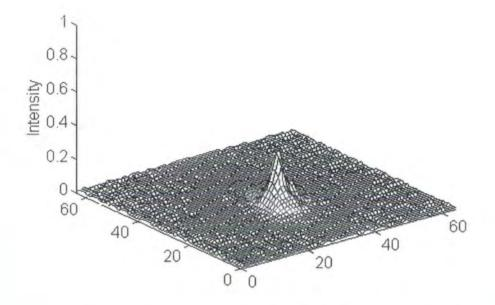
Figure 7.8. The corrected PSF. The Strehl ratio was 33%.
