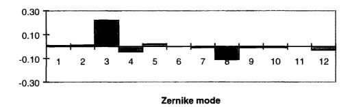
Figure 8.17. The Shack-Hartmann measured power spectrum of mode 3.
