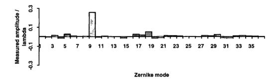
Figure 8.14. The Zernike power spectrum of a mode 9 aberration introduced by the Hex 69 of amplitude  $0.25\lambda$ . There is some crosstalk into mode 18.
