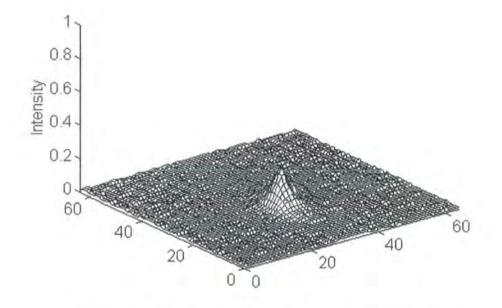
Figure 7.7. The aberrated PSF. The Strehl ratio was 23%.
