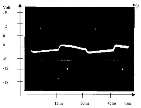
Figure 4.7. CRO trace showing the voltage across pixel (32,22) with a ramp function applied across the whole array. The ramp goes from 0V to  $\pm 2V$  and the spikes are  $\pm 10.9V$  and  $\pm 11V$ . The waveform is an image of what has been applied to the whole array.
