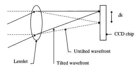
Figure 3.3. A single lenslet of the Shack-Hartmann array. An unaberrated beam is represented by the dotted line. The beam with a tilt across it is represented by the solid line. The amount of tilt can be calculated from  $\delta x$ , the displacement of the spot on the CCD chip.
