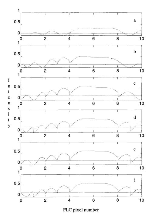
Figure 5.5 a, b, c, d, e, f (ii). The simulated interferograms. The top one (a) is the uncorrected interferogram. The horizontal line is the threshold value. The vertical scale is the intensity, the horizontal is the FLC pixel number.
