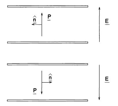
Figure 2.9 The SSFLC. The layers of smectic molecules are in the plane of the page. The director,  $\hat{\mathbf{n}}$ , is shown as its projection onto the plane of the page. It is at an angle of 22.5° to the perpendicular of the page's plane. The application of an electric field causes the switching between the two states.
