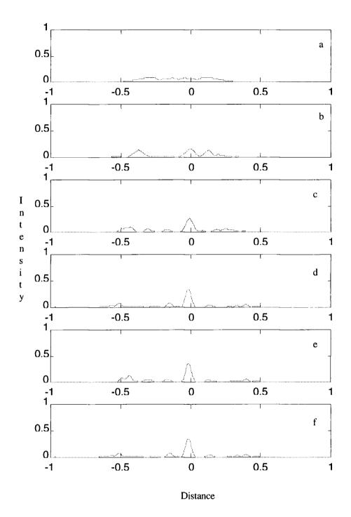
Figures 5.5 a, b, c, d, e, f(i). The top (a) is the aberrated PSF. The one below (b) is the first correction and the next 4 are the following corrections. Figure (d) is identical to (f). The vertical scale is normalised intensity, the horizontal is distance in arbitrary units.
