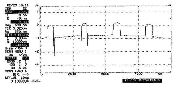
Figure A2.6. An Alpha-step profile of the device. Note how the graphite rods protrude from the surface by  $\sim 2\mu m$ .
