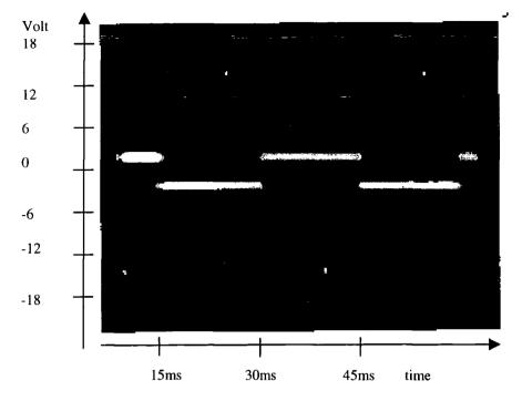
Figure 4.4. CRO trace showing the voltage across an individual pixel when the whole device is switched fully on. The square wave is  $\pm 2V$  and the spikes (only seen as dots on this plot) are  $\pm 15V$ . The period is 30ms.
