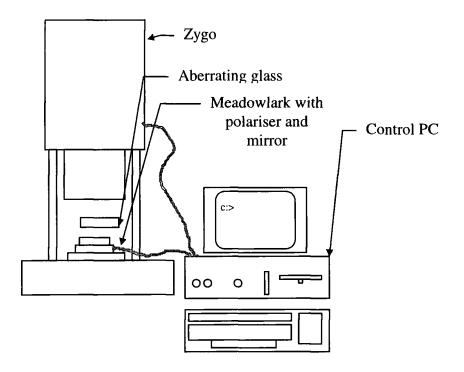
Figure 8.2. The Hex69 in the Zygo interferometer. The Hex69 is mounted on top of an optically flat mirror and a high quality polariser is placed on top of the Hex69. A PC controls both the Hex69 and the Zygo, however the correction is not real time.
