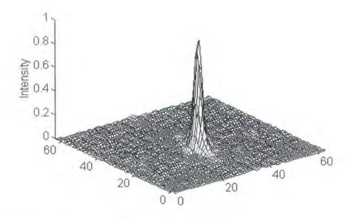
Fig 7.3 The unaberrated PSF.
