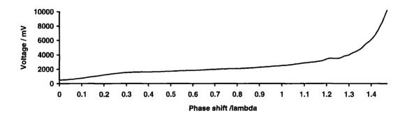
Figure 6.6. The voltage versus phase shift response of the Hex69. The polynomial fitted is a 6<sup>th</sup> order with a correlation coefficient, r, of 0.998776
