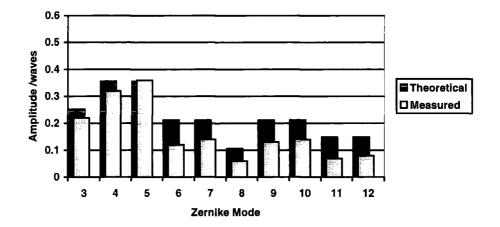
Figure 6.11. The RMS power spectrum of the ATS. This data was taken over 4552 frames.
