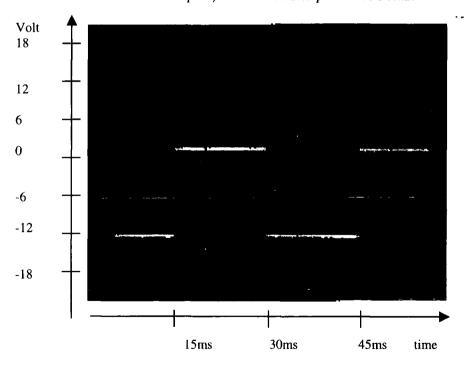
Figure 4.5. CRO trace showing the voltage applied to a pixel's column electrode. The device is switched fully on. The square wave is +2.1V to -13V, the spikes are +4V and -15V, and the period is 30ms.
