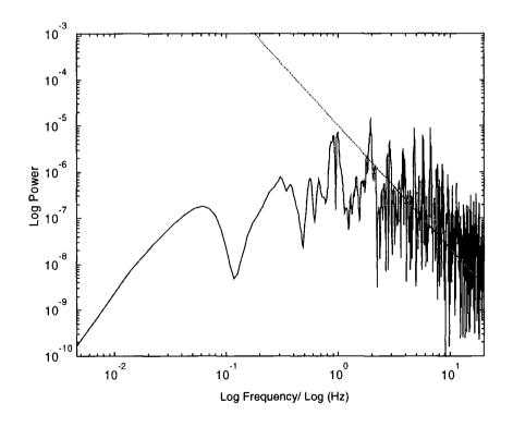
Figure 6.13. The power spectrum of the phase produced by the ATS (solid). The dotted line shows a -8/3 power law.
