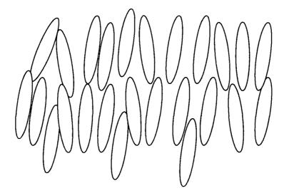
Figure 2.2. A snap shot of the molecules in nematic liquid crystal. On average the molecules point in the same direction.
