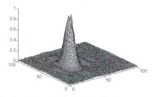
Figure 5.9 (a). The unaberrated PSF. The Strehl ratio is defined as being 100% at the peak intensity.
