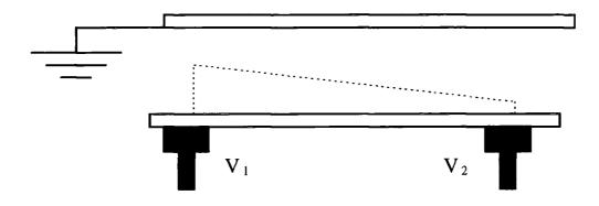
Figure A2.1. The voltage slope across the resistive layer.  $V_1$  and  $V_2$  are applied via discrete electrodes. At the top is earthed ITO glass.
