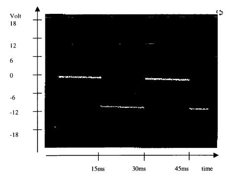
Figure 4.6. The same as figure 4.5 but showing the row voltage only (row 32). The square wave is 0V to -11V. Note that there are no spikes on this plot. Subtracting figure 4.5 gives us figure 4.4.
