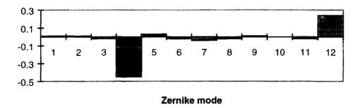
Figure 8.26. The Shack-Hartmann measured power spectrum of mode 12.
