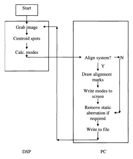
Figure 6.9. The software flowchart of the Shack-Hartmann system.
