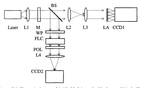
Figure 7.1. The optical set-up. L1, L2, L3, L4 are doublet lenses; M is the Hex69
