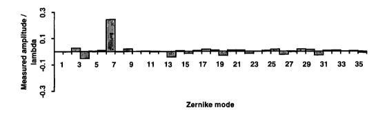
Figure 8.12. The Zernike power spectrum of a coma (mode 7) aberration introduced by the Hex 69 of amplitude  $0.25\lambda$ .
