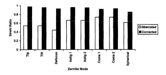
Figure 8.5. The aberrated and corrected Strehl ratios from simulated data. The amplitude of the Zernike modes was  $\mathcal{N}4$
