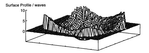
Figure A2.5. A surface profile of the plastic layer measured with the Zygo interferometer.
