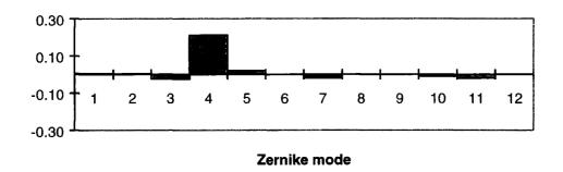
Figure 8.18. The Shack-Hartmann measured power spectrum of mode 4.
