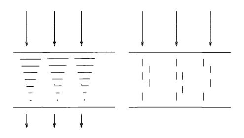
Figure 2.11. A twisted nematic display. Light enters at the top though a polariser. When there is no electric field the molecules rotate the plane of polarisation by 90° and it passes through the second polariser that is orthogonal to the first. When an electric field is applied there is no rotation and hence no transmission of light.
