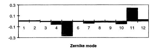
Figure 8.25. The Shack-Hartmann measured power spectrum of mode 11.
