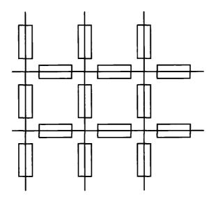
Figure A2.2. An example of the resistive network used as an approximation for the simulation of the resistive layer.
