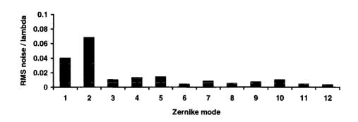
Figure 6.10. The RMS noise limit of each mode.
