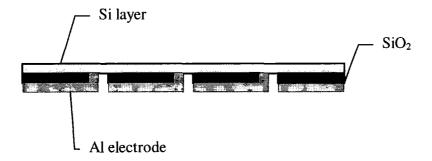
Figure A2.7. Design 2. The liquid crystal material would go on top of the Si layer. The  $SiO_2$  would shield the liquid crystal from the Al electrodes except at the points were pits are etched.
