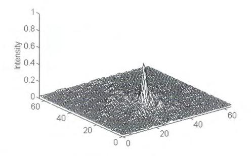
Figure 7.5. The corrected PSF. The Strehl ratio was 48%
