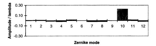
Figure 8.24. The Shack-Hartmann measured power spectrum of mode 10.
