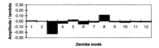
Figure 8.22. The Shack-Hartmann measured power spectrum of mode 8.
