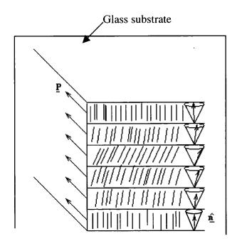
Figure 2.7. The director in Smectic C\* rotates from layer to layer when the liquid crystal is not stabilised by the glass substrate.  $\underline{P}$  is the direction of electric dipole moment.  $\underline{\hat{n}}$  is the direction of the liquid crystals director.
