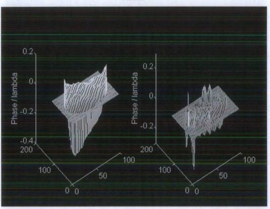
Figure 8.4. The left graph is the uncorrected phase graph. The right graph is the corrected. The sharp peaks on the corrected phase graph are from bad data points measured by the Zygo. Ignoring these points will greatly improve the peak to valley measurement.
