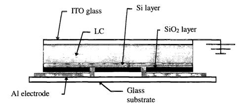
Figure A2.8. Design 3. This design is based on a glass substrate with Aluminium tracks on top of this and either  $SiO_2$  or 'liquid glass' acting as the insulator between the conducting tracks and the resistive Si layer.
