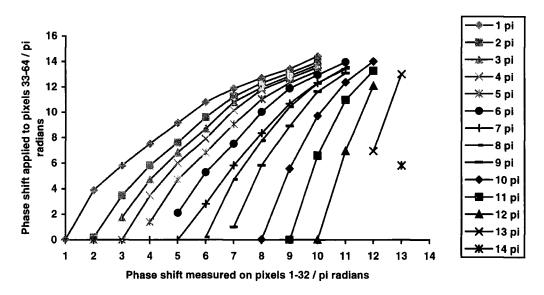
Figure 4.13. The measured phase shift produced in columns 1-32 of the SLM. Columns 1-32 has the expected phase shift applied that is indicated by the legend. The phase shift produced by columns 1-32 is shown (x-axis) as the voltage is varied across columns 33-64 (y-axis).
