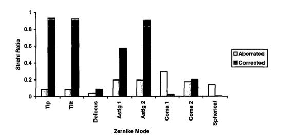
Figure 8.6. The aberrated and corrected Strehl ratios from simulated data. The amplitude of the Zernike modes was  $\lambda/2$ . Defocus, astigmatism 1, coma 1 and 2 and spherical are incorrect because the Zygo could not measure the aberration produced by the Hex69 due to the coarse pixelation so no reliable results were possible for these modes at this amplitude.
