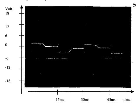
Figure 4.9. CRO trace showing the voltage measured from pixel (32,22). A step function is been applied to the SLM. Columns 1-32 are fully on and columns 33-64 are off. The waveform goes from +2V to -0.1V to -2.2V to -0.2V. The spikes are +15V and -15V.
