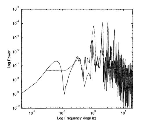
Figure 6.14. The power spectrum of the measured mode 3 (solid line) and the power spectrum of the initial data (dotted line) showing that the Hex69 accurately represents the phase data generated by the Glindemann software.
