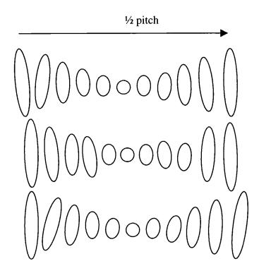
Figure 2.3. A snap shot of the molecules in cholesteric or chiral nematic. The directors are rotated by some angle from one molecule to the next. The distance it takes for a 360° rotation is known as the pitch.
