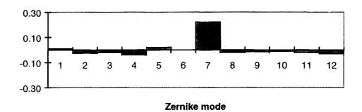
Figure 8.21. The Shack-Hartmann measured power spectrum of mode 7.
