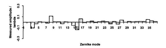
Figure 8.13. The Zernike power spectrum of a mode 8 spherical aberration introduced by the Hex 69 of amplitude  $0.25\lambda$ . There is some crosstalk into defocus, higher order spherical (mode 15) as well as other modes.
