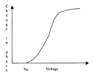
Figure 2.6. A typical voltage response curve of nematic liquid crystal. V<sub>th</sub> is the threshold voltage. The exact units will depend upon the liquid crystal material and the cell thickness.
