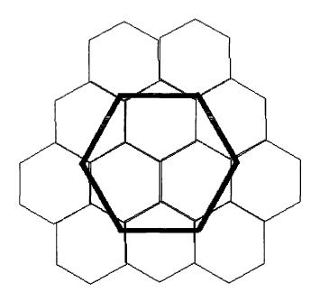
Figure 6.3. The approximate sampling of the Hex69 pixels (thin lines) by a Shack-Hartmann lenslet (dark line).
