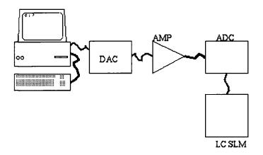
Figure 4.1. The 64x64 SLM's drive electronics block diagram.
