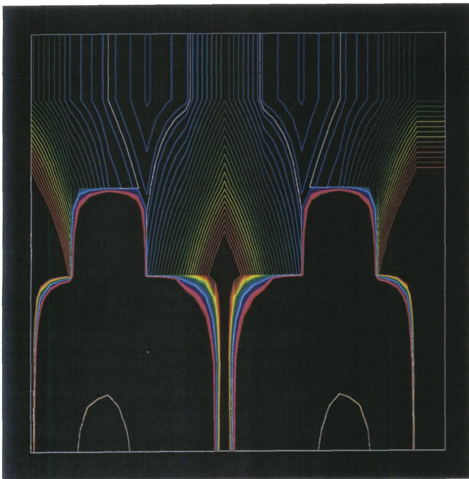
Figure 5.13: Contour plot perpendicular to surface through section O-O in figures 5.10 - 5.12. The white contour marks zero energy relative to CO at infinite distance
