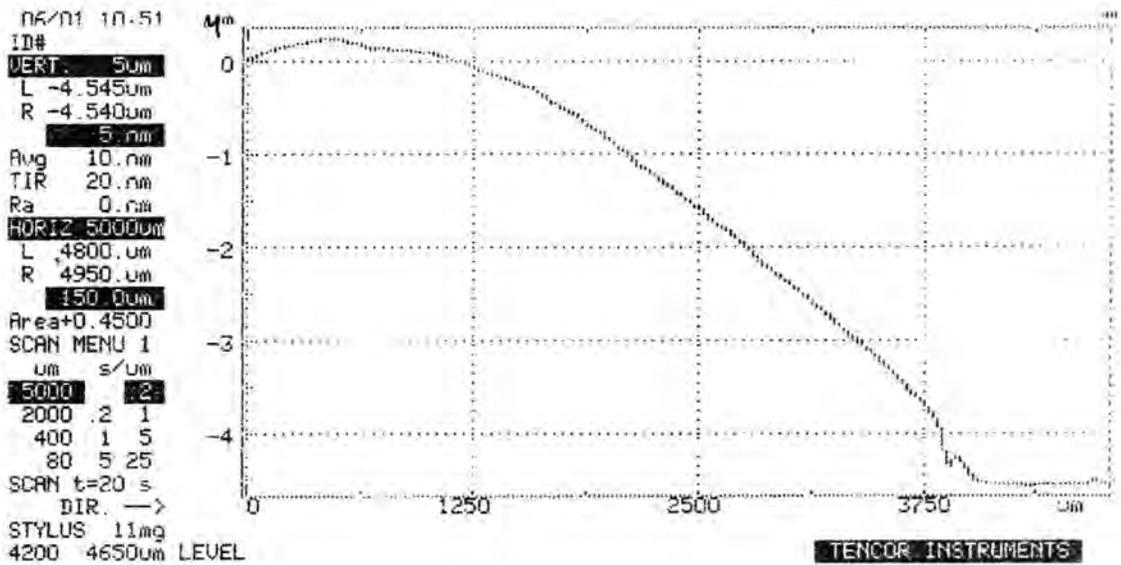
Figure 59: Alpha step scan for CdCl<sub>2</sub> sample
