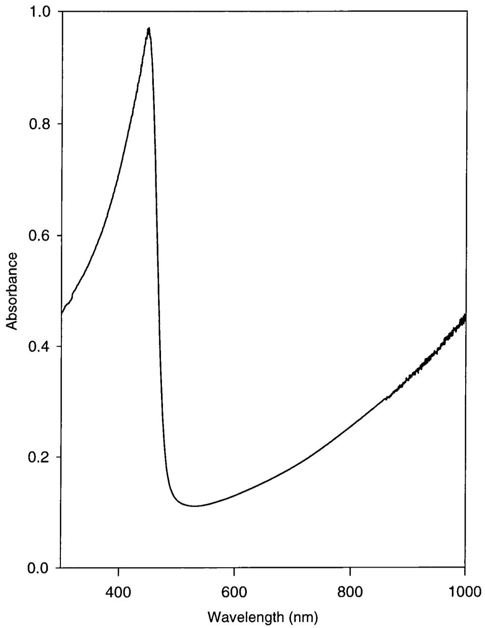
**Figure 39: Absorption spectrum of a 0.1µm PANi film on glass**
