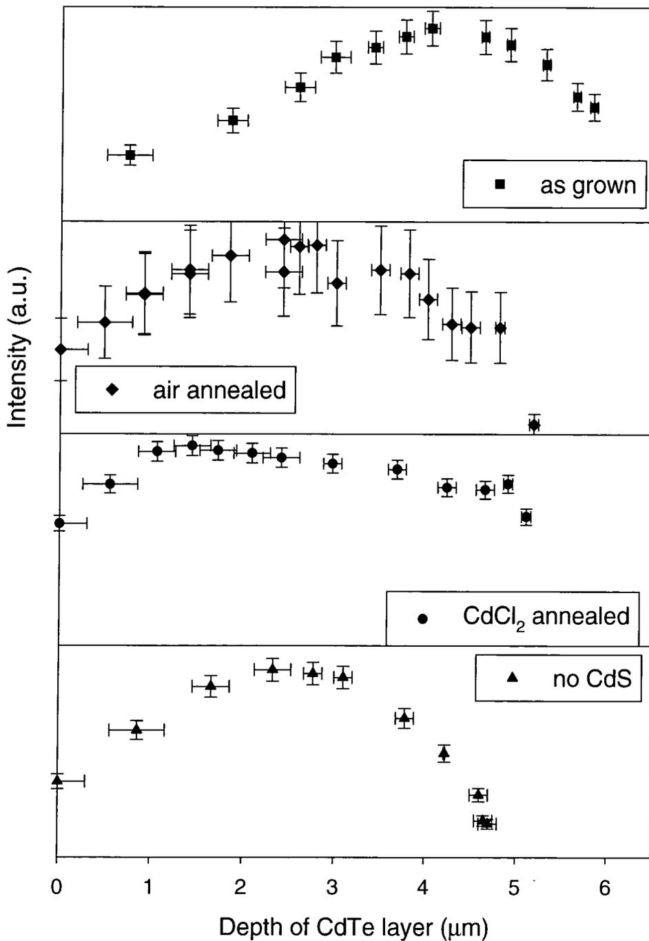
**Figure 67: Comparison of 1.45 eV photoluminescence emission band**
