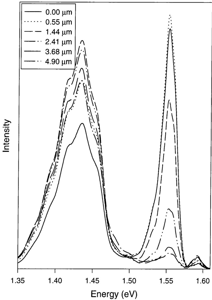
**Figure 60: Photoluminescence spectra from different depths of the CdTe layer of a CdCl<sub>2</sub> treated CdS/CdTe solar cell**
