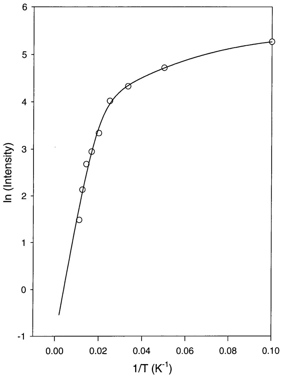
**Figure 56: Temperature dependence of excitonic emission from CdCl<sub>2</sub> treated sample**
