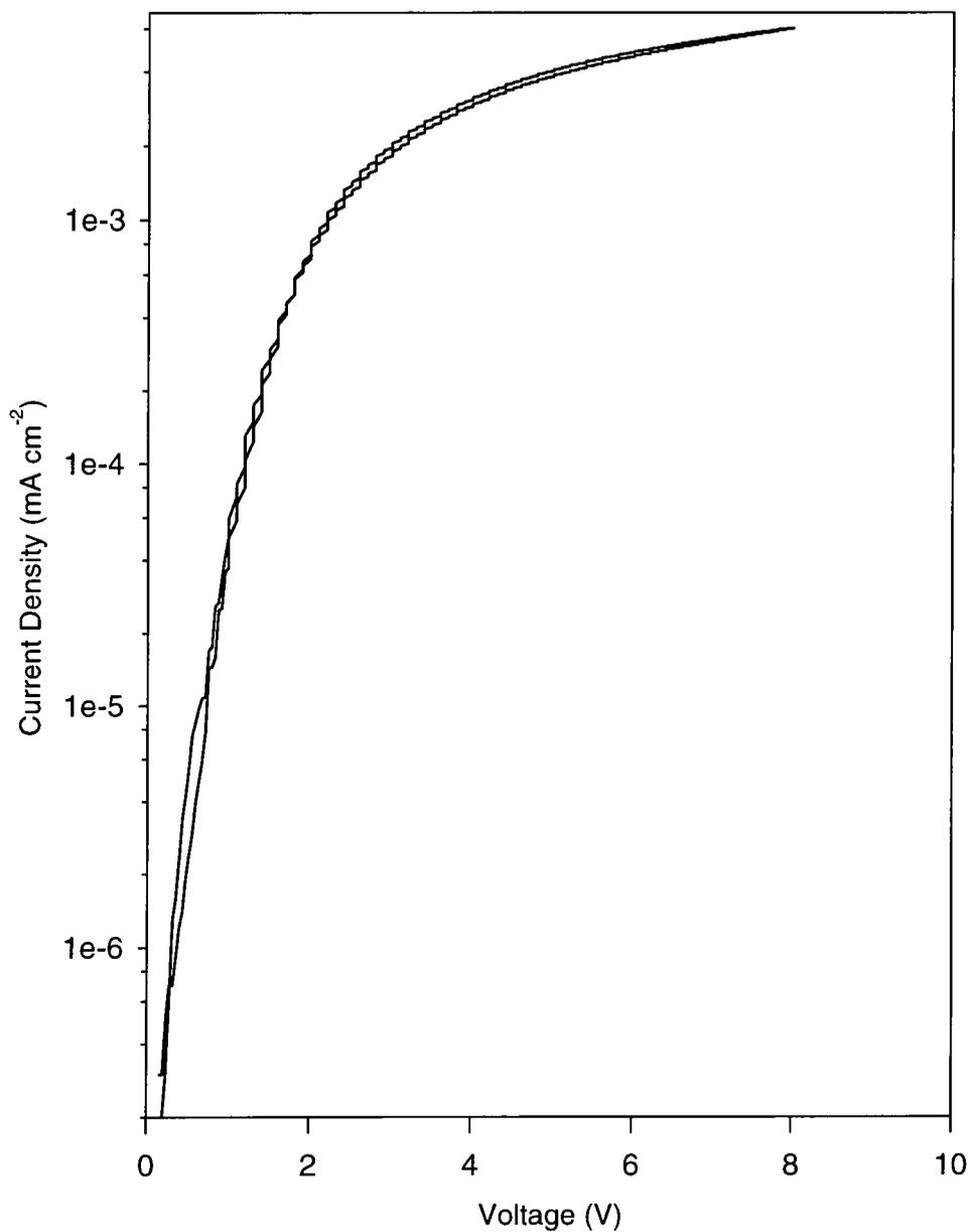
**Figure 43: I-V characteristics of porous silicon-polyaniline device using a log scale**
