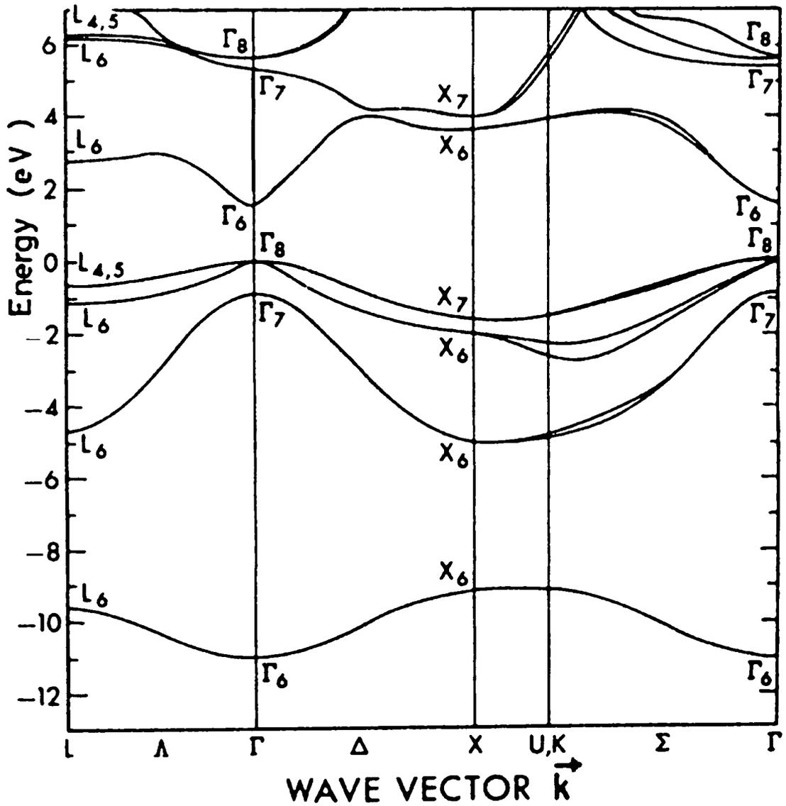
Figure 11:  $E$ - $k$  bandstructure diagram for cadmium telluride<sup>[9]</sup>
