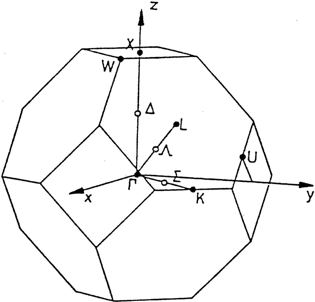
**Figure 3: Locations of points in reciprocal space used in band structure diagrams**
