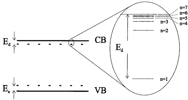
**Figure 16: Diagram of donor and acceptor energies**
