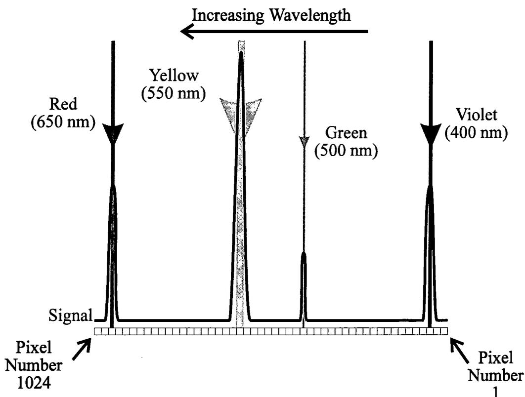
**Figure 23: Spectral dispersion across the diode array**
