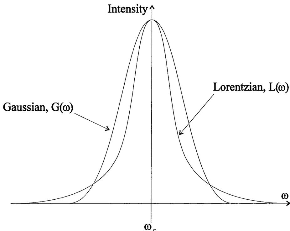
**Figure 19: Comparison of Lorentzian and Gaussian line shapes**
