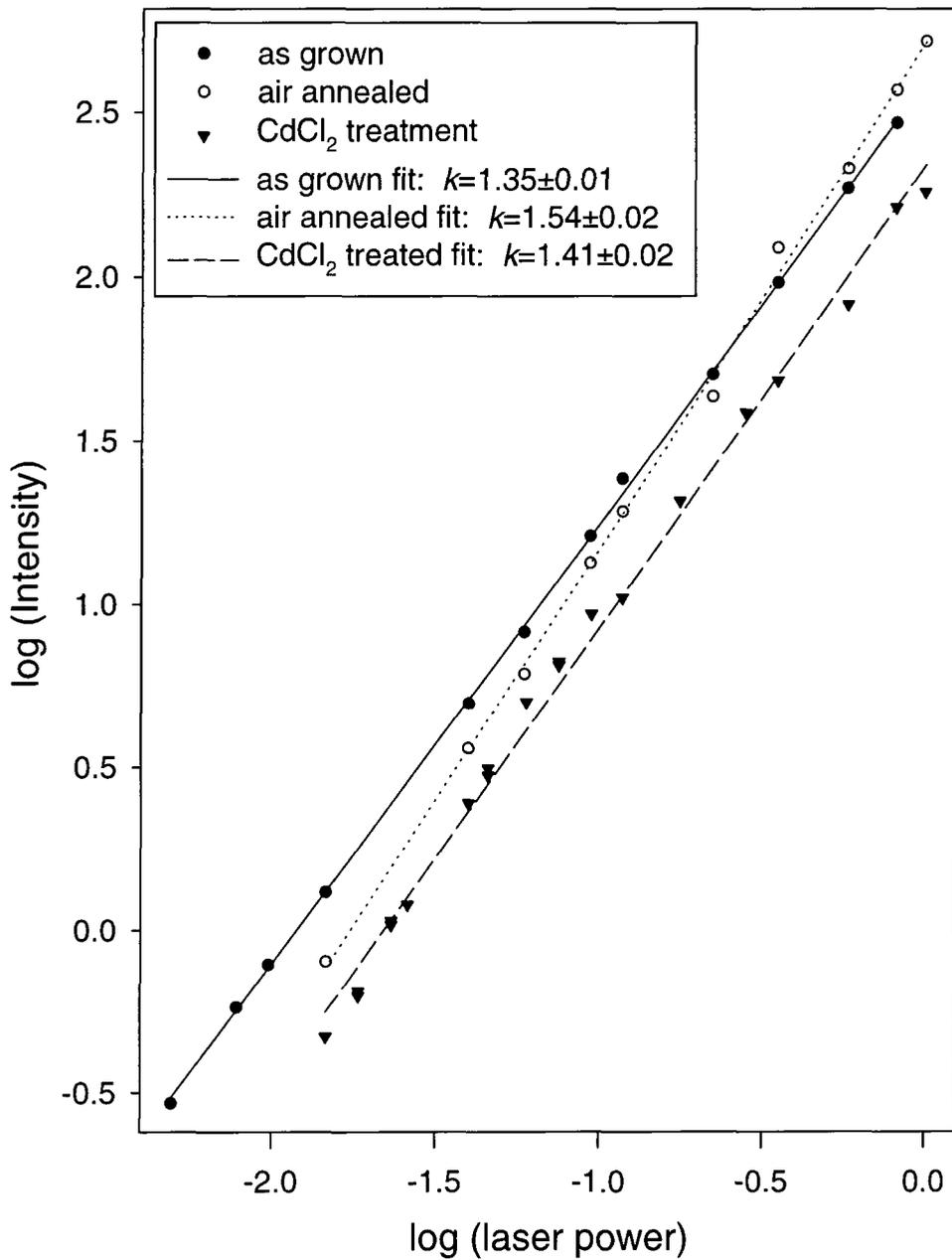
Figure 52: Power dependence of 1.59 eV emissions from samples
