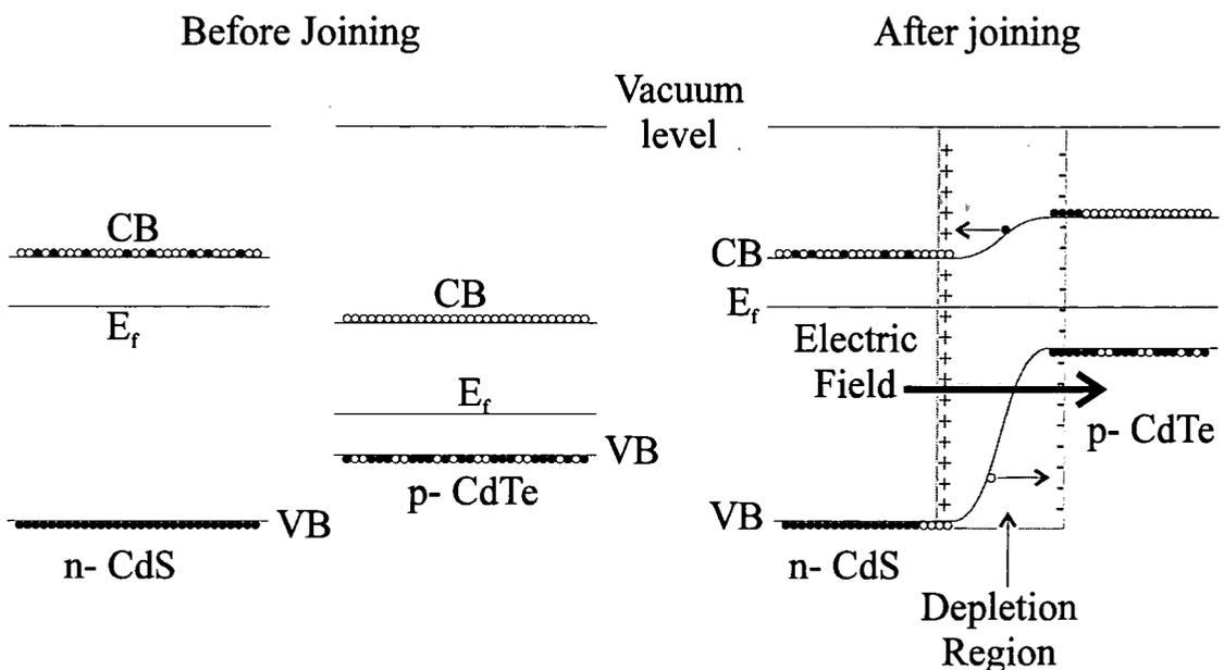
**Figure 46: Creation of in built electric field**
