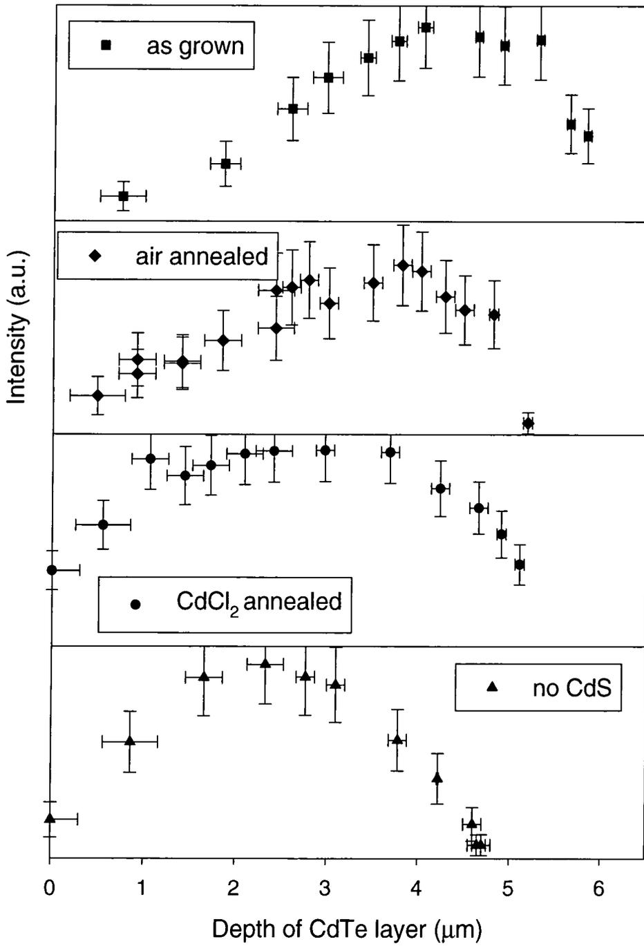
**Figure 65: Comparison of 1.59 eV photoluminescence emission band**
