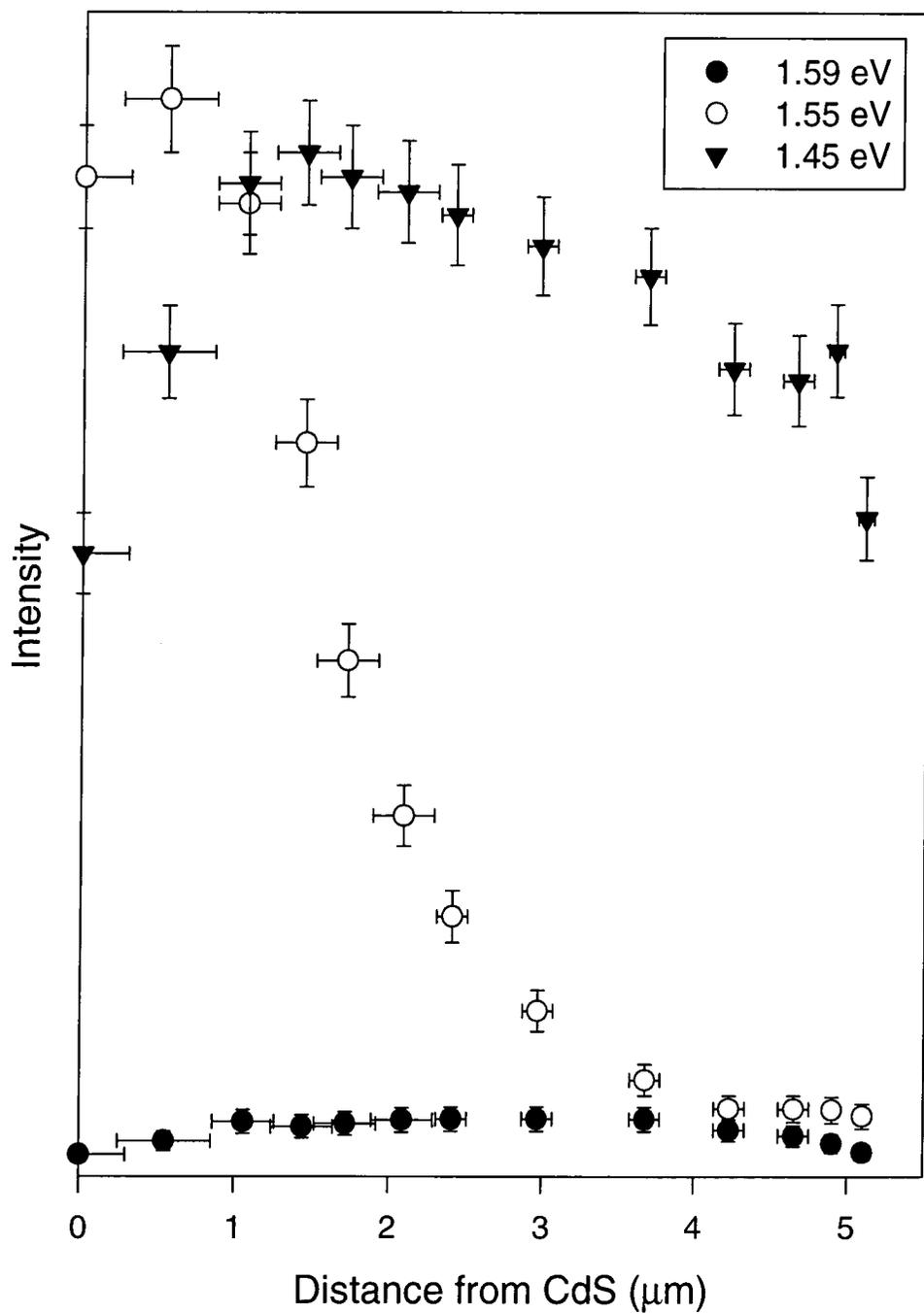
**Figure 63: Depth dependence of photoluminescence intensity for CdCl<sub>2</sub> annealed sample**
