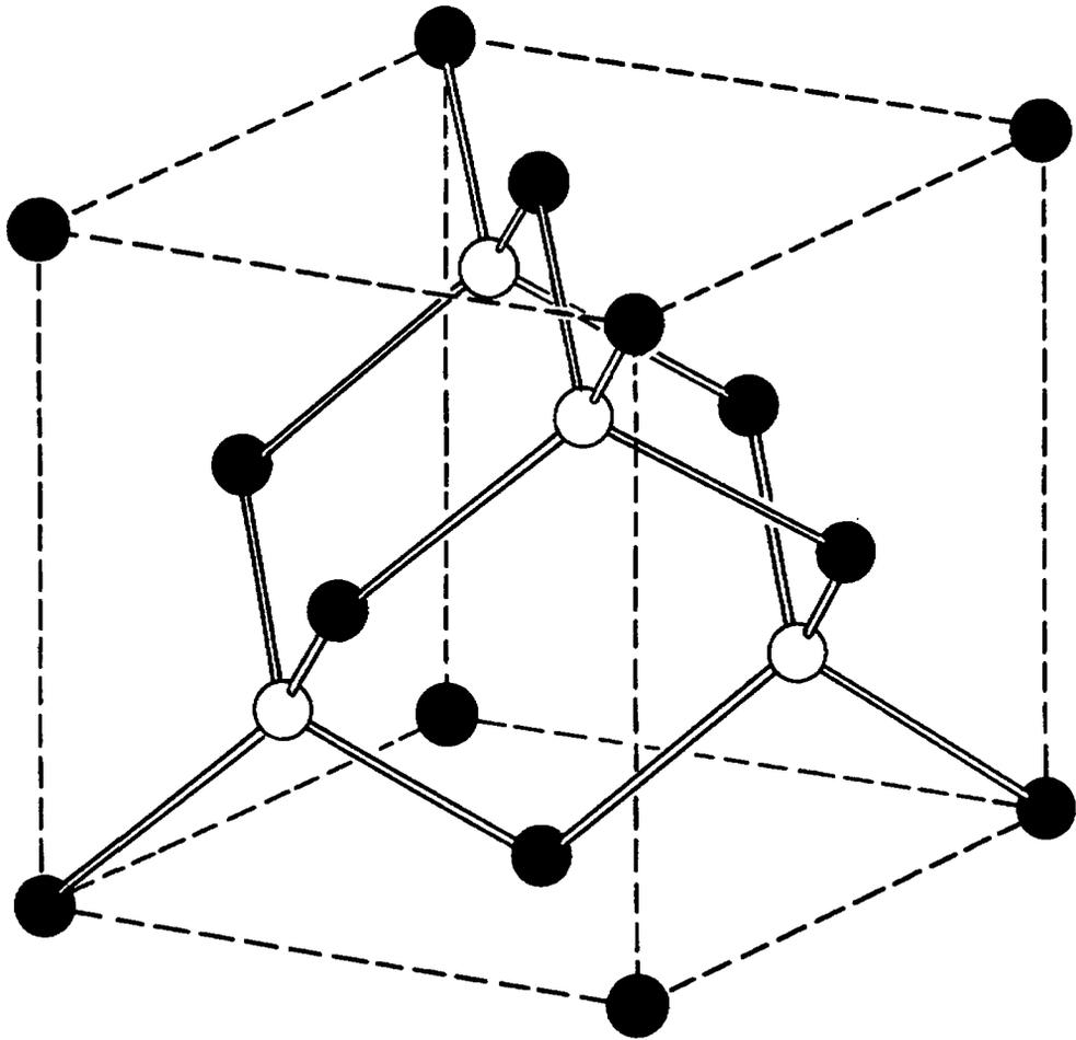
**Figure 1: Zinc blende, or face centred cubic, structure**
