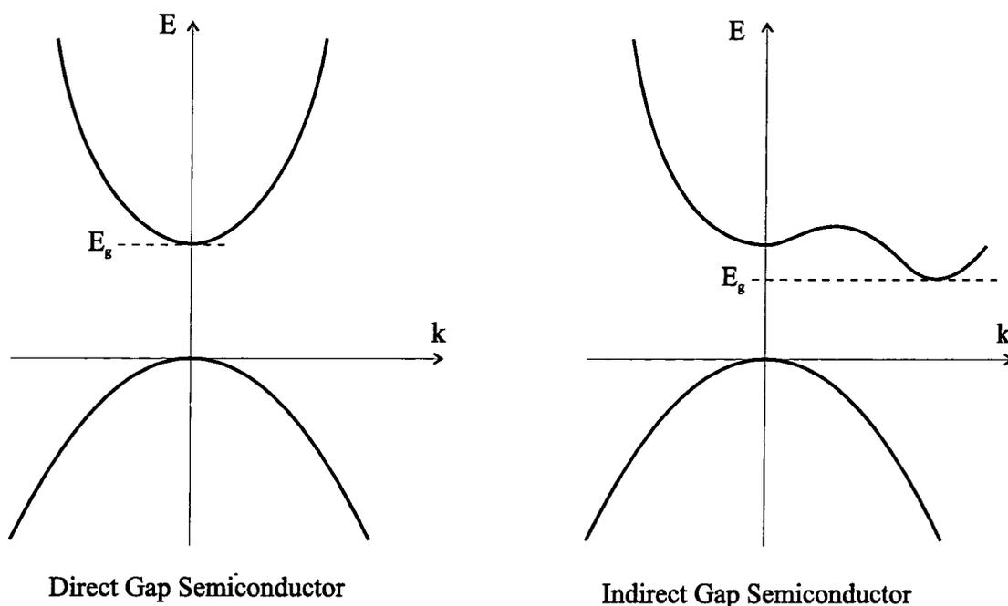
**Figure 13: Direct and indirect energy gaps**
