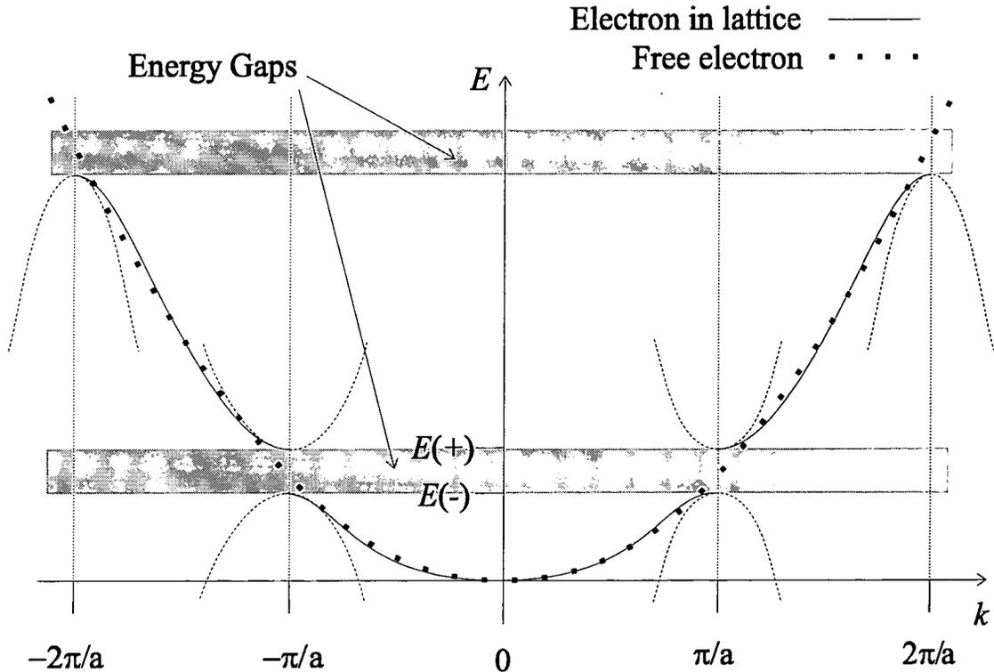
**Figure 5: Electronic band structure for the Nearly Free Electron Model**
