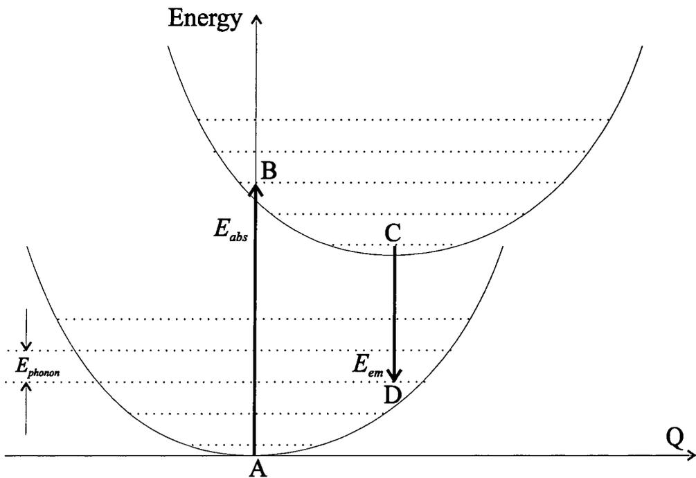
**Figure 21: Configuration co-ordinate diagram for Franck - Condon approximation**
