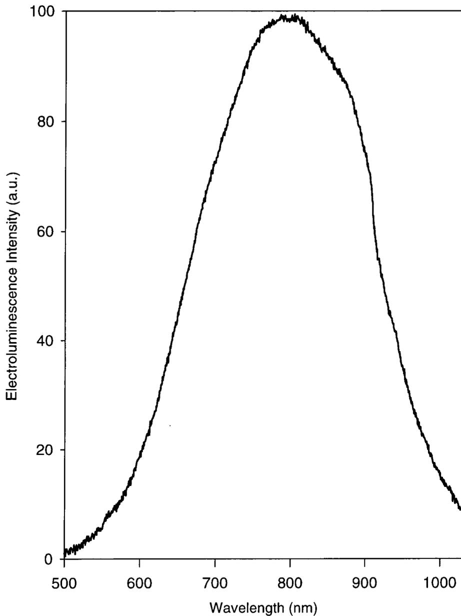
**Figure 44: Electroluminescence spectrum measured from a PS-PANi junction
