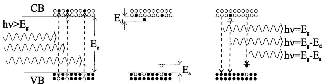
**Figure 18: Some photoluminescence process in a semiconductor**
