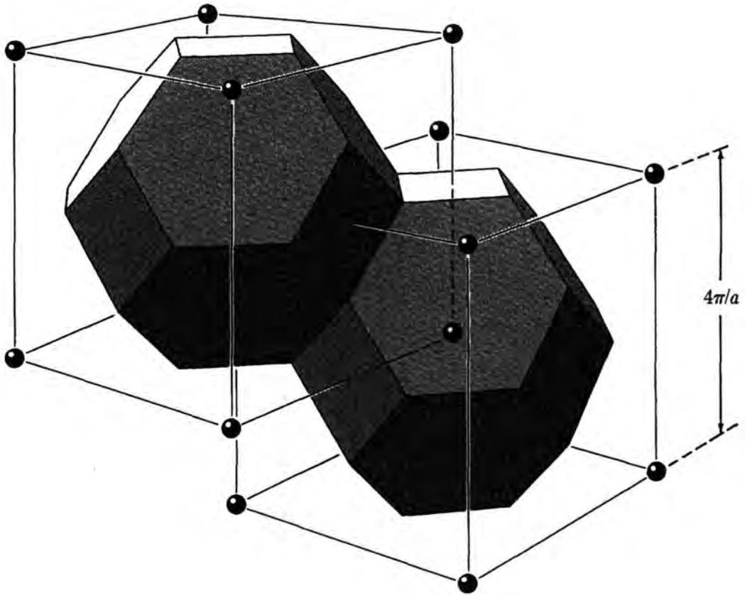
**Figure 2: The 1st Brillouin Zone for a zinc blende semiconductor (having a body centred cubic reciprocal lattice)<sup>[3]</sup>**
