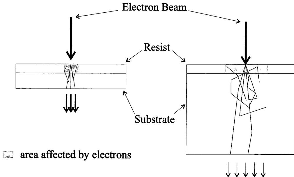
**Figure 24: Effect of back-scattered electrons in lowering resolution**
