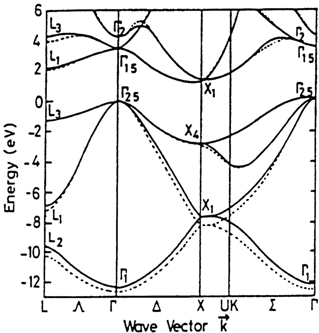
Figure 9:  $E-k$  Bandstructure diagram for silicon<sup>[7]</sup>
