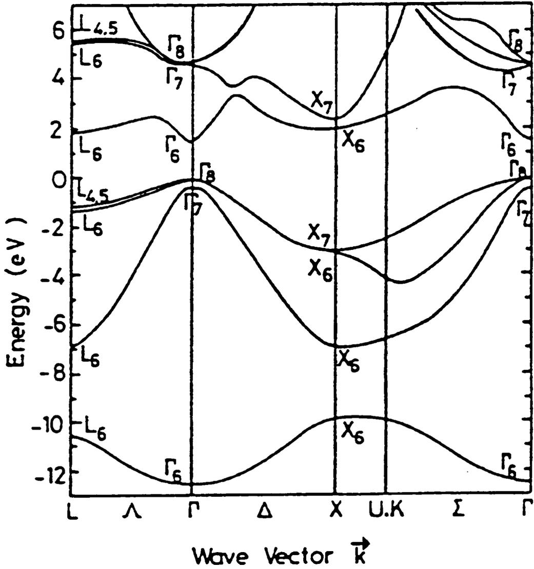
Figure 10:  $E-k$  Bandstructure diagram for gallium arsenide<sup>[8]</sup>
