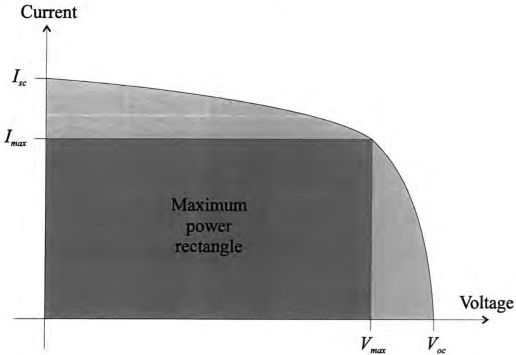
**Figure 48: Cell power performance and output values**
