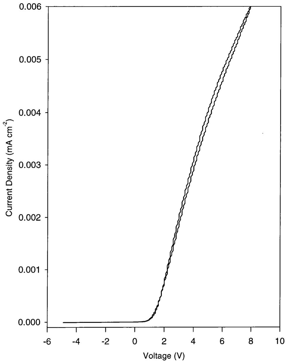
**Figure 42: I-V characteristics of a porous silicon-polyaniline device**
