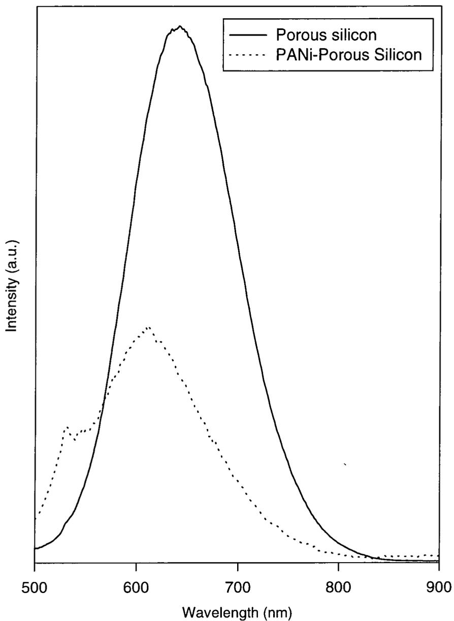
**Figure 38: Photoluminescence spectrum of porous silicon**
