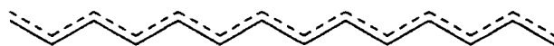
Figure 1.4. A schematic representation of the way in which the \pi orbital of PA was expected to average for long chain PA. The dotted lines represent a "half" \pi bond.
