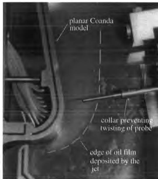
Figure 4.25 : Photograph of the planar model, demonstrating the oil contamination
