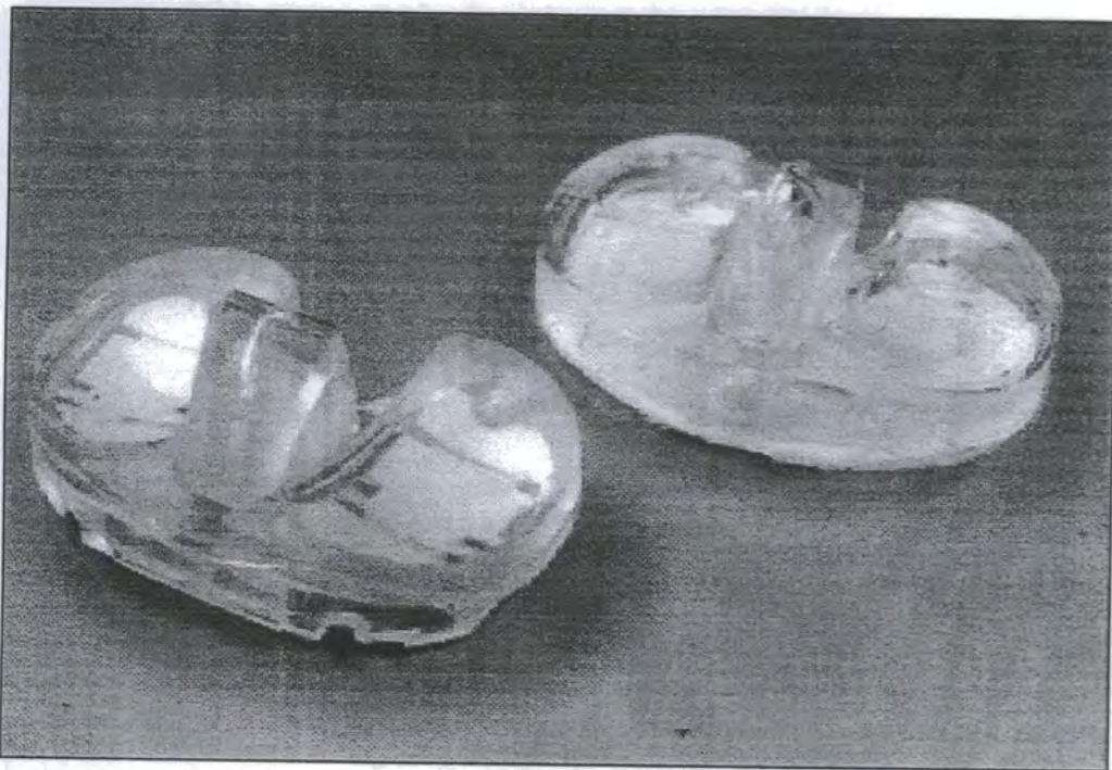
Figure 3.5 Pre-prototype acrylic / PU tibial compliant bearings.
