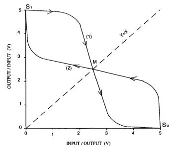
Figure 6.1 Bistable State transfer Curve
