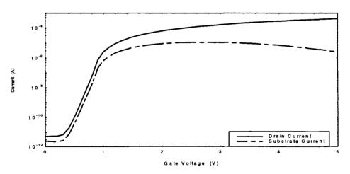
Figure 3.2 Drain current and substrate current versus gate voltage for an nMOS transistor (W=1  $\mu$ m, L=0.8  $\mu$ m, V<sub>DS</sub> = 5 V, Process: EC/3 (see appendix D))
