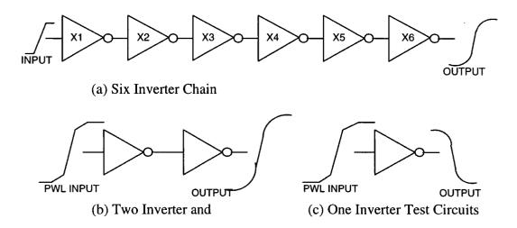
Figure 4.6 Input conditioning test circuits and the wave forms used for simulations
