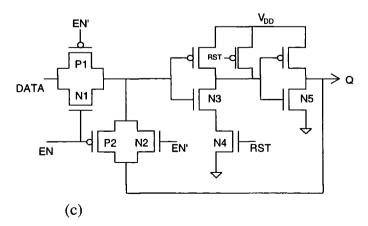
Figure 5.2 Transistor level circuits for the three bistable circuits
