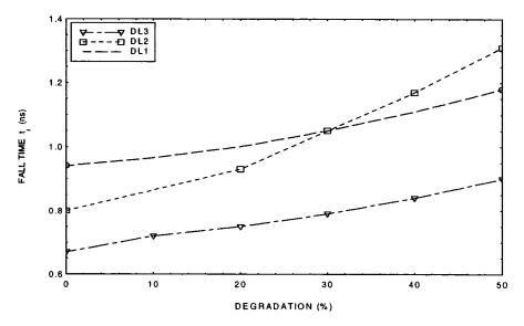
Figure 5.10 Fall Time as a function of Degradation for the three latch circuits (Process: EC/3, Device: 1/0.8)
