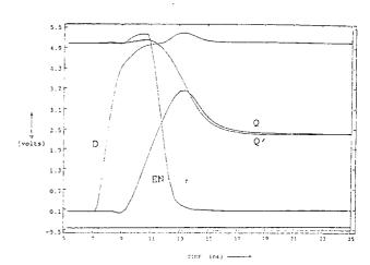
Fig 10. Metastability simulation for NAND-N3
