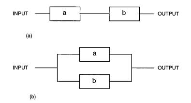
Figure 2.1 (a) Series and (b) parallel models for reliability evaluation
