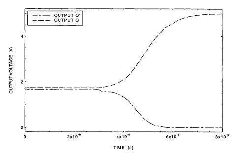
**Figure 6.9 Metastable state resolving simulation for DL1**. (Process: EC/3, Device: 1/0.8)
