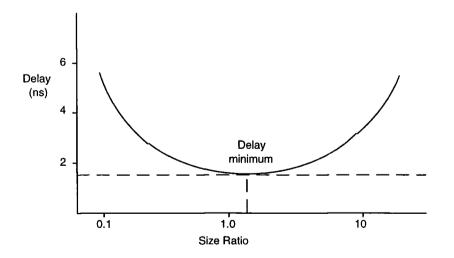
Figure 4.2 Delay of a CMOS inverter versus size ratio of p- and n- devices
