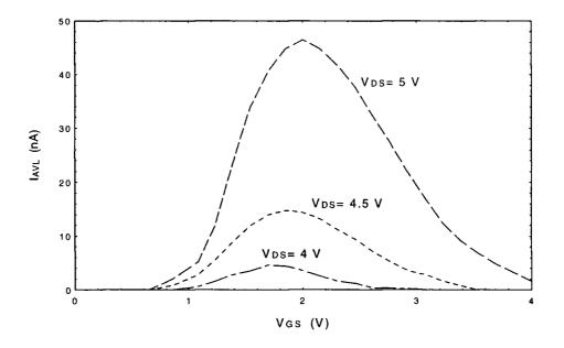
**Figure 3.5 Substrate currents plotted using Philips model** (Device: N 1/0.8, Process: EC/3)
