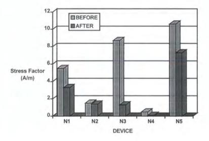
Figure 7.7 Stress factors for DL3 before and after design changes (Technology: EC/3, Device size has been adjusted to reduce stress)
