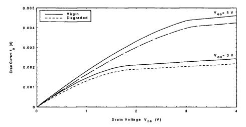
Figure 3.13 Characterisation of degradation effects:  $I_D$  vs  $V_{DS}$  plotted for a virgin device and for a device with SPICE parameters degraded by 10% (Device: N:10/0.55, Process: EC/3) Lunenborg [3.41].
