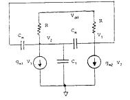
Fig 4. Small signal model of the latc
