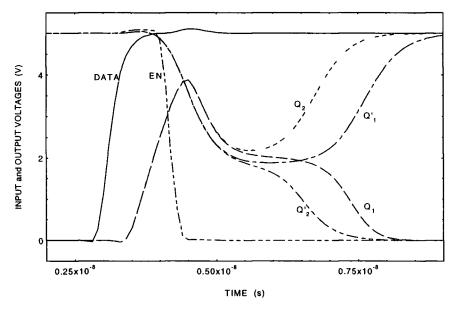
Figure 6.6 Metastability resolving for latch DL2 at clock edge of 0.92329685 ns  $(Q_1 \& Q_1')$  and 0.92329688 ns  $(Q_2 \text{ and } Q_2')$ . (Process: EC/3, Device: 1/0.8)
