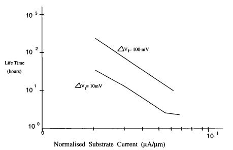
Figure 3.9 Lifetime vs normalised substrate current: HOTRON model
