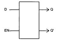
Figure 4.0 D-latch logic symbol
