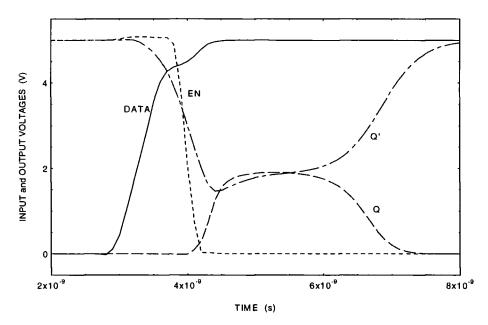
Figure 6.7 Metastabilty simulation for latch DL3 at a clock edge of 0.7139798 ns. (Process: EC/3, Device: 1/0.8)
