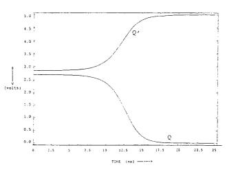
Fig 12. Metastability resolving for MX-GATE
