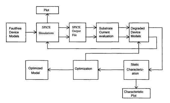
Figure 3.6 Optimisation steps: Substrate current model
