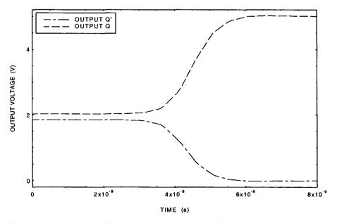
Figure 6.10 Metastable state resolving for DL2. (Process: EC/3, Device: 1/0.8)
