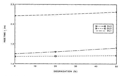
Figure 5.10 Rise Time as a function of Degradation for the three latch circuits (Process EC/3, Device 1/0.8)
