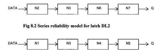
Fig 8.3 Series reliability model for latch DL3
