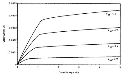
(b) Output curves in Level 2: Short channel effects (Process: EM/3, Device: N 2/4)
