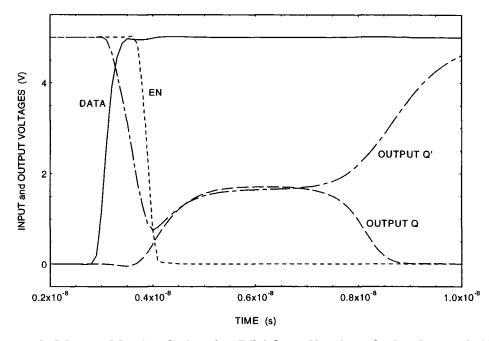
Figure 6.5 Metastable simulation for DL1 by adjusting clock edge to 0.61035 ns (Process: EC/3, Device: 1/0.8)
