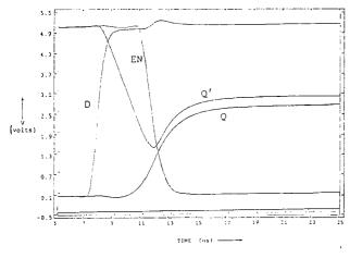
Fig 11. Metastability simulation for MX-GATE
