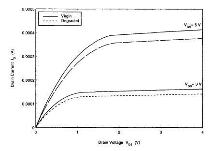
Figure 3.14 Degradation characterisation under normalised conditions: SPICE parameters degraded by 10% (Device N:1/0.8, Process EC/3)
