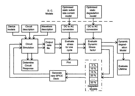
Fig 5.3 Hot-carrier degradation simulation cycle for bistable circuits
