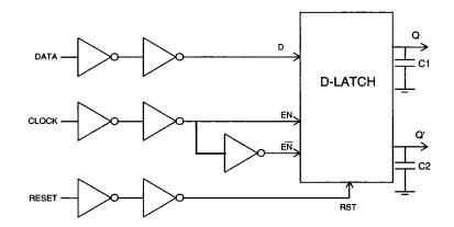
Figure 4.7 Simulation environment for the Latch
