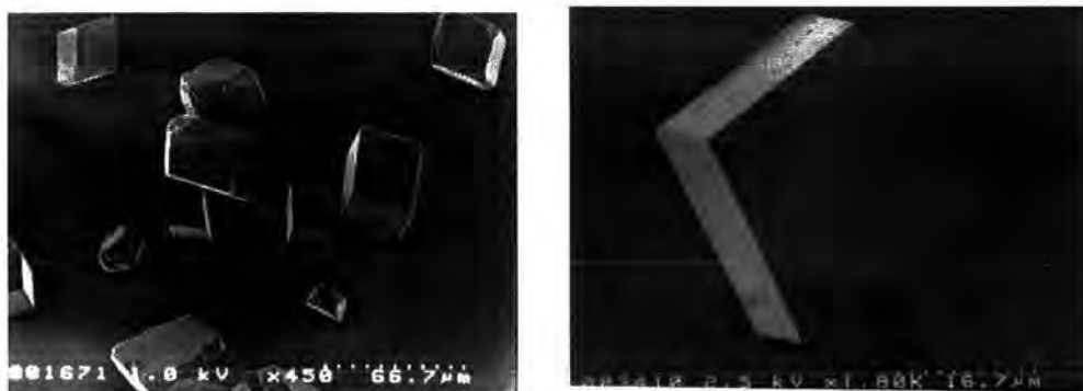
Fig. 3.3.1. Scanning electron micrographs showing control rhombs grown from bulk solution.
