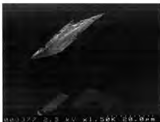
Fig. 5.3.4. Scanning electron micrographs showing \text{CaCO}_3 crystals grown at the air,polymer/water interface with Poly3F [\text{Ca}^{2+}]:[\text{repeat unit}] 10:1.
