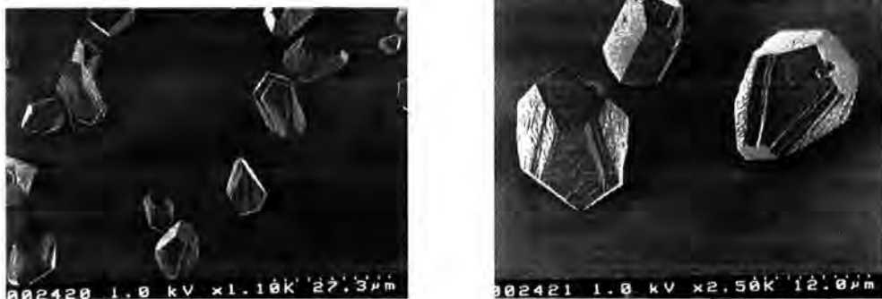
Fig. 3.3.17. Scanning electron micrographs showing \text{CaCO}_3 crystals grown from bulk solution in presence of model compound 4c [\text{Ca}^{2+}]:[\text{model compound 4c}] 100:1.
