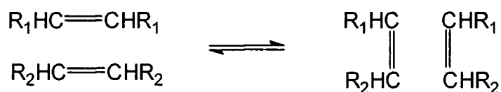
Fig. 1.3.1. The olefin disproportionation reaction.
