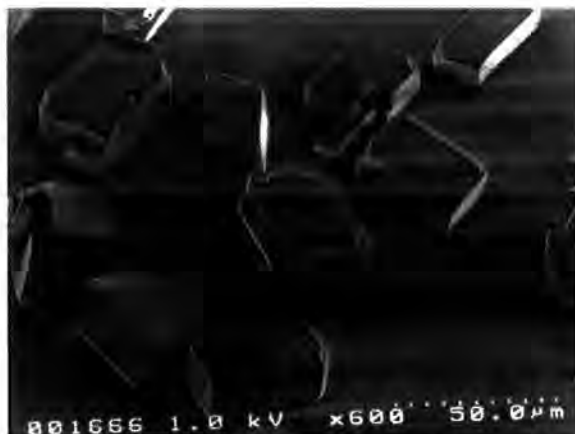
Fig. 3.3.3. Scanning electron micrographs showing \text{CaCO}_3 crystals grown from bulk solution in presence of model compound 5. a. [\text{Ca}^{2+}]:[\text{model compound 5}] 10:1.
