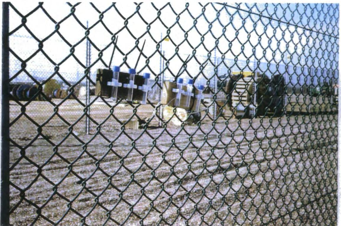
**Plate 6. NO<sub>2</sub> passive diffusion tube samplers at the CATS Terminal, adjacent to the constructed reedbed.**
