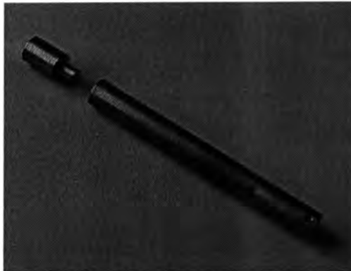
Figure 6.9. DAFI lens and fibre mount.
