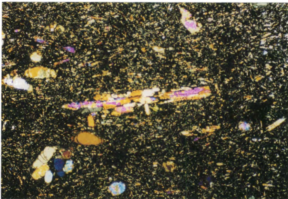
Plate 4.21. Prismatic crystals of clinopyroxene set in a fine-grained groundmass. 1.3x0.77mm, XP
