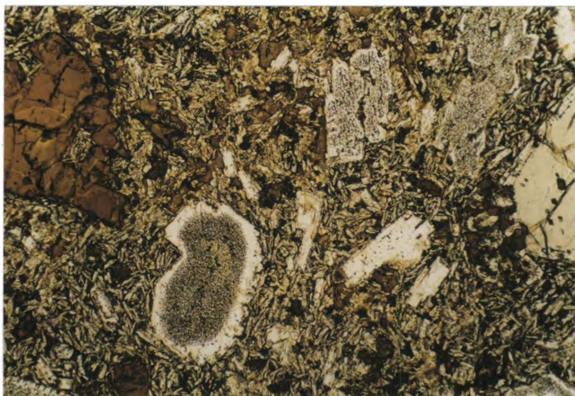
Plate 4.15. Resorbed plagioclase and altered olivine phenocrysts set in a microcrystalline groundmass. Olivines are altered to iddingsite. 3x1.9mm, XP and PPL
