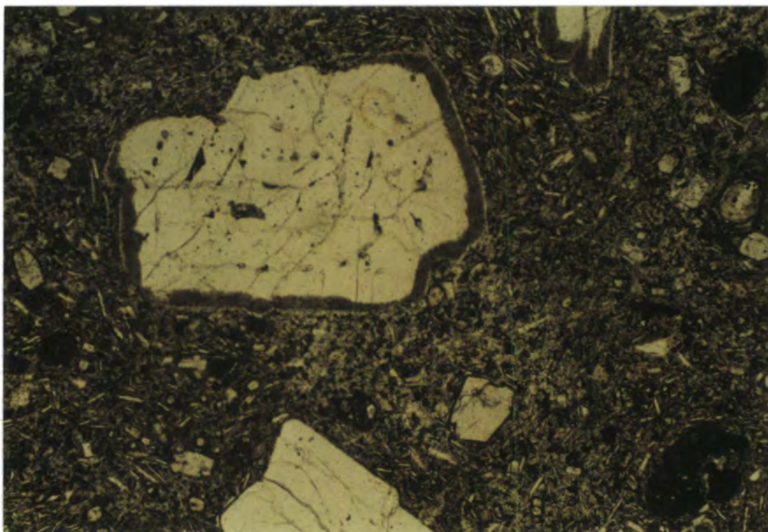
Plate 4.1. Large, intermediate plagioclase set in a partially crystalline groundmass. The plagioclase is surrounded by a dark, dusty reaction rim. Field of view 3x1.9mm, shown in plane polarized light (PPL).
