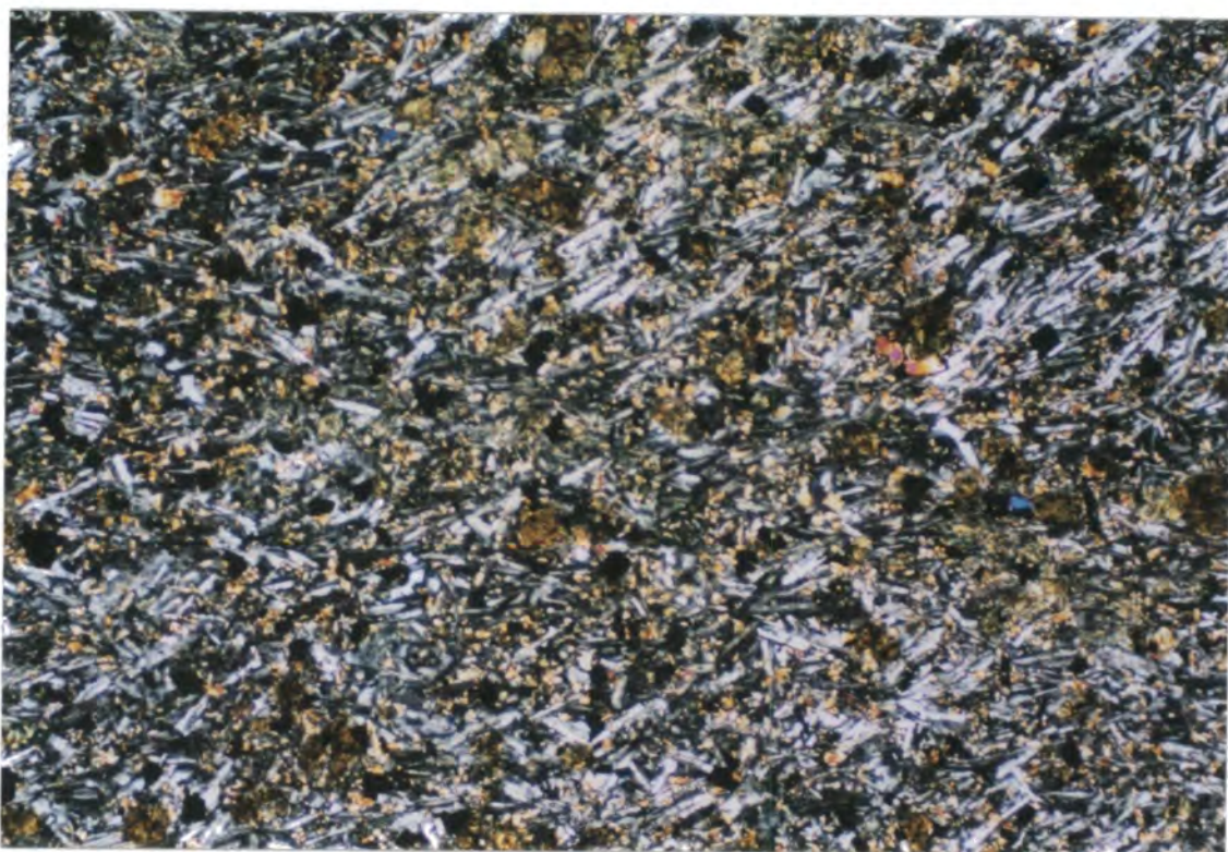
Plate 4.18. Felty textured aphyric alkaline basalt. Plagioclase microlites characteristically show parallel alignment. 3x1.9mm, XP
