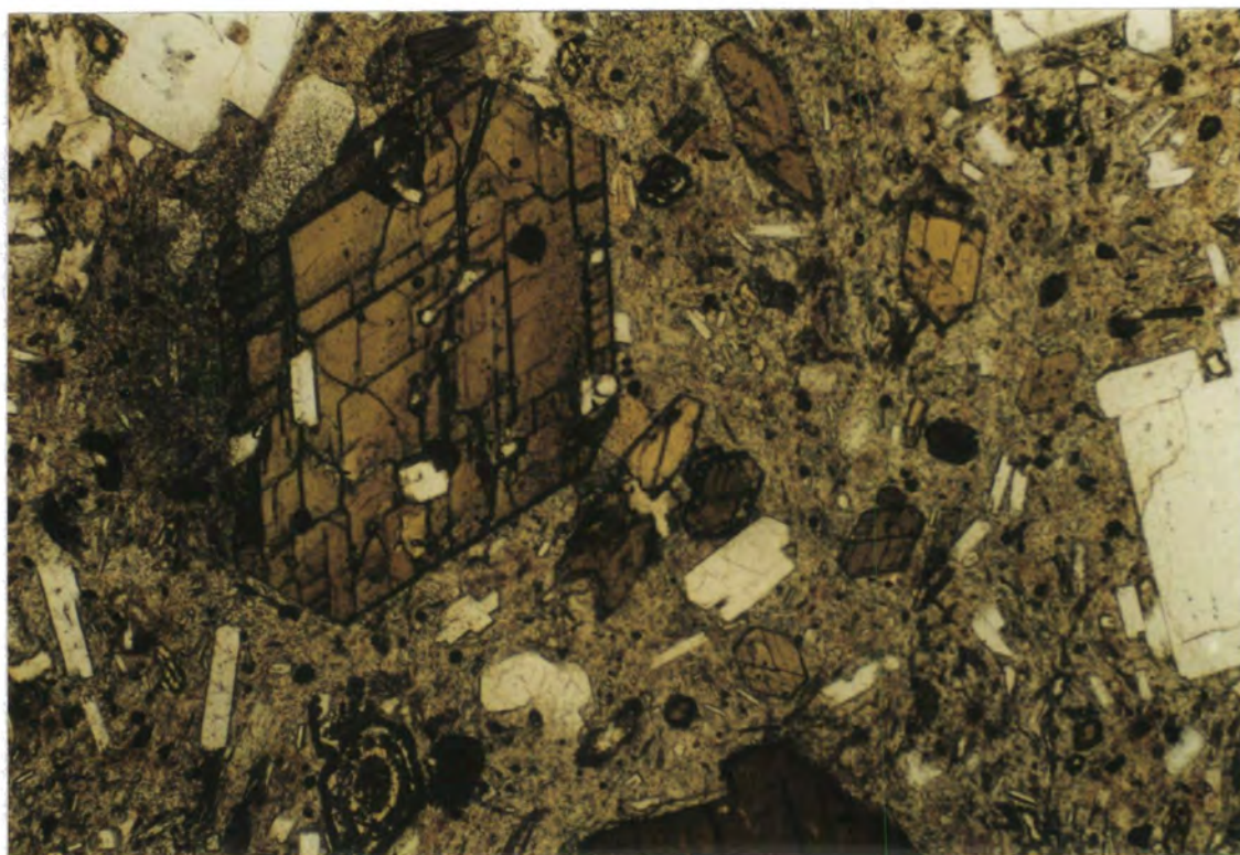
Plate 4.24. Euhedral amphibole phenocrysts set in a mostly glassy groundmass. 3x1.9mm, PPL
