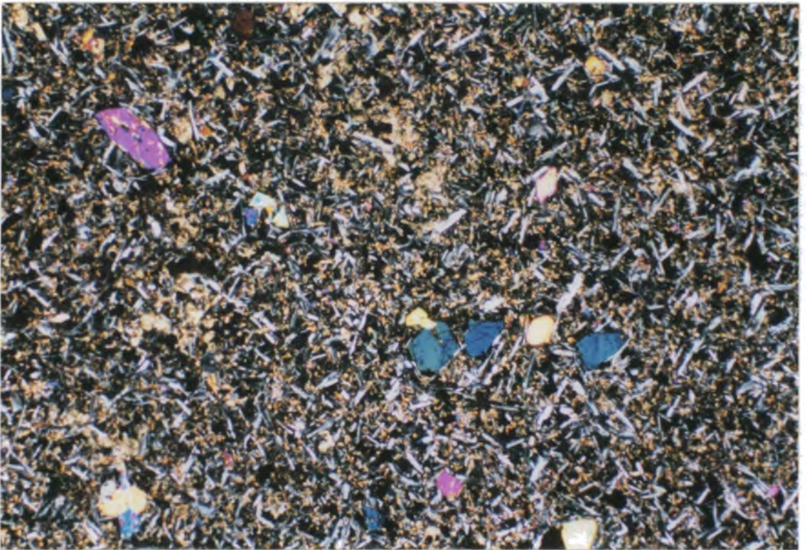
Plate 4.19. Olivine microphenocrysts set in an intergranular groundmass that consists of plagioclase laths and interstitial clinopyroxenes. 3x1.9mm, XP
