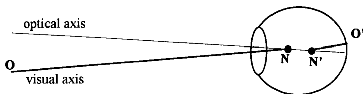
Figure 2.1 Diagrammatic representation of the eye's visual axis and its nodal points (N & N')
