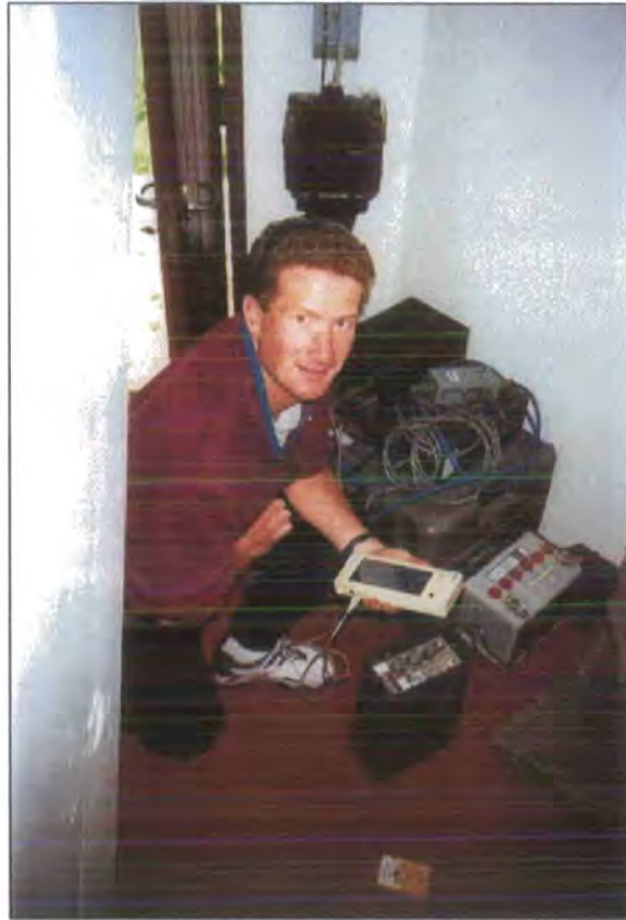
Figure 3.8 Epson EHT being used to load parameters into the DAS (upper left grey unit) at station HOT08 (Ólafsvíti). Also visible is the connected field disk and breakout box (next to DAS), battery and spare field disk on floor. The Seismometer is beneath the insulation on the right.
