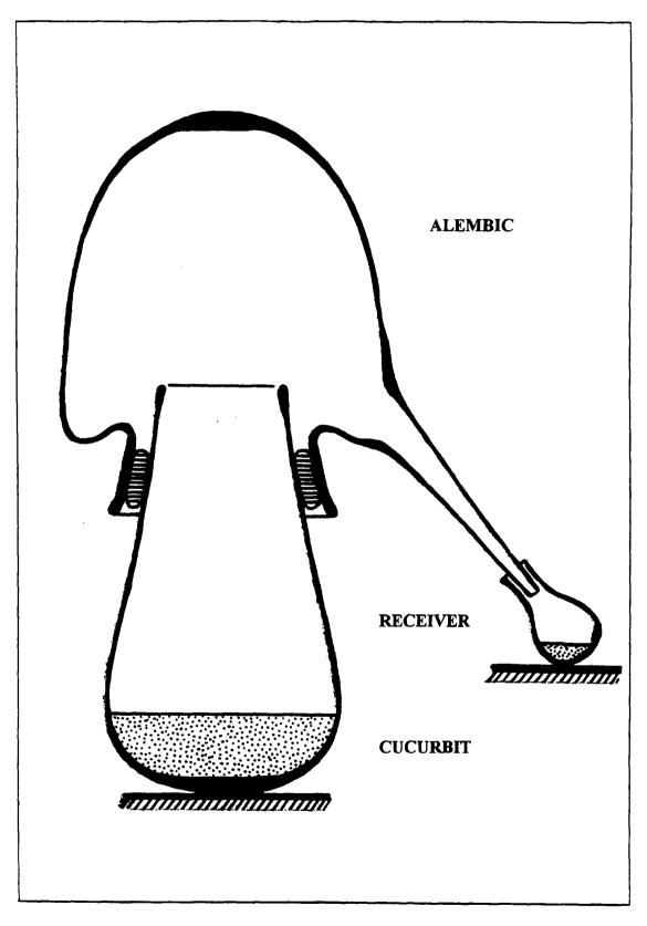
Reconstruction of a medieval distilling set or still comprising a cucurbit, alembic and receiver
