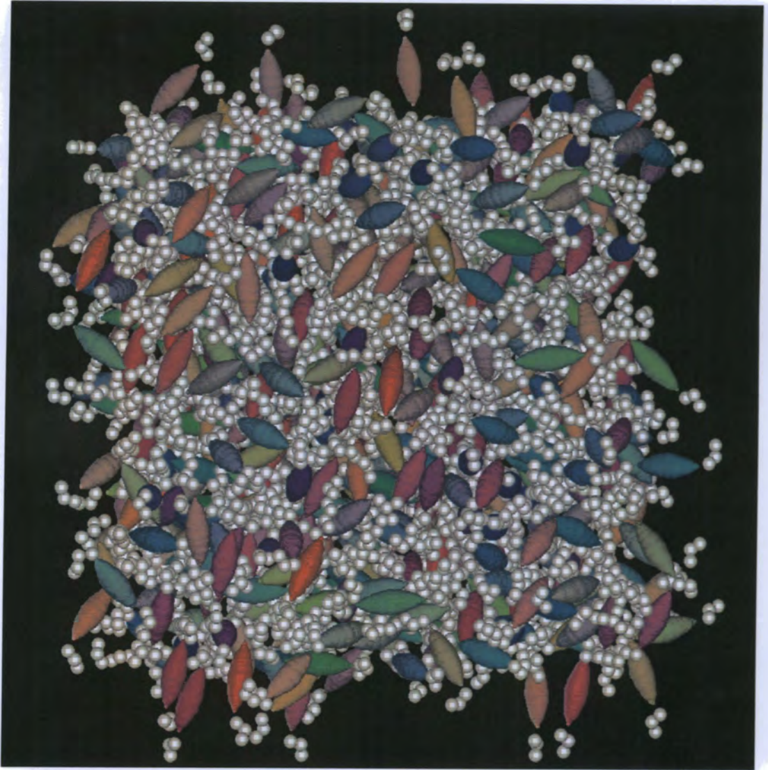
Figure 4.4: System snapshot: isotropic configuration at 500 K ( 752.092 \text{ kg m}^{-3} ). Gay-Berne sites are represented by coloured ellipsoids; Lennard-Jones sites are represented by white spheres.
