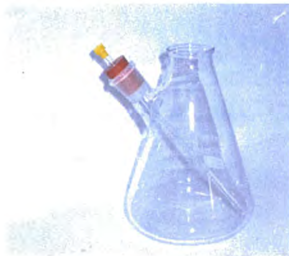
Fig. 2.6 Modified conical flask used to centrifuge the liquid crystalline material within the NMR tube
